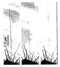
Fig. 1.7 SEM Image of a CNT with two ends attached to two AFM tips before tensile loading [29].
