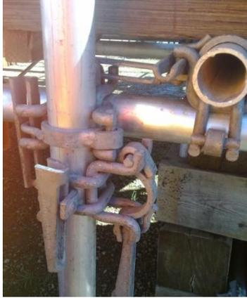
**Figure 2-2 Tube and clamp connections, PCL Modular Yard, Nisku, Edmonton**
