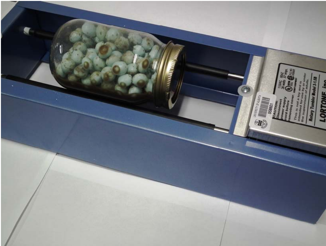
Figure 3.5: Modified rotating mixer used in bitumen removal.
