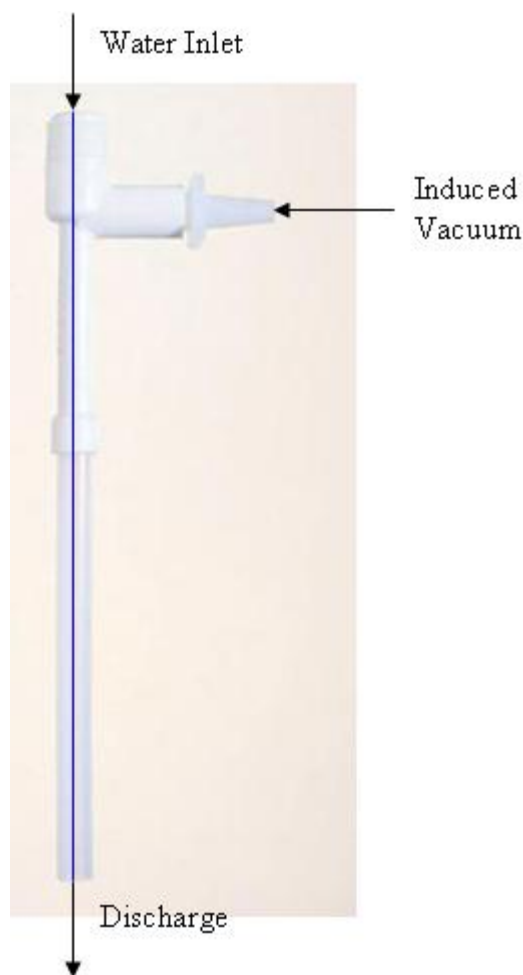
Figure 3.6: Faucet aspirator vacuum pump illustration.
