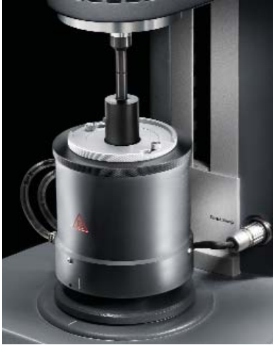
Figure 3.9: AR-G2 concentric cylinder geometry (from TA Instruments, 2006).
