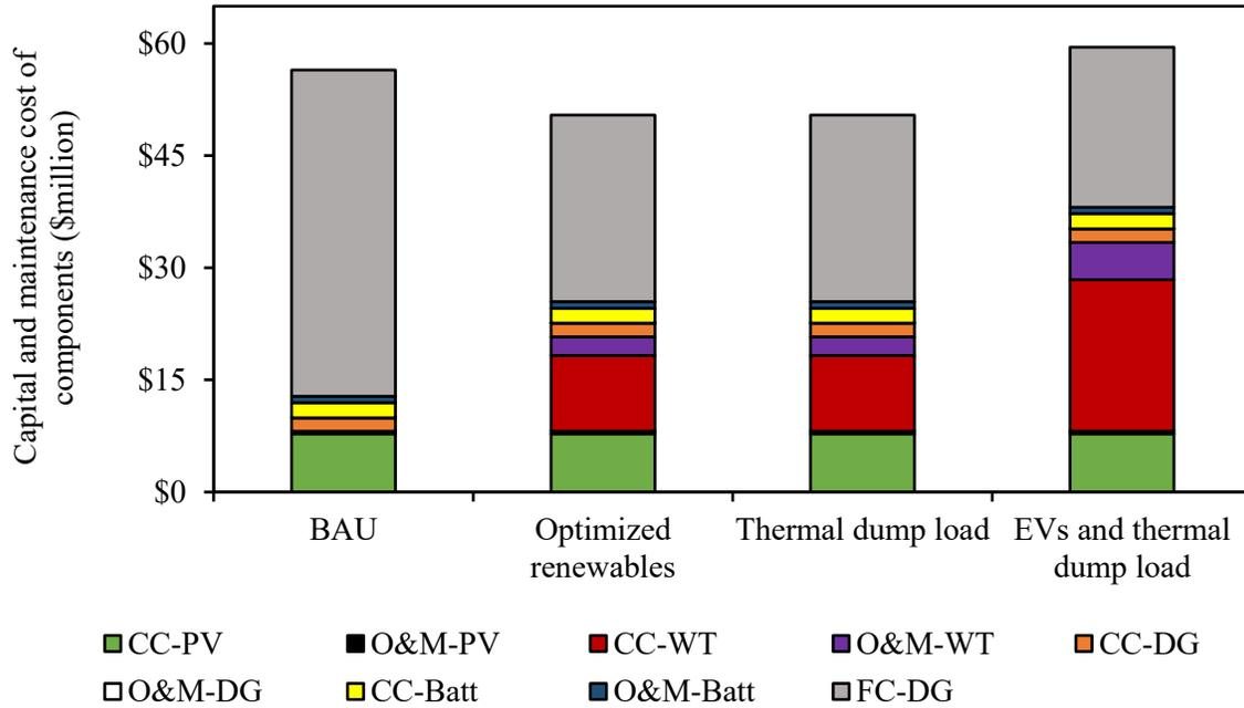
**Figure 16: Capital and maintenance cost of components for cost minimization scenarios**
