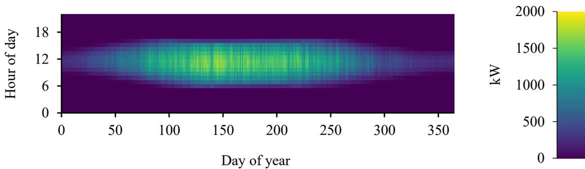
**Figure 19: Daily power output of solar PV for EVs and thermal dump load scenario**
