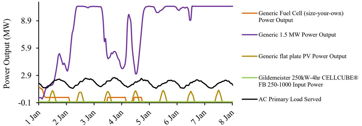
**Figure 23: Hourly dispatch of energy for EVs and hydrogen heating scenario**
