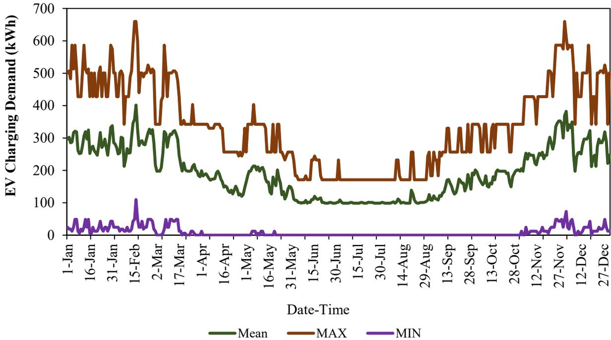
**Figure 8: Simulated EV load for Fort Chipewyan**
