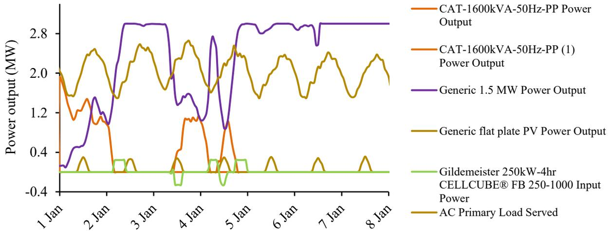
**Figure 18: Hourly dispatch of energy for EVs and thermal dump load scenario**
