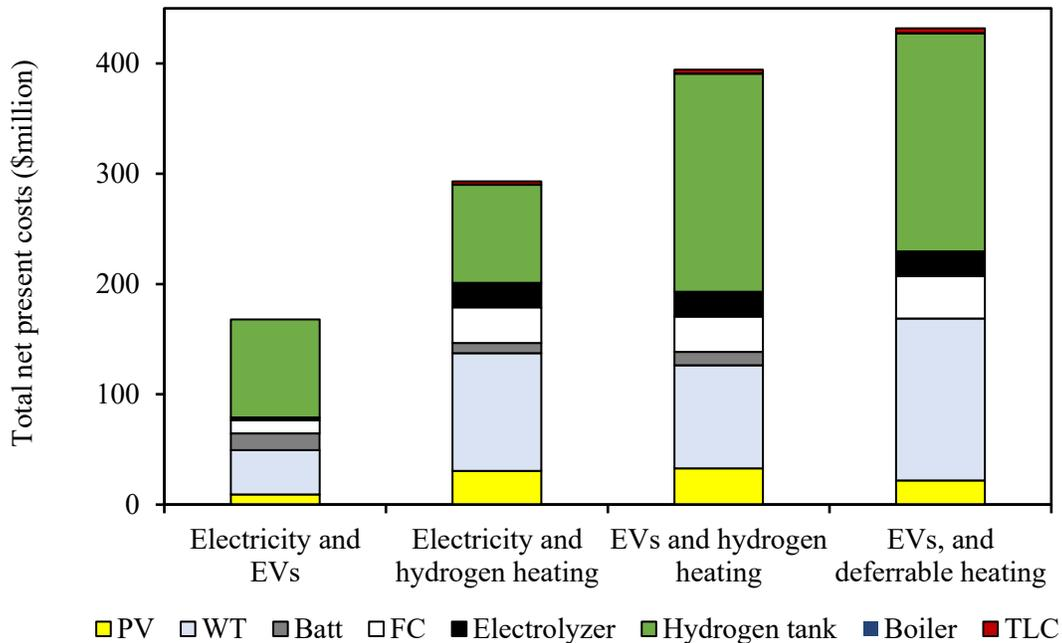
**Figure 20: Total net present cost of components for deep carbonization scenarios**
