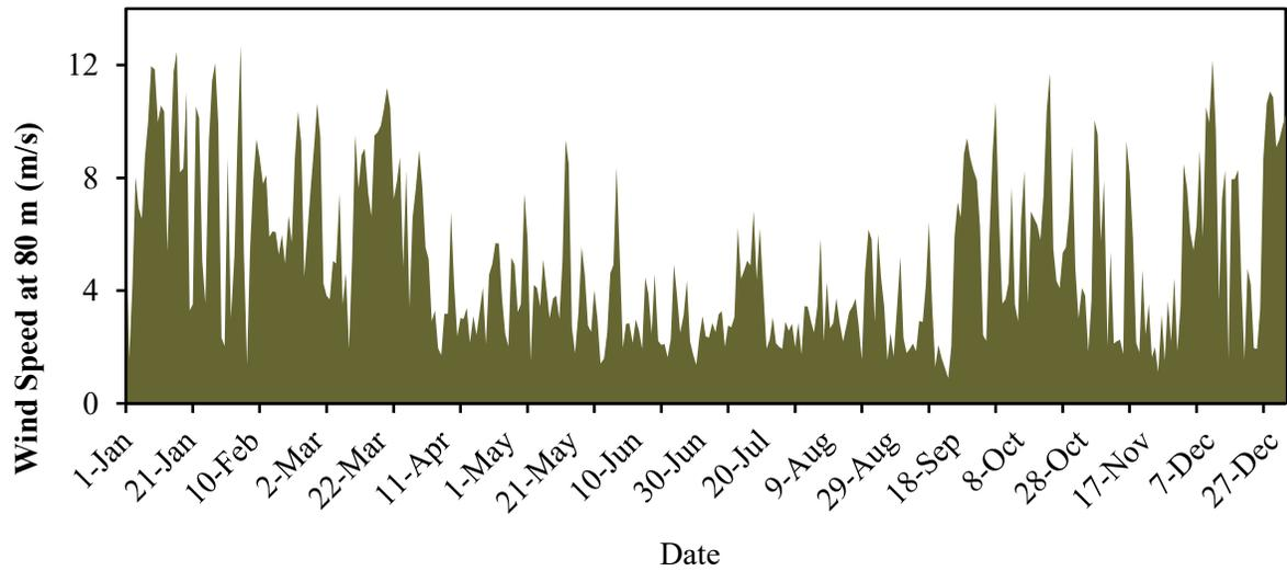
**Figure 12: 10-minute averaged wind speeds at Fort Chipewyan for a typical meteorological year [136]**
