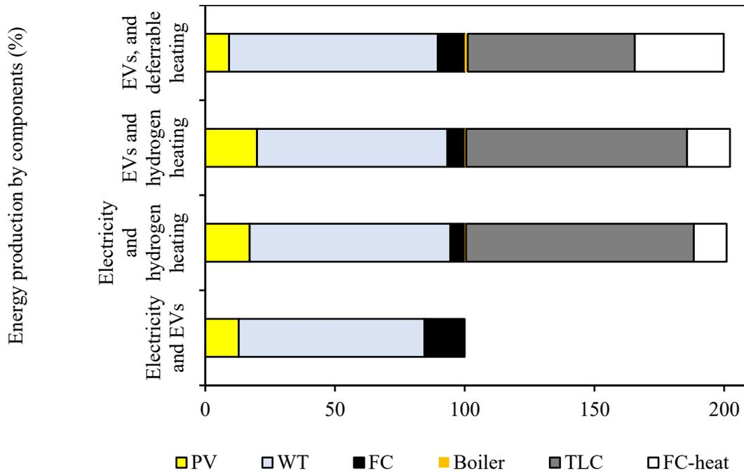
Figure 22: Electricity and heating production by components for deep carbonization scenarios
