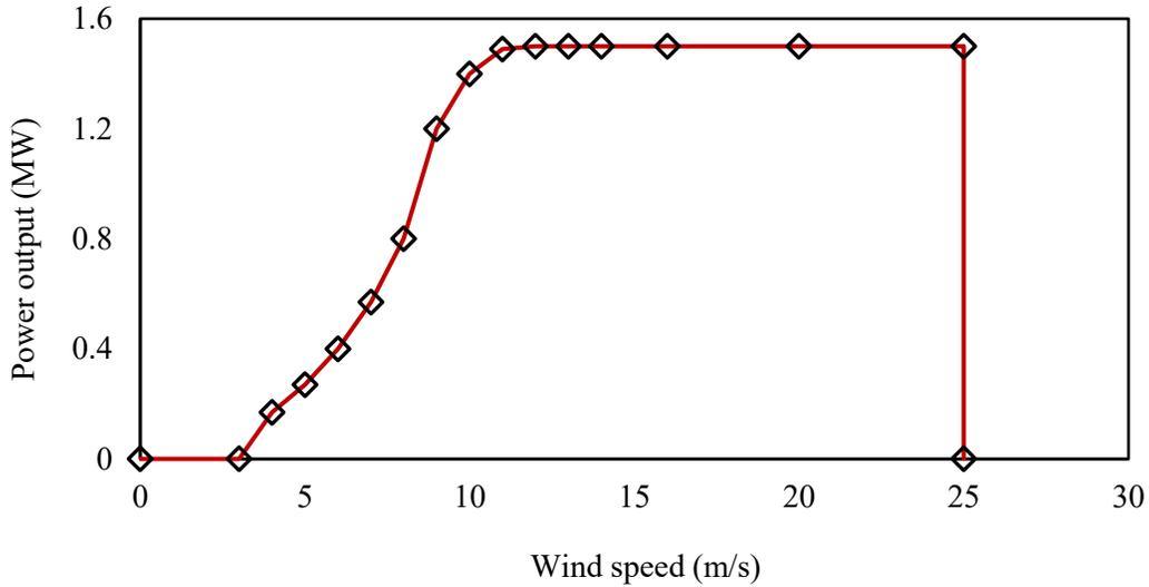
**Figure 28: Wind turbine power output curve**
