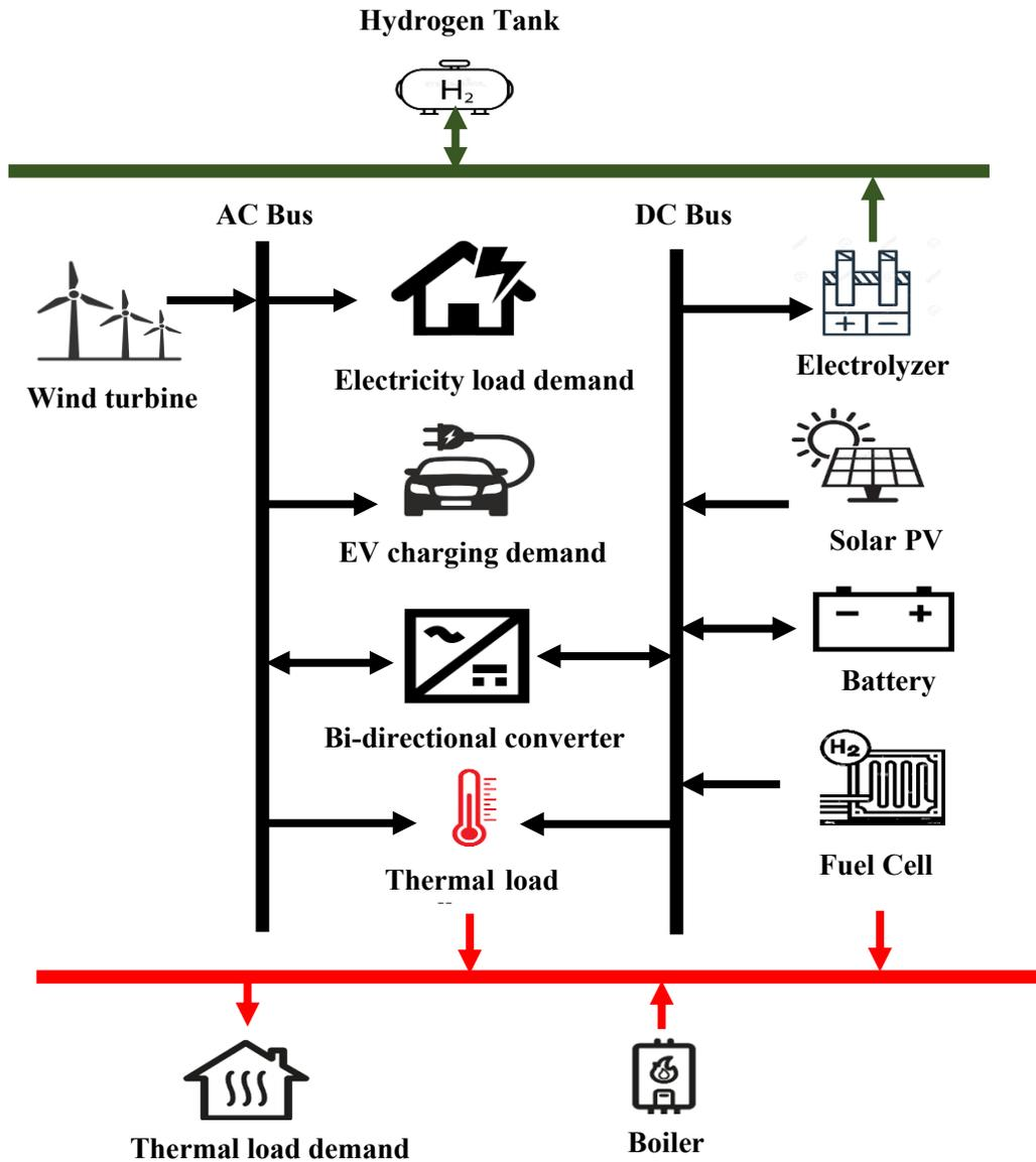
**Figure 3: Schematic of the proposed HRES**
