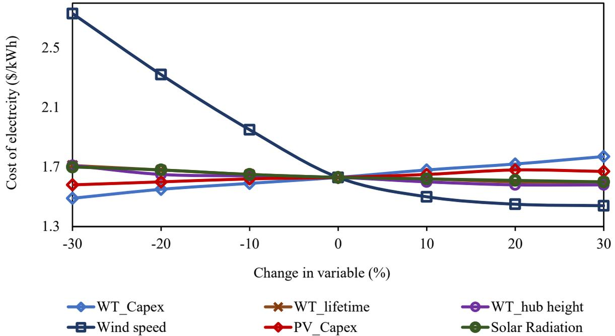
**Figure 25: Sensitivity analysis to check the impact on COE of electricity and hydrogen heating scenario**
