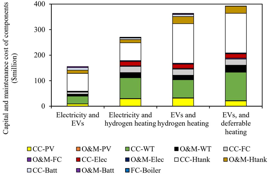
Figure 21: Capital and maintenance cost of components for deep carbonization scenarios
