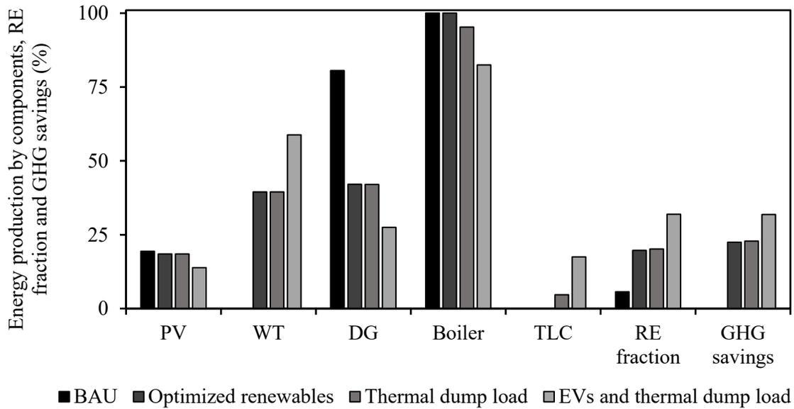
**Figure 17: Electricity and heating production by components (%), the renewable fraction (%), and emissions reduction (%) for cost minimization scenarios**
