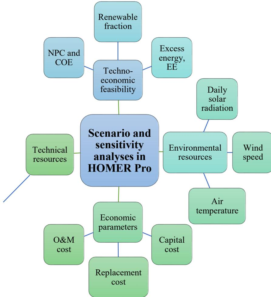
**Figure 2: Inputs to the optimization model**
