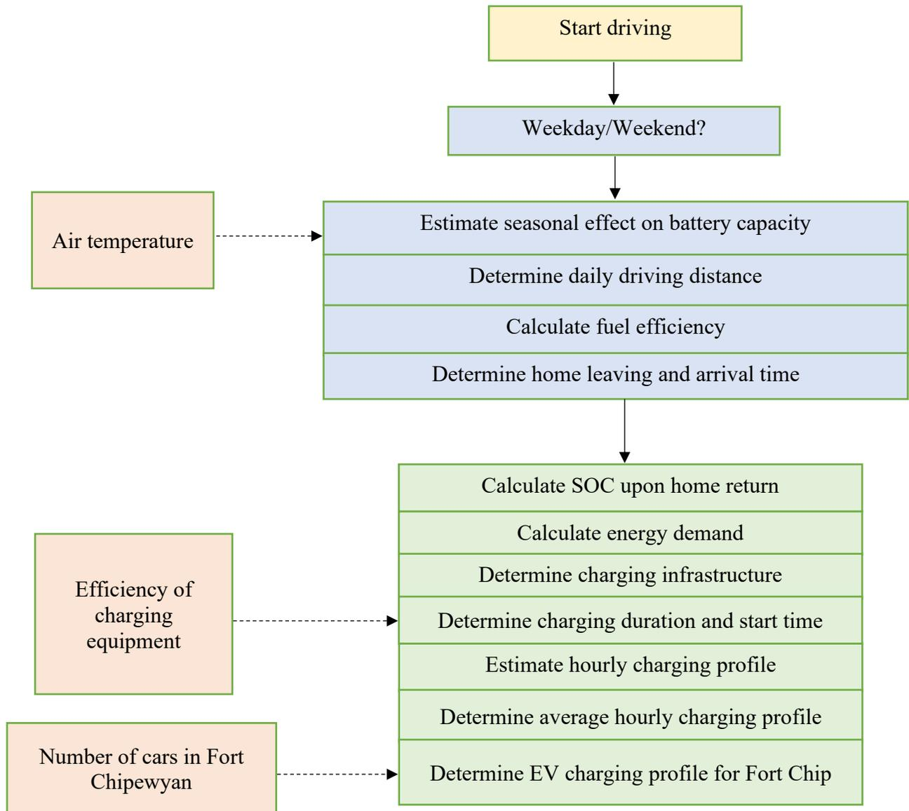
**Figure 7: Design framework of hourly EV charging profile**
