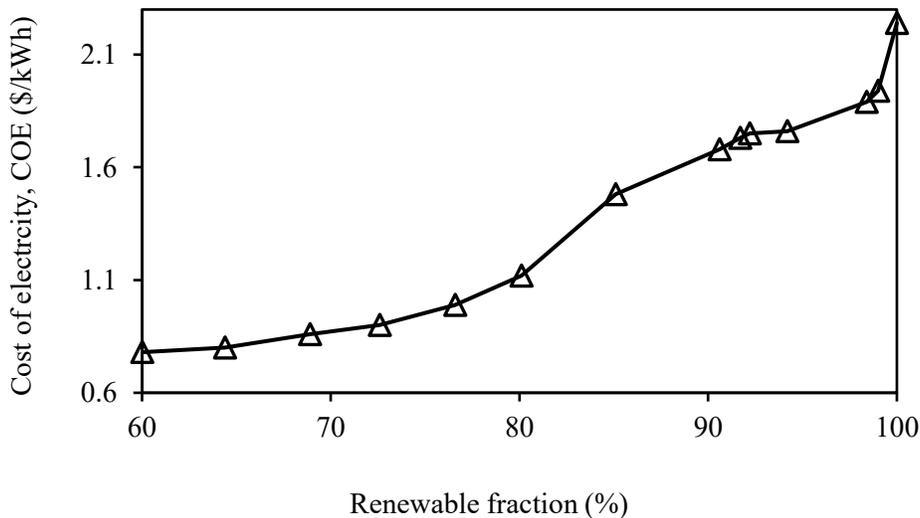
**Figure 27: Increasing trend of COE with renewable fraction for EVs and hydrogen heating scenario**
