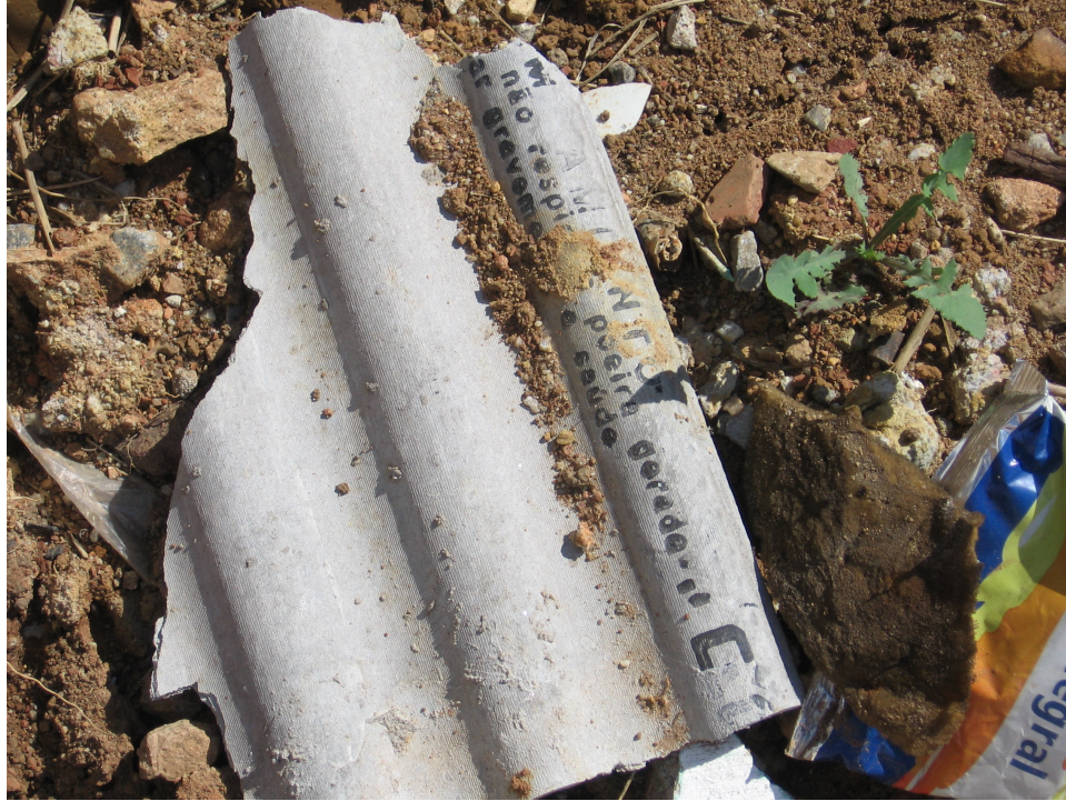
Asbestos-cement waste, text translates to “Warning: do not breathe; may be dangerous to your health” ©Kyla Elizabeth Sentes, 2006
