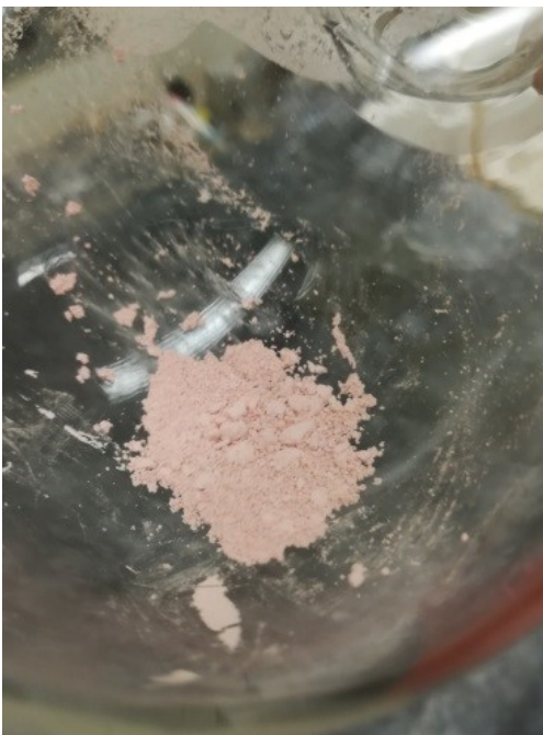
Figure 2-6. BaSO 4 supported ester hydrogenation catalyst, 124 .
