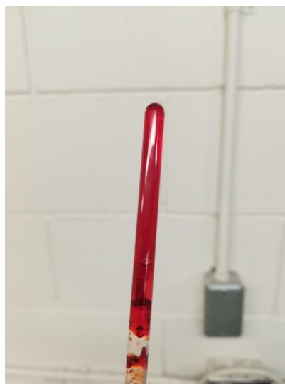
Figure 2-5. A representative picture of an NMR tube containing the polymerized catalyst gel that does not flow with shaking.
