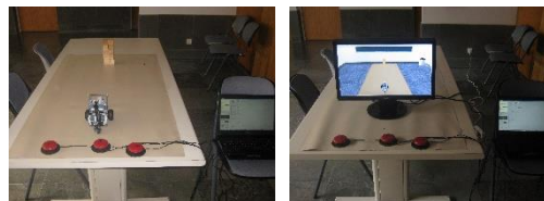
Figure 5. Experimental setup with the physical and the virtual robots
