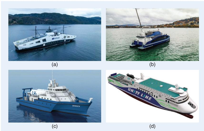
**Figure 2.** Hydrogen fuel cell-powered marine vessels: (a) the *MF Hydra* in Norway; (b) the *Switch* passenger ferry in the United States; (c) the *Zero-V* research vessel in the United States; and (d) the Polish ferry *Unity Line*, which will be operated in the Baltic Sea.
