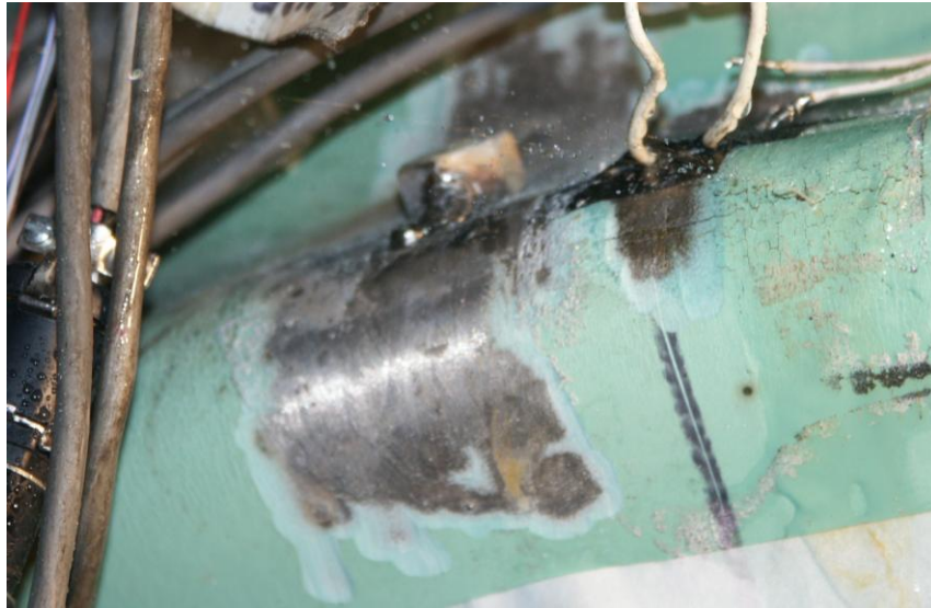
Figure 4.33: Pressurized water spraying from specimen LCF20N1
