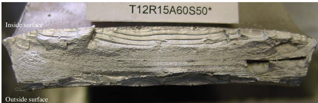
Figure A.6 Pictures of fracture surface: strip specimen series of T12R15A60
