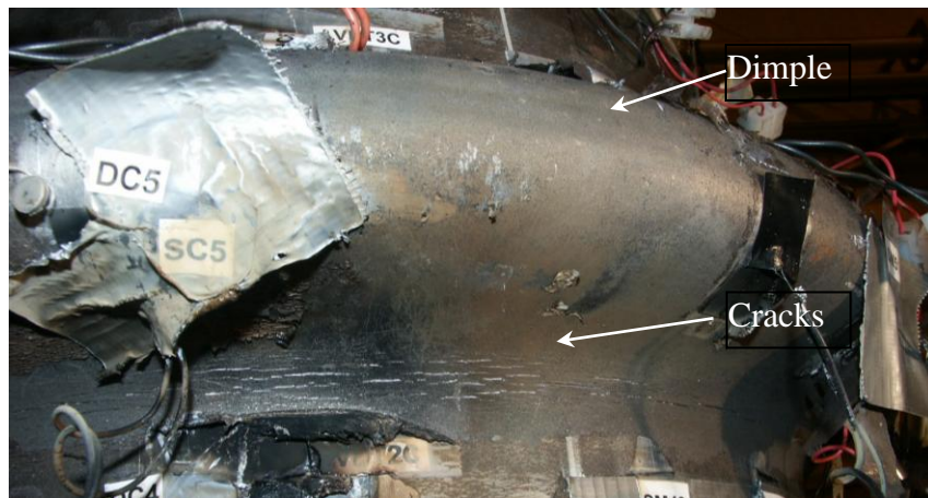
Figure 4.30: Cracks on the lower wrinkle foot and dimple formed on wrinkle crest (specimen LCF16N1)
