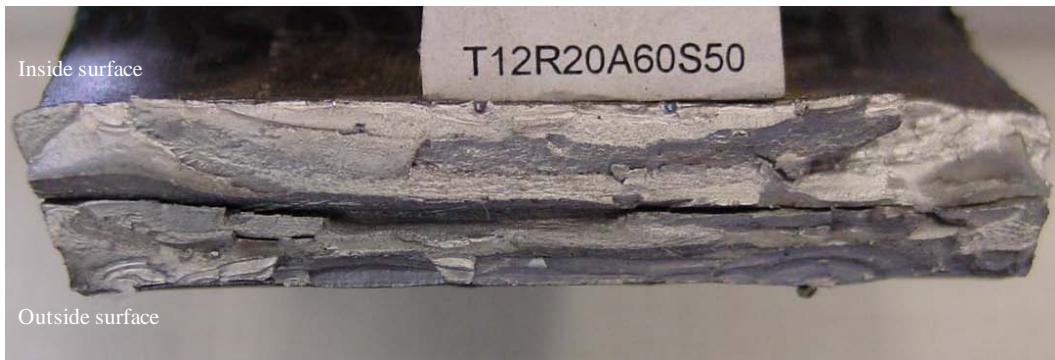
Figure A.8 Pictures of fracture surface: strip specimen series of T12R20A60
