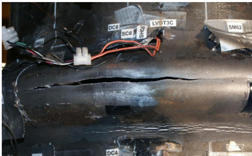
Figure 4.31: Wrinkle crest on concave side being totally fractured (LCF16N1)
