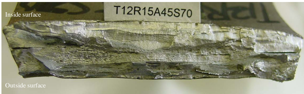
Figure A.5 Pictures of fracture surface: strip specimen series of T12R15A45
