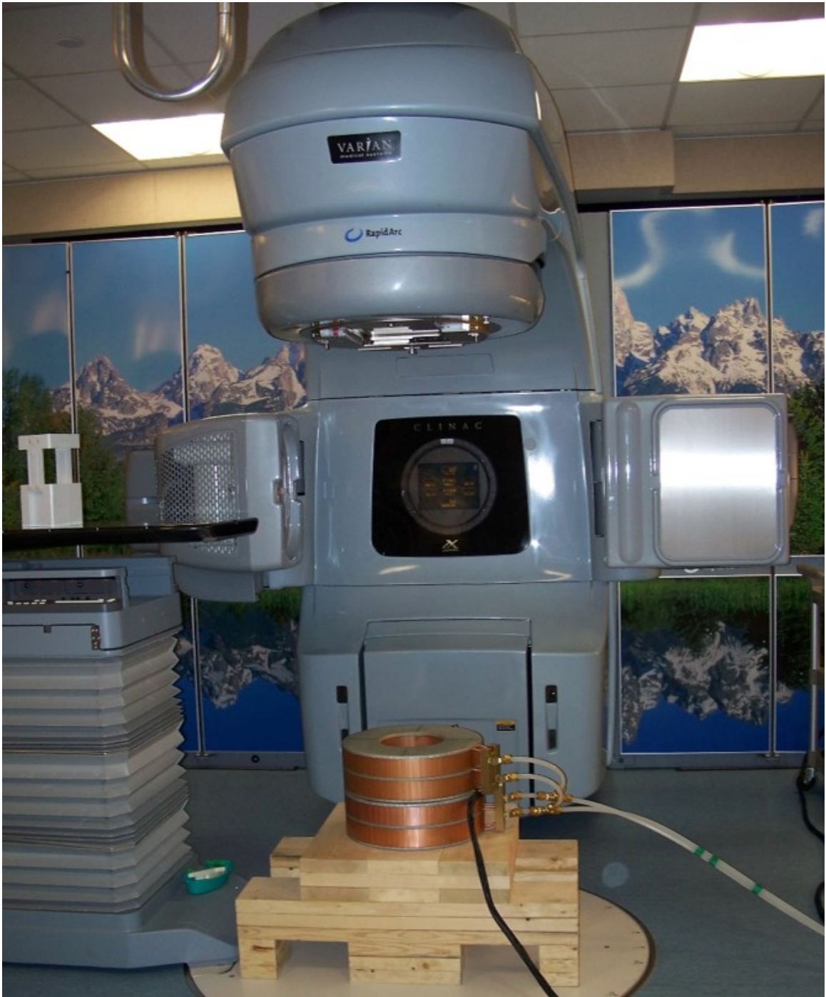
Figure 3.2: A photograph of the dual solenoid magnet positioned at the center of the light field at an SSD of 170 cm to the top of the magnets.
