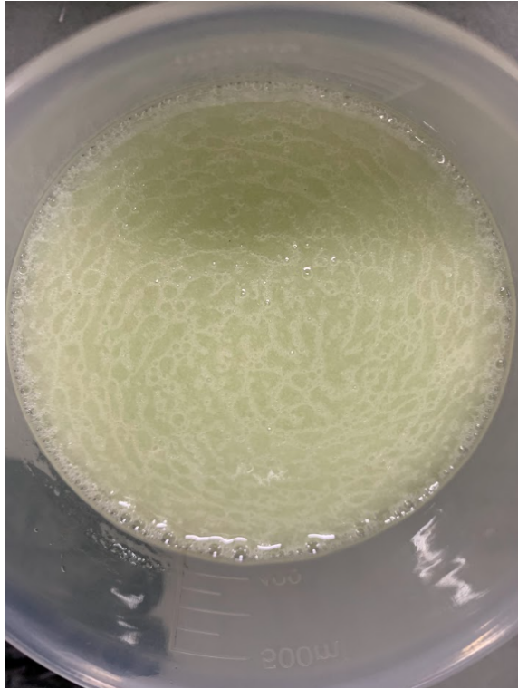
Figure 2.2: An example of a not fully separated 80% water cut emulsion (top view). (courtesy of Sand Separation Technologies)
