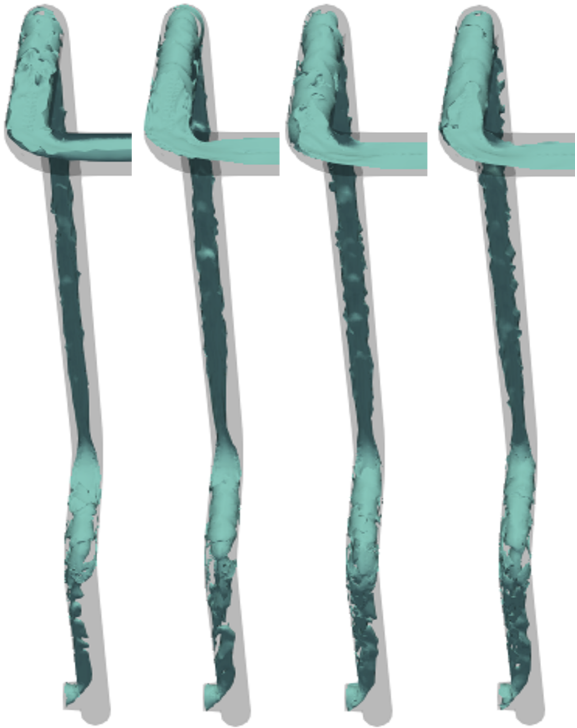
Figure 4.16: The contour plot of the free surface obtained from multiphaseEmulsion-Foam case at 10, 20, 30 and 40 s, respectively.
