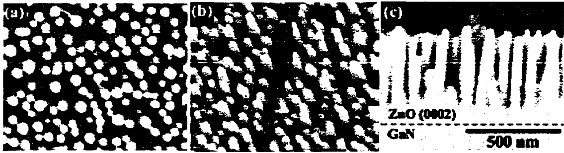
Fig 8 SEM images of 1% ZnO on C-plane GaN: (a) Top view, (b) 60° tilted view, and (c) cross-section view. The scale bar applies to all images [43].
