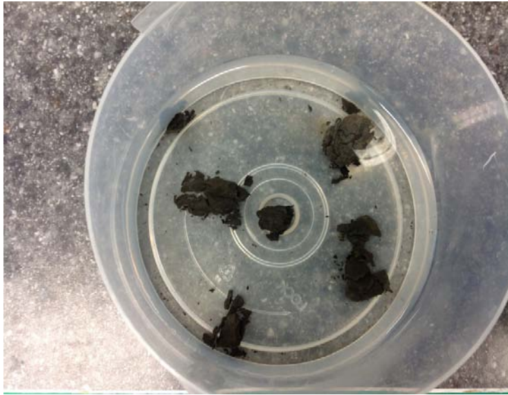
Figure 5-1 Disintegration of shale samples after 48 hours
