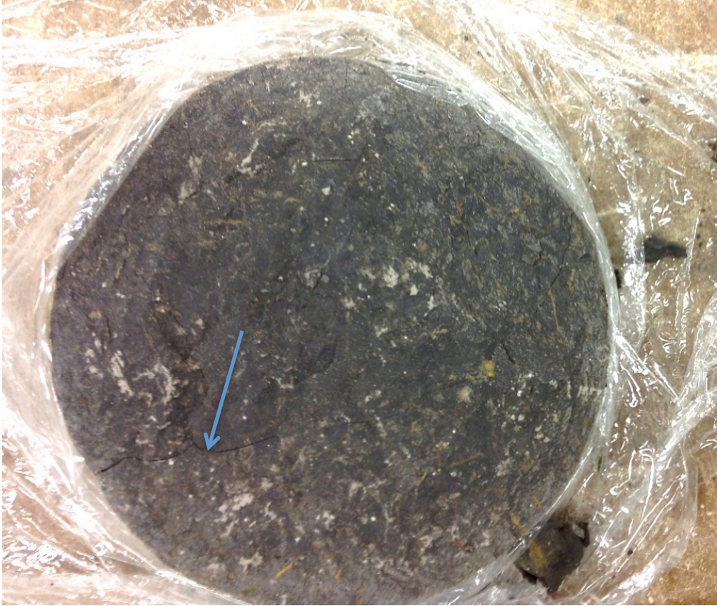
Figure 5-9 Fissures in Lea Park shale core
