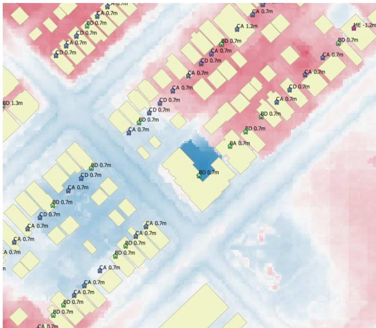
Figure 2-1: Example of spatially represented building inventory showing building type and main floor height. Yellow geometry shows the measured building foot prints, red/blue shading shows a WSL raster shaded by depth above the DEM.
