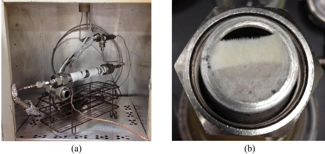
**Figure 3.4** Horizontal configuration of the reactor to measure phenolic acids solubility in water (a). Picture showing the layers of phenolic acid (upper part) and sand (lower part) inside the reactor after a solubility measurement (b).
