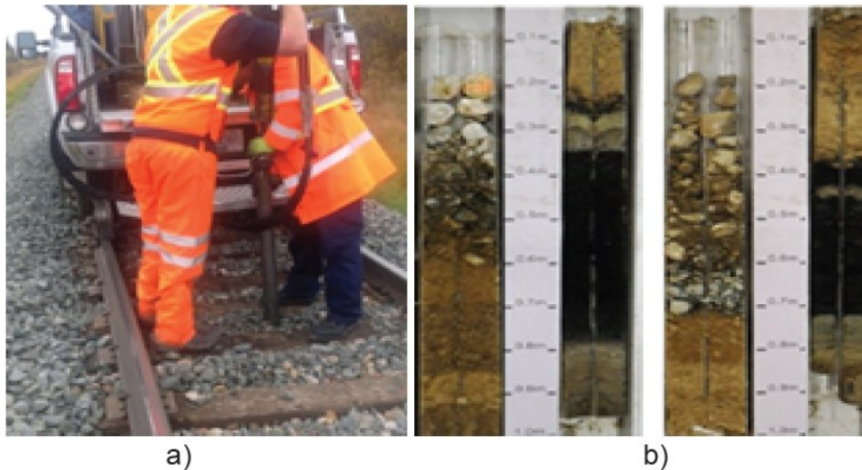
Figure A-7. Figure shows a) taking sample at LLBS and b) two samples taken from LLBS
