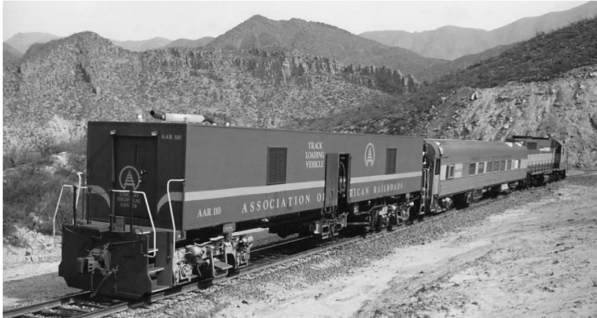
Figure 2-11. Track Loading Vehicle (Li et al., 2004)
