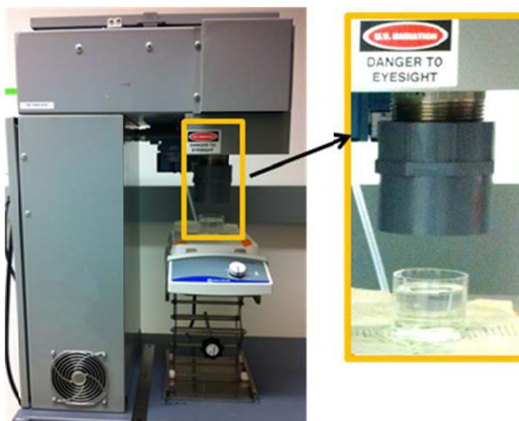
**Figure 4.1** Quasi-collimated beam UV apparatus
