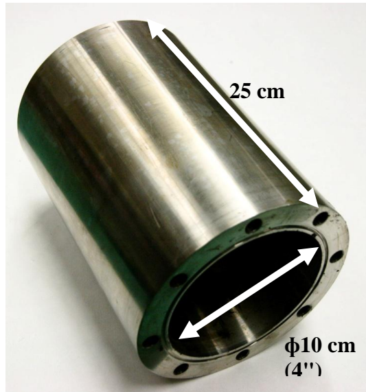
Figure 6-1: High pressure /temperature cylinder used for carbonate experiments
