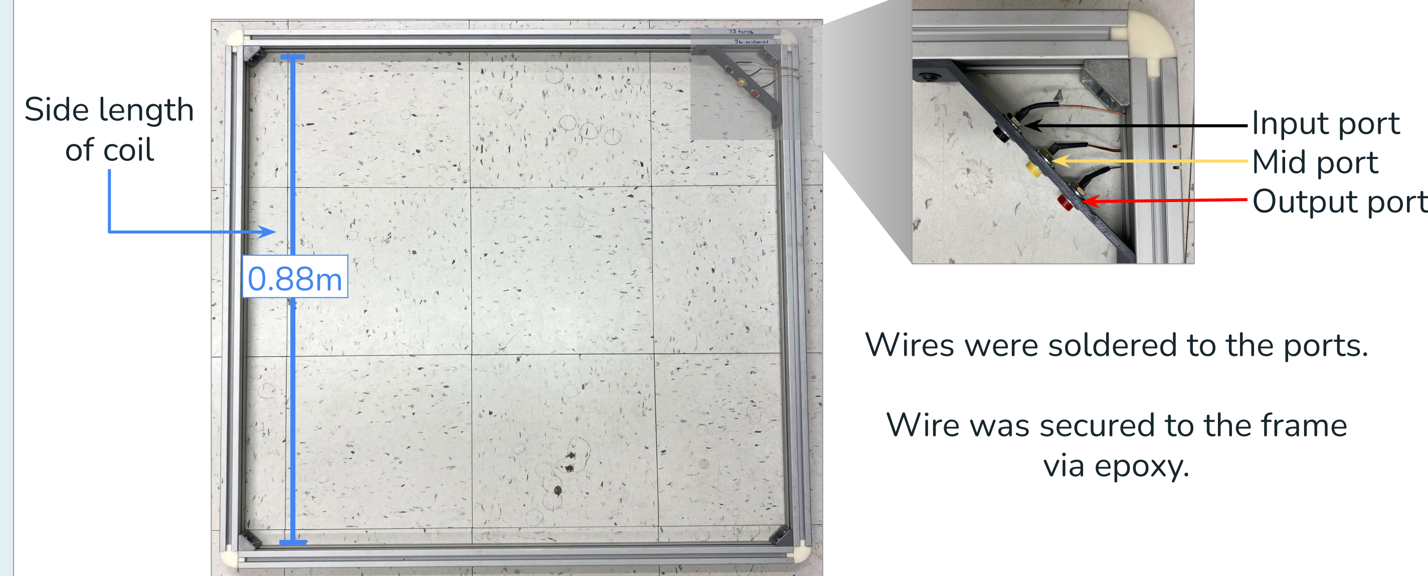
Fig 7. A completed coil
