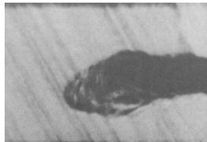
(b) Cavity failure pattern for Core No. 1
