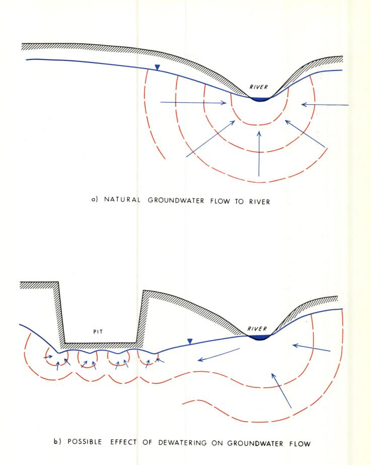
FIG. 5 EFFECT OF DEWATERING
