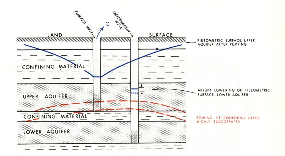
FIG. 13 DIAGRAM SHOWING THE EFFECT ON A DEEP ARTESIAN AQUIFER OF PUMPING FROM AN OVERLYING ARTESIAN AQUIFER causing failure of overlying confining beds may exist anywhere in the Oil Sands area.
