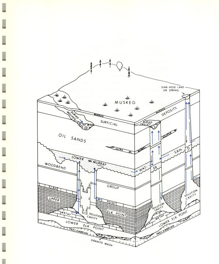
FIG. 15 SKETCH SHOWING POSSIBLE EFFECTS OF SALT SOLUTION ON GROUNDWATER SYSTEMS (not to scale)
