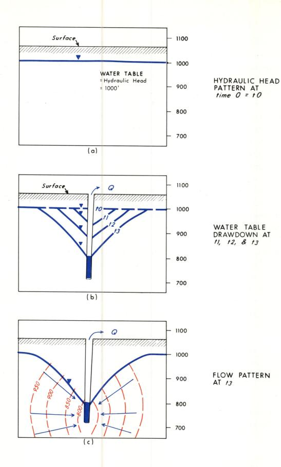
FIG. 3 DRAWDOWN IN A WELL PUMPED AT RATE Q
