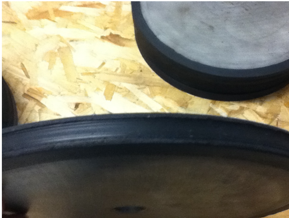
Figure 19 - Worn rubber wheel after wet test with PU
