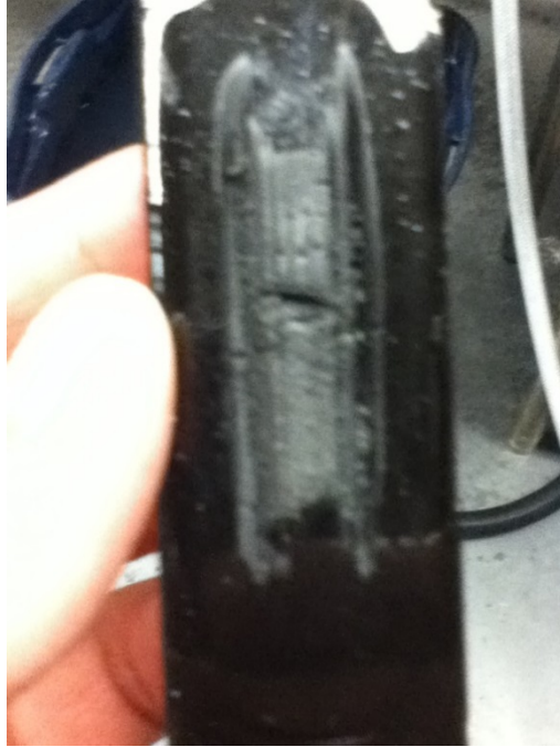
Figure 18 - Wear scar on PU sample tested with rubber wheel
