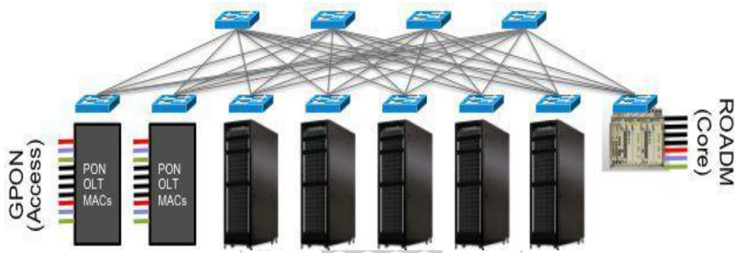
Fig5.1. Target hardware built from commodity servers, I/O Blades, and switches.
