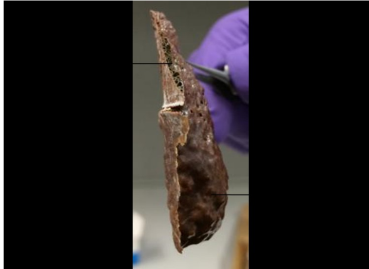
Figure 4: Difference in surface and cross section area of the slag layer in top section of furnace
