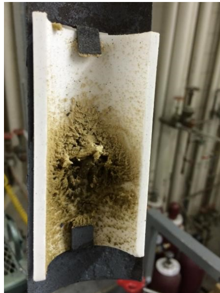
Figure 4.4: Particle deposition on the ceramic plate (T=1200°C, θ=60°)
