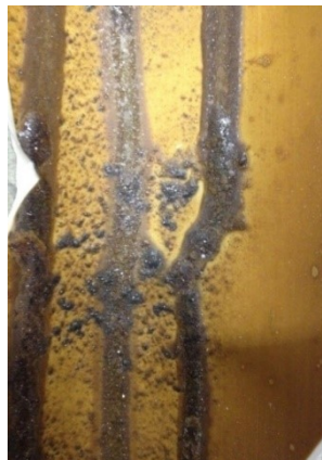
Figure 5.15: Experimental results of slag flow on the wall of gasifier
