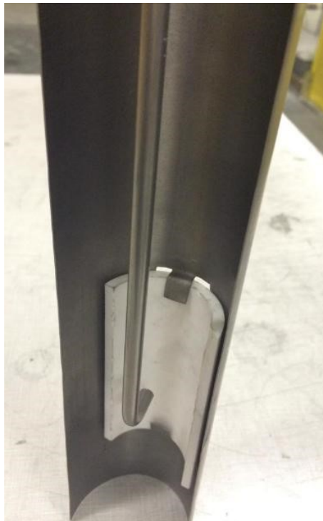
Figure 4.2: Injection set up including injector tube, removable ceramic plate and holder metal sheet
