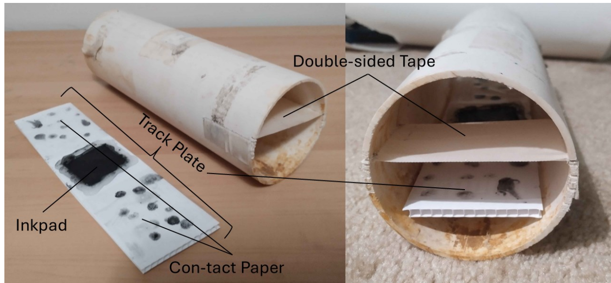
Fig. 3.1 Combination track and hair tube used to monitor small rodents. From October through December 2023, we monitored coyote and mouse-sized rodent activity at bird feeders in residential yards near urban greenspaces in Edmonton, Alberta ( n = 44 ).
