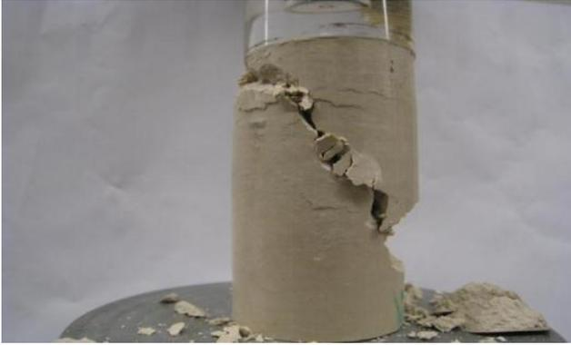
Figure B.20 Photo after UC test for sample-2:  $A_c=0.01\%$ ,  $w=22\%$ , 7-day moisture room dry
