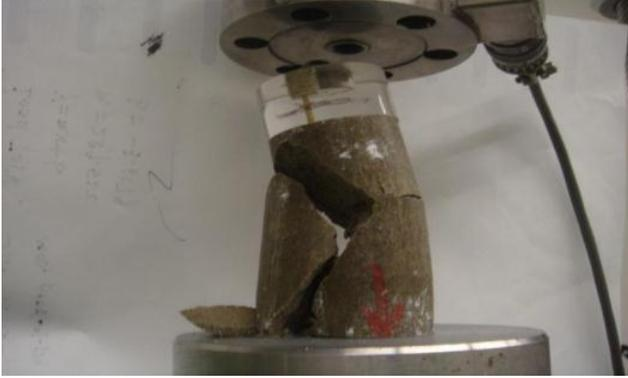
Figure C.4 Photo after UC test for Sample-1:  $A_c=0.01\%$ ,  $w=32\%$ , 21-day moisture room dry
