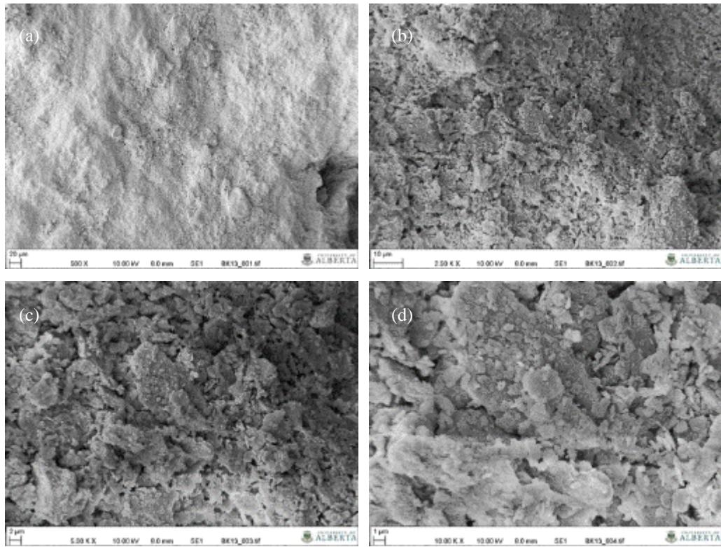
Figure G.8 Photomicrographs of BK20 in unconfined compression test at  $w=28\%$ ,  $T_c=7$  days,
