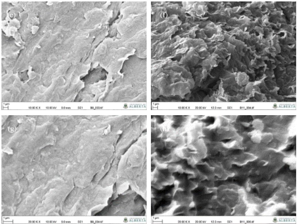
Figure G.5 Photomicrographs of bentonite in unconfined compression test at  $w=32\%$ ,  $T_c=21$  days, (a)  $A_c=0\%$ ,  $M\sim 500X$ ; (b)  $A_c=0.25\%$ ,  $M\sim 500X$ ; (c)  $A_c=0\%$ ,  $M\sim 5,000X$ ; (d)  $A_c=0.25\%$ ,  $M\sim 5,000X$ ; (e)  $A_c=0\%$ ,  $M\sim 10,000X$ ; (f)  $A_c=0.25\%$ ,  $M\sim 10,000X$ ; (g)  $A_c=0\%$ ,  $M\sim 20,000X$ ; (h)  $A_c=0.25\%$ ,  $M\sim 20,000X$ .
