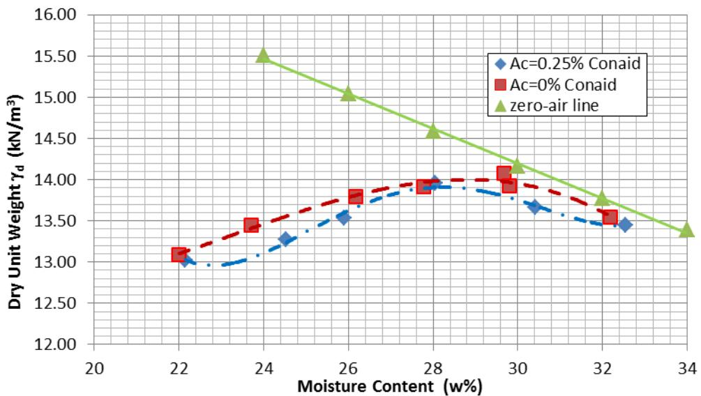
Figure 4.5 Standard Proctor compaction curves for bentonite-kaolinite Mixture
