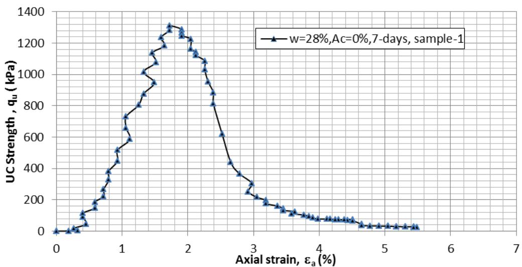
Figure D.9  $q$  vs.  $\varepsilon_a$  for  $A_c=0\%$ ,  $w=28\%$ , 7-day air dry, sample-1
