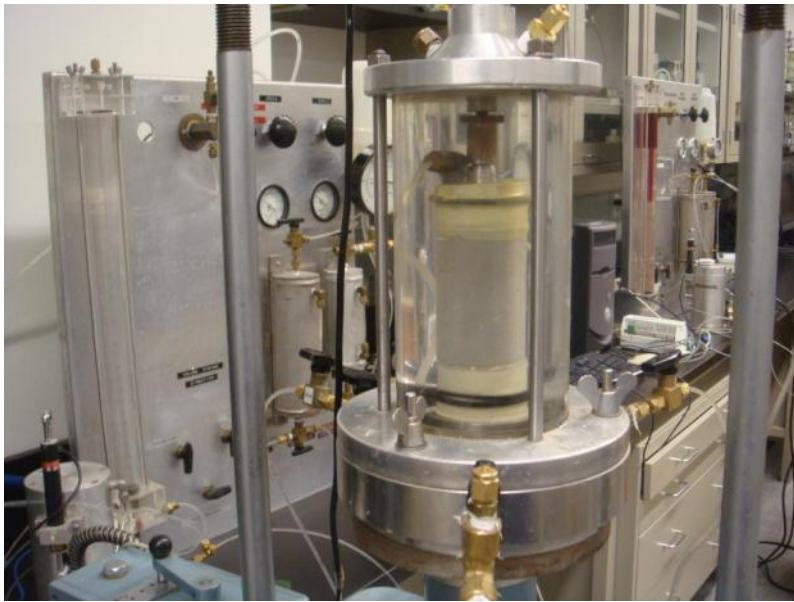
Figure 3.2 Photo of triaxial test apparatus
