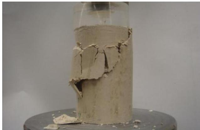
Figure B.16 Photo after UC test for sample-2:  $A_c=0.05\%$ ,  $w=22\%$ , 7-day moisture room dry
