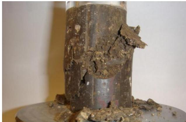
Figure F.4 Photo after UC test for sample-2:  $A_c=0.025\%$ ,  $w=17\%$ , 5-day moisture room dry
