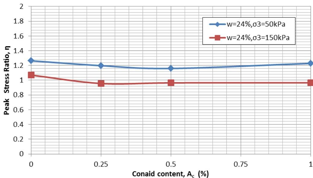
Figure 5.2 Peak stress ratio vs. Conaid content for CD tests at confining pressures of 50kPa and 150kPa
