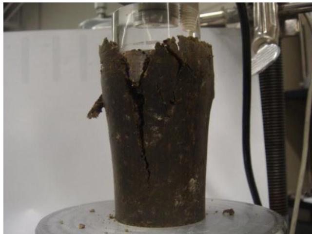
Figure F.8 Photo after UC test for sample-1:  $A_c=0.025\%$ ,  $w=17\%$ , 0-day (as-molded)
