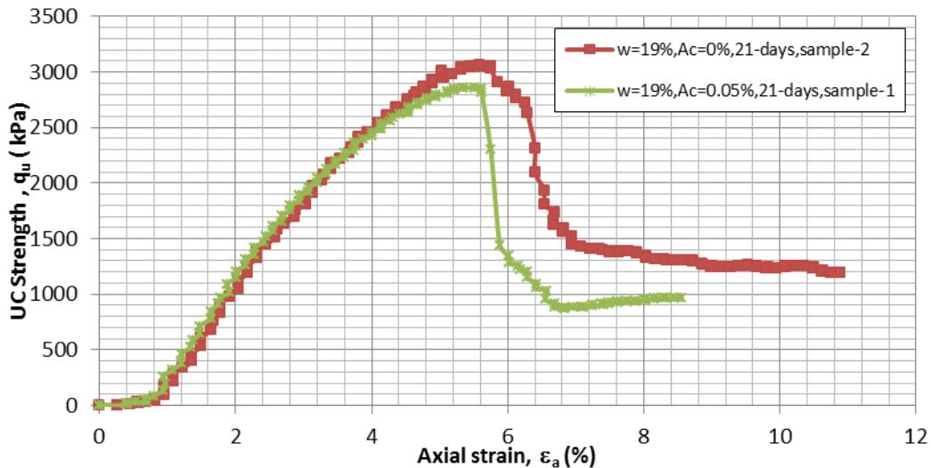
Figure 5.28 UC stress- strain curve for  $w=19\%$ ,  $T_c=21$  days
