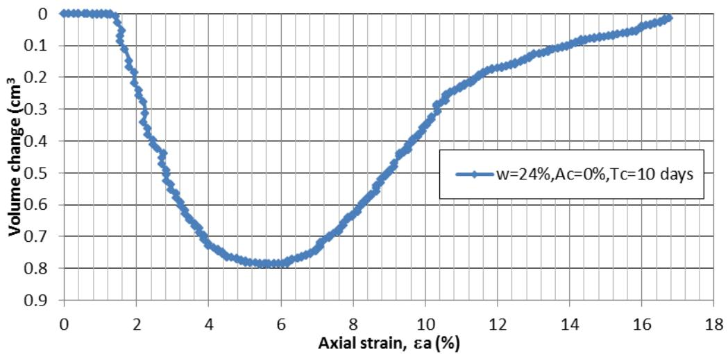
Figure A.2 Volume change vs.  $\epsilon_a$  for  $Ac=0\%$ ,  $w=24\%$ , 10-day &  $p_0'=150\text{kPa}$
