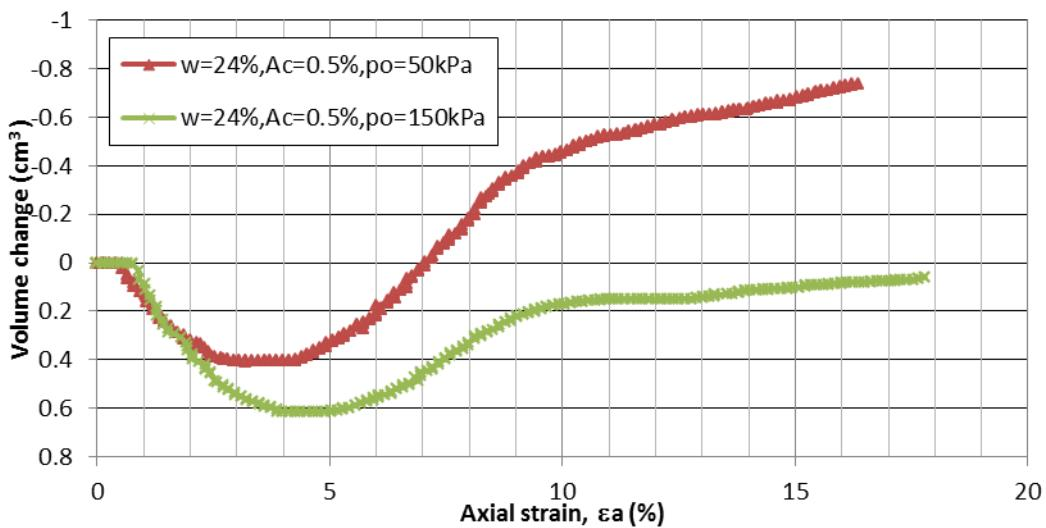
Figure 5.9 Volume change vs.  $\epsilon_a$  for  $w=24\%$  &  $p_0'=50\text{kPa}$ ,  $150\text{kPa}$
