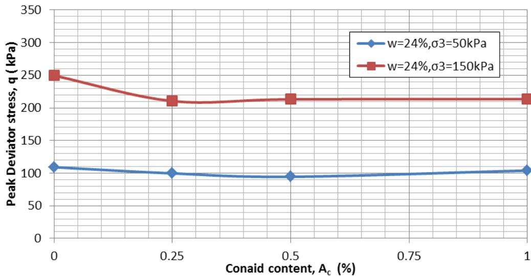
Figure 5.1 Peak deviator stress vs. Conaid content for CD tests at confining pressures of 50kPa and 150kPa
