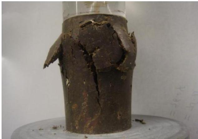
Figure F.6 Photo after UC test for sample-1:  $A_c=0\%$ ,  $w=17\%$ , 0-day (as-molded)
