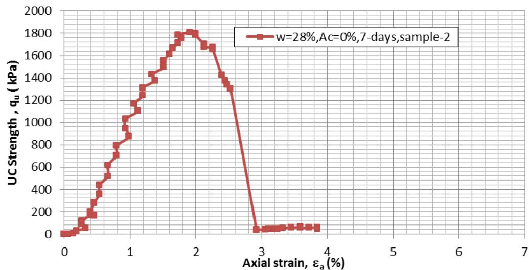
Figure D.11  $q$  vs.  $\epsilon_a$  for  $A_c=0\%$ ,  $w=28\%$ , 7-day air dry, sample-2
