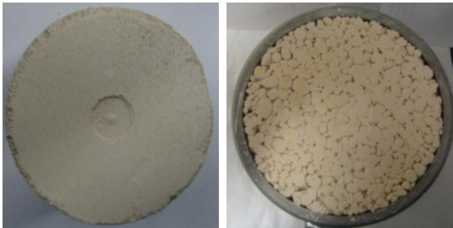
Figure 4.1 Compacted samples with and without passing No.8 sieve (2.36 mm)
