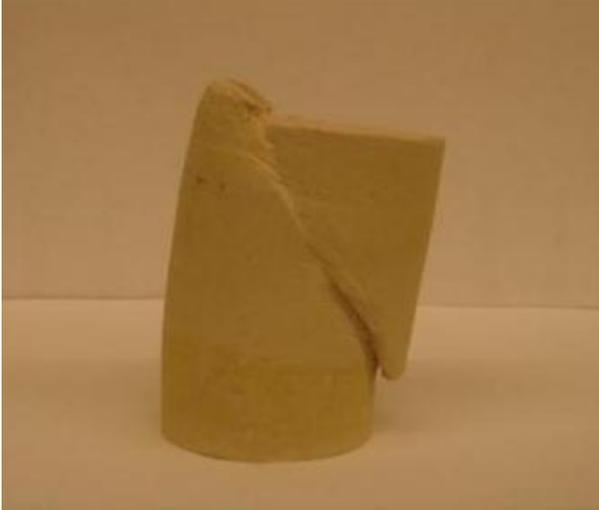
Figure A.10 Photo after CD test for Sample:  $A_c=0.25\%$ ,  $w=24\%$ , 17-day &  $p_0'=50\text{kPa}$
