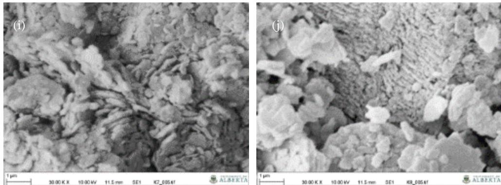
Figure G.4 Photomicrographs of kaolinite in unconfined compression test at  $w=24\%$ ,  $T_c=7$  days, (a)  $A_c=0\%$ ,  $M\sim 500X$ ; (b)  $A_c=0.25\%$ ,  $M\sim 500X$ ; (c)  $A_c=0\%$ ,  $M\sim 2,500X$ ; (d)  $A_c=0.25\%$ ,  $M\sim 2,500X$ ; (e)  $A_c=0\%$ ,  $M\sim 5,000X$ ; (f)  $A_c=0.25\%$ ,  $M\sim 5,000X$ ; (g)  $A_c=0\%$ ,  $M\sim 10,000X$ ; (h)  $A_c=0.25\%$ ,  $M\sim 10,000X$ ; (i)  $A_c=0\%$ ,  $M\sim 30,000X$ ; (j)  $A_c=0.25\%$ ,  $M\sim 30,000X$ .
