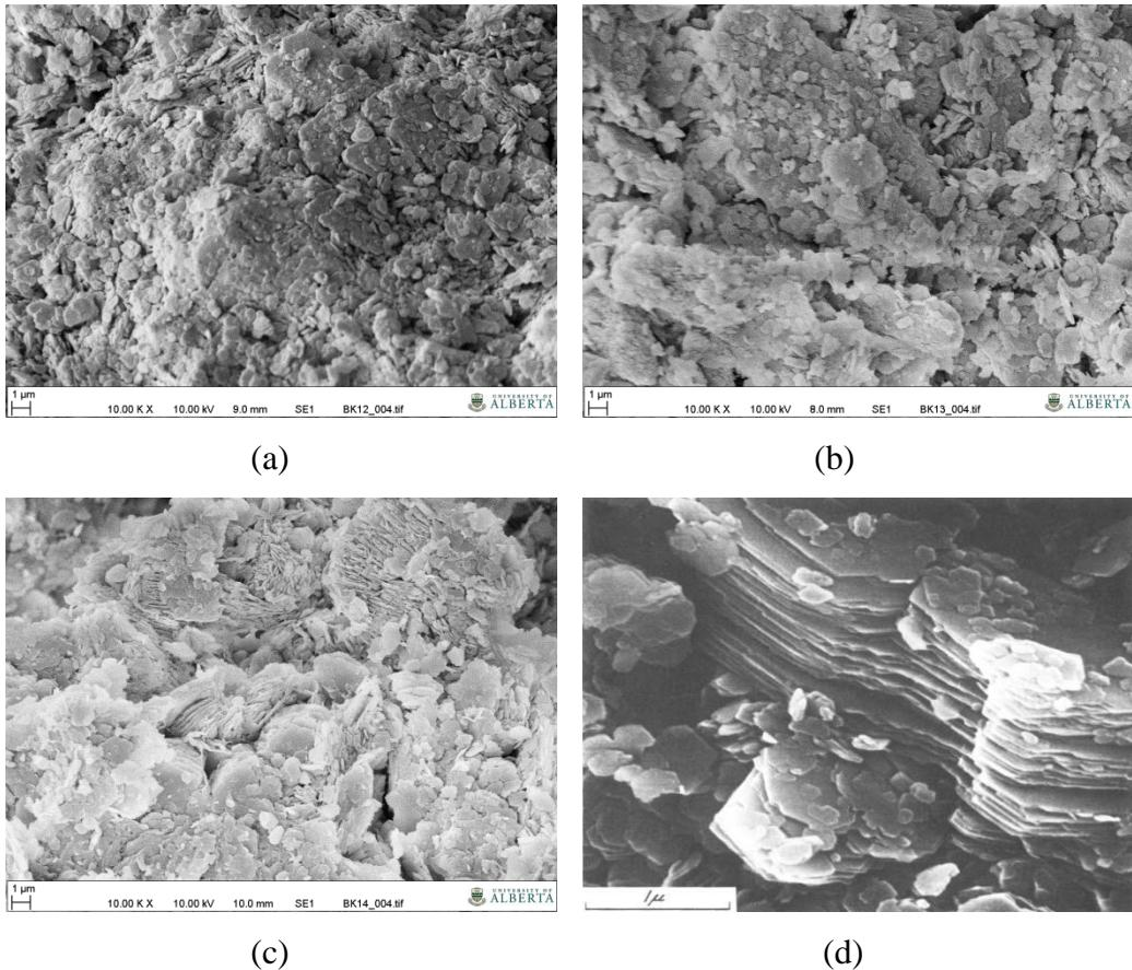
Figure 6.5 Photomicrographs of BK20 at  $w=28\%$ ,  $T_c=7$  days and  $M\sim 10,000X$ , (a)  $A_c=0\%$ ; (b)  $A_c=0.025\%$ ; (c)  $A_c=0.25\%$ ; (d) kaolinite after Terzaghi (1996)
