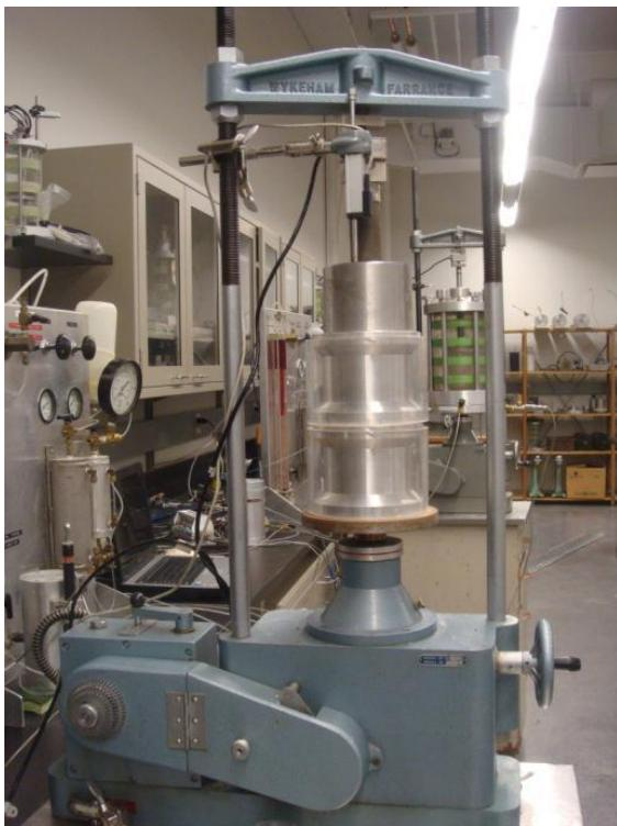
Figure 3.3 Photo of unconfined compression test apparatus
