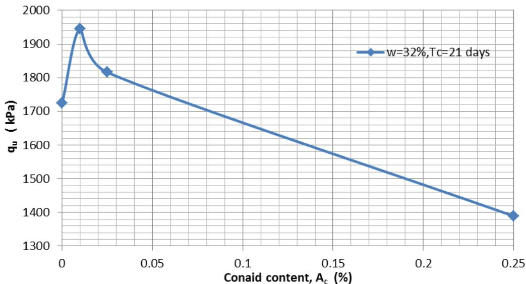
Figure 5.19 UC peak strength vs. Conaid content for  $w=32\%$ ,  $T_c=21$  days
