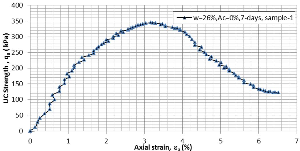
Figure D.1  $q$  vs.  $\epsilon_a$  for  $A_c=0.25\%$ ,  $w=26\%$ , 7-day moisture room dry, sample-1
