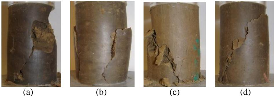
Figure 5.29: Photos of specimens after UC test: (a)  $A_c=0\%$ ,  $w=16.5\%$ , 12-day moisture room dry; (b)  $A_c=0.05\%$ ,  $w=16.5\%$ , 12-day moisture room dry; (c)  $A_c=0\%$ ,  $w=19\%$ , 21-day moisture room dry; (d)  $A_c=0.05\%$ ,  $w=19\%$ , 21-day moisture room dry.
