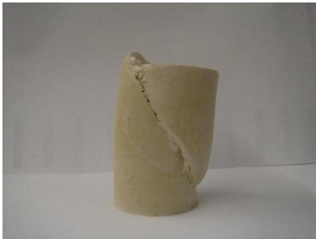
Figure A.13 Photo after CD test for Sample:  $A_c=0.5\%$ ,  $w=24\%$ , 16-day &  $p_0'=150\text{kPa}$
