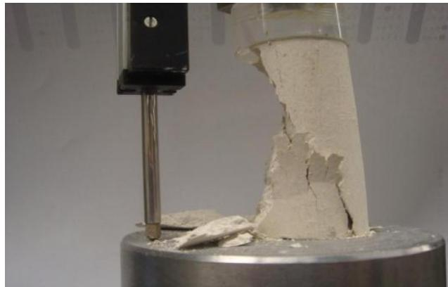
Figure D.12 Photo after UC test for sample-2:  $A_c=0\%$ ,  $w=28\%$ , 7-day air dry
