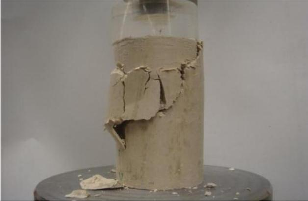
Figure B.16 Photo after UC test for sample-2:  $A_c=0.05\%$ ,  $w=22\%$ , 7-day moisture room dry
