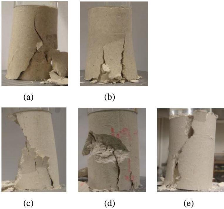
Figure 5.26: Photos of specimens after UC test: (a)  $A_c=0\%$ ,  $w=26\%$ , 7-day moisture room dry; (b)  $A_c=0.25\%$ ,  $w=26\%$ , 7-day moisture room dry; (c)  $A_c=0\%$ ,  $w=28\%$ , 7-day air dry; (d)  $A_c=0.025\%$ ,  $w=28\%$ , 7-day air dry; (e)  $A_c=0.25\%$ ,  $w=28\%$ , 7-day air dry moisture
