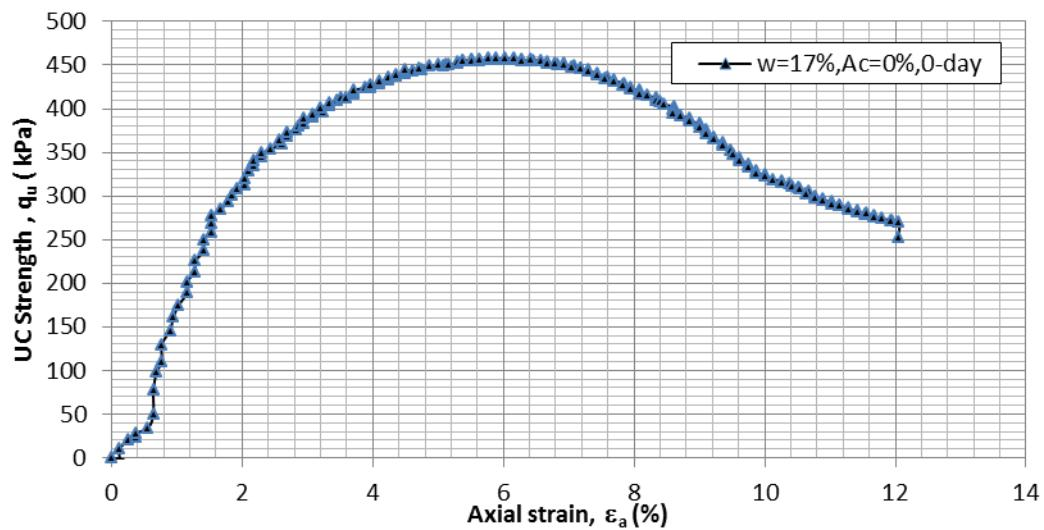
Figure F.5  $q$  vs.  $\epsilon_a$  for  $A_c=0\%$ ,  $w=17\%$ , 0-day (as-molded), sample-1
