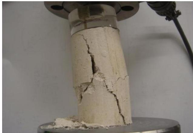
Figure D.24 Photo after UC test for sample-2:  $A_c=0\%$ ,  $w=28\%$ , 90-day air dry
