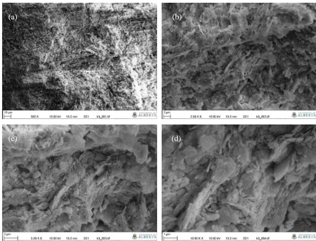
Figure G.3 Photomicrographs of kaolinite in drained triaxial test at  $w=24\%$ ,  $A_c=0.5\%$ ,  $T_c=16$  days, (a)  $M\sim 500X$ ; (b)  $M\sim 2,500X$ ; (c)  $M\sim 5,000X$ ; (d)  $M\sim 10,000X$ .
