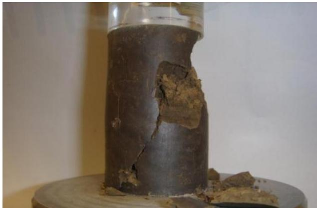
Figure E.4 Photo after UC test for sample-2:  $A_c=0\%$ ,  $w=16.5\%$ , 12-day moisture room dry
