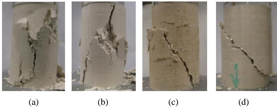
Figure 5.17: Photos of specimens after UC test: (a)  $A_c=0\%$ ,  $w=24\%$ , 7-day air dry; (b)  $A_c=0.25\%$ ,  $w=24\%$ , 7-day air dry; (c)  $A_c=0\%$ ,  $w=22\%$ , 7-day moisture room dry; (d)  $A_c=0.01\%$ ,  $w=22\%$ , 7-day moisture room dry
