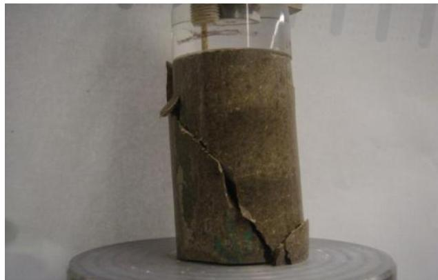
Figure C.18 Photo after UC test for sample-1:  $A_c=0\%$ ,  $w=27\%$ , 31-day moisture room dry
