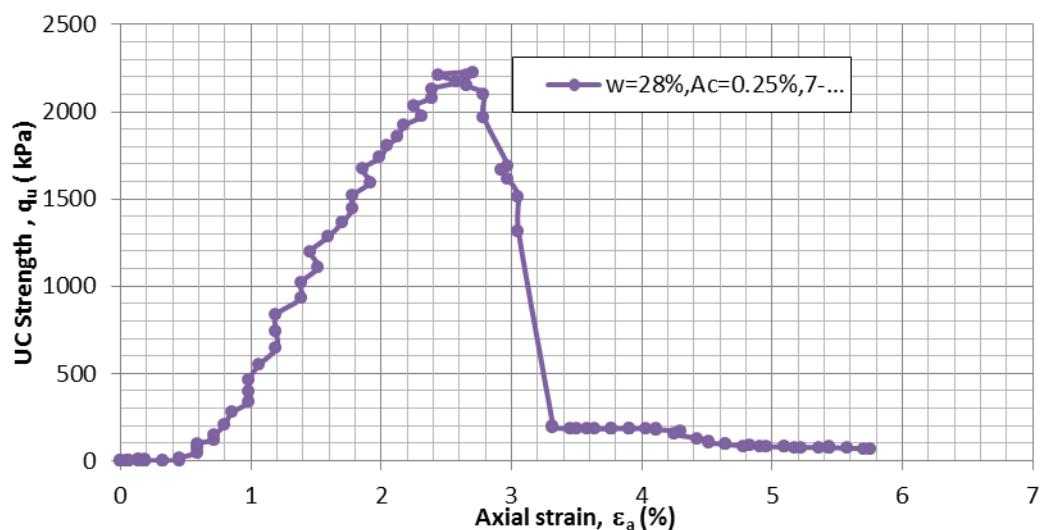
Figure D.19  $q$  vs.  $\epsilon_a$  for  $A_c=0.25\%$ ,  $w=28\%$ , 7-day air dry, sample-2
