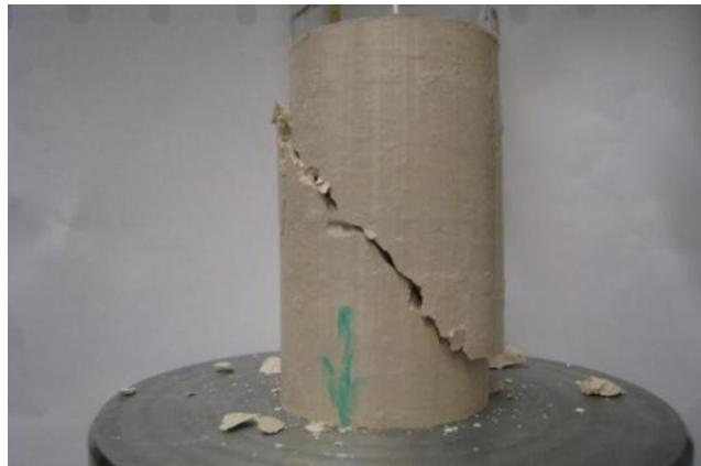
Figure B.18 Photo after UC test for sample-1:  $A_c=0.01\%$ ,  $w=22\%$ , 7-day moisture room dry
