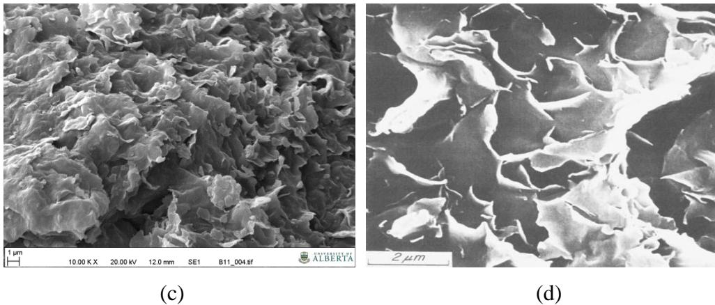
Figure 6.4 Photomicrographs of bentonite at  $w=32\%$ ,  $T_c=21$  days and  $M \sim 10,000X$ , (a)  $A_c=0\%$ ; (b)  $A_c=0.025\%$ ; (c)  $A_c=0.25\%$ ; (d) montmorillonite after Terzaghi (1996)
