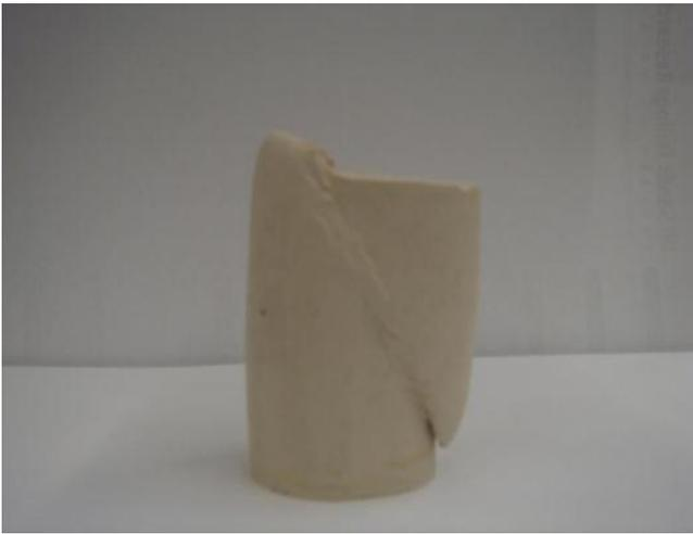
Figure A.15 Photo after CD test for Sample:  $A_c=0.5\%$ ,  $w=24\%$ , 16-day &  $p_0'=50\text{kPa}$
