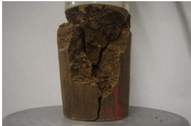
Figure E.8 Photo after UC test for Sample-2:  $A_c=0.05\%$ ,  $w=16.5\%$ , 12-day moisture room dry
