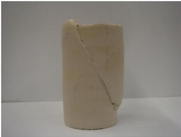
Figure A.3 Photo after CD test for Sample:  $Ac=0\%$ ,  $w=24\%$ , 10-day &  $p_0'=150\text{kPa}$
