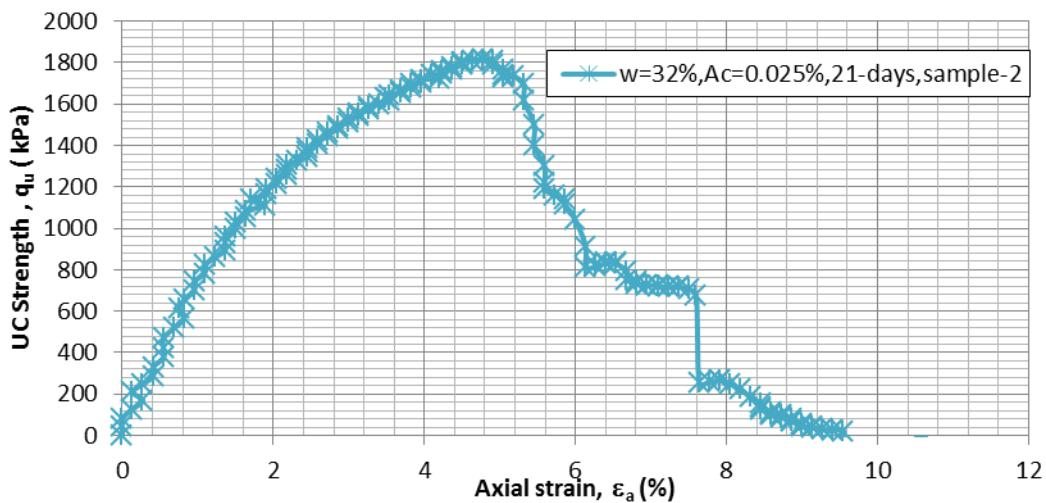
Figure C.7  $q$  vs.  $\epsilon_a$  for  $A_c=0.025\%$ ,  $w=32\%$ , 21-day moisture room dry, sample-2
