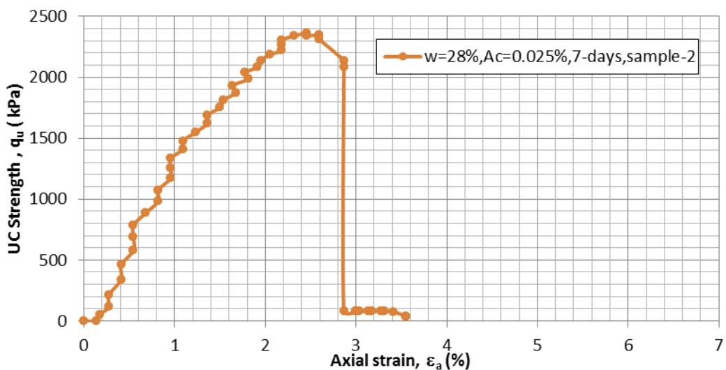
Figure D.15  $q$  vs.  $\varepsilon_a$  for  $A_c=0.025\%$ ,  $w=28\%$ , 7-day air dry, sample-2
