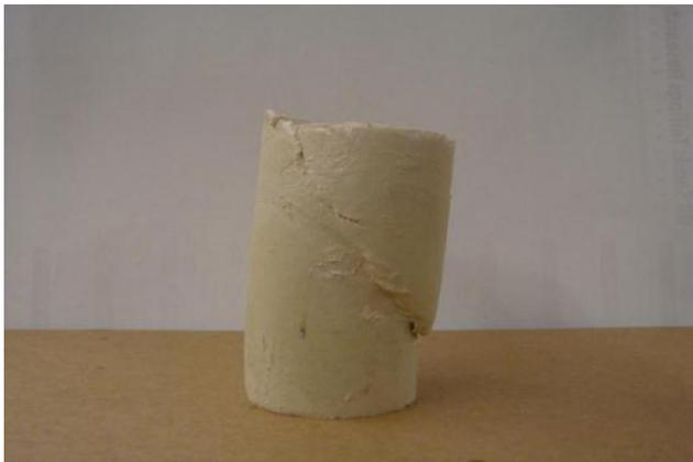
Figure A.17 Photo after CD test for Sample:  $A_c=1\%$ ,  $w=24\%$ , 14-day &  $p_0'=150\text{kPa}$
