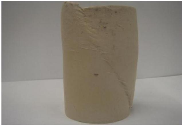
Figure A.5 Photo after CD test for Sample:  $A_c=0\%$ ,  $w=24\%$ , 10-day &  $p_0'=50\text{kPa}$
