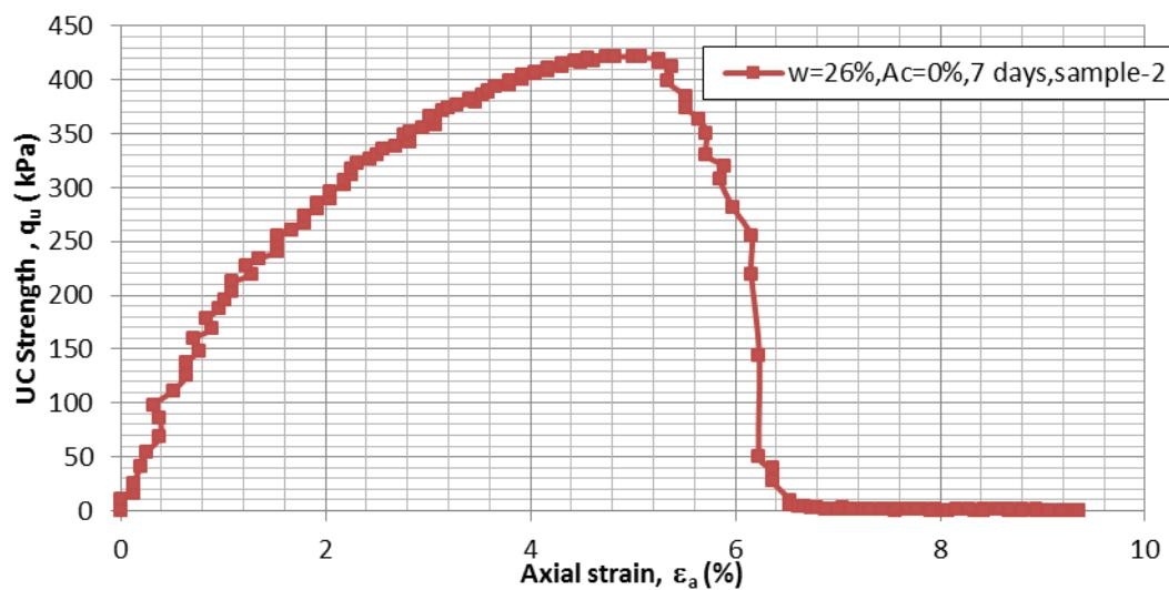
Figure D.7  $q$  vs.  $\epsilon_a$  for  $A_c=0\%$ ,  $w=26\%$ , 7-day moisture room dry, sample-2
