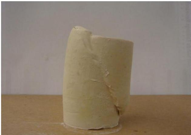
Figure A.19 Photo after CD test for Sample:  $A_c=1\%$ ,  $w=24\%$ , 14-day &  $p_0'=50\text{kPa}$
