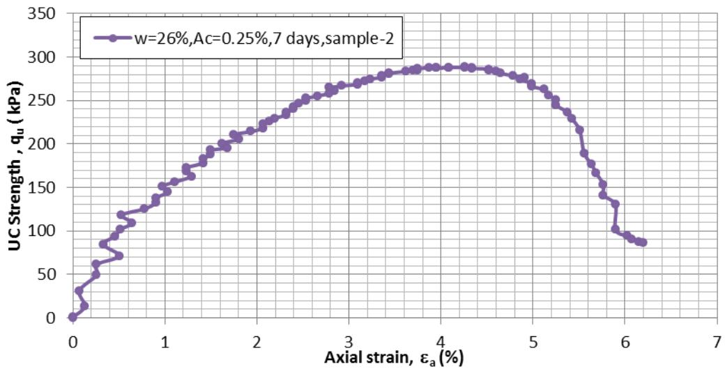
Figure D.3  $q$  vs.  $\varepsilon_a$  for  $A_c=0.25\%$ ,  $w=26\%$ , 7-day moisture room dry, sample-2
