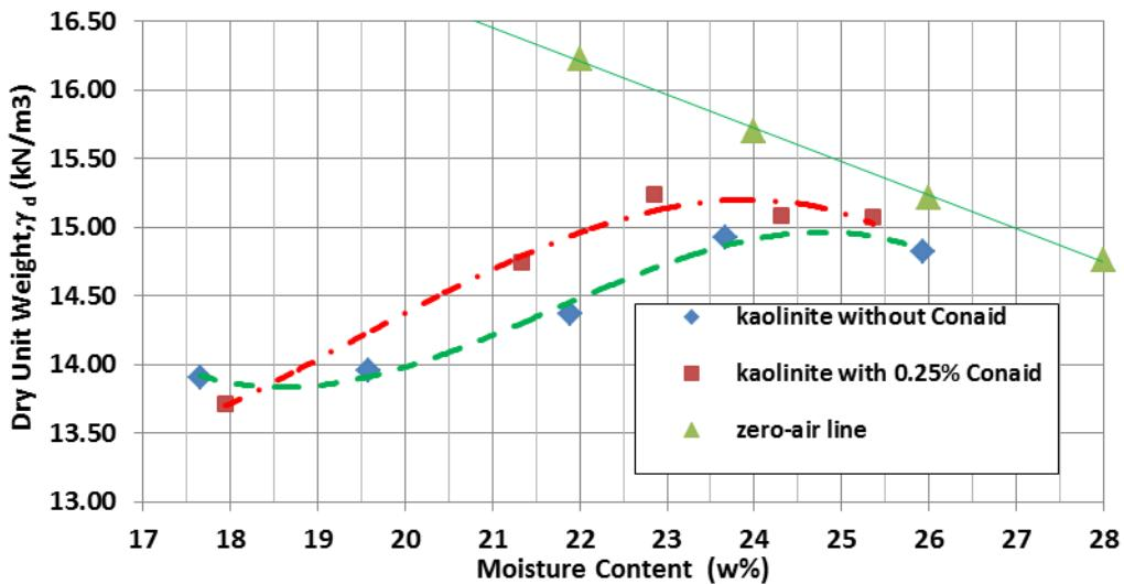
Figure 4.3 Compaction curve of kaolinite passing No. 8 sieve
