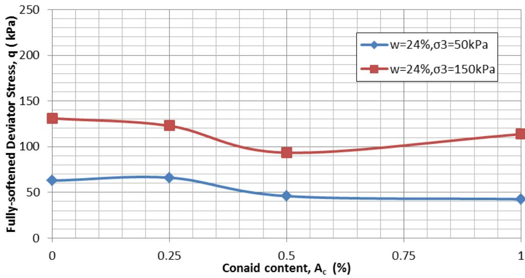
Figure 5.3 Fully-softened deviator stress vs. Conaid content for CD tests at confining pressures of 50kPa and 150kPa
