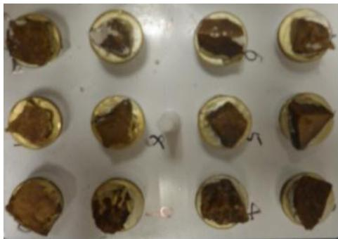
Figure 6.1 SEM samples glued on stubs and coated with gold coating
