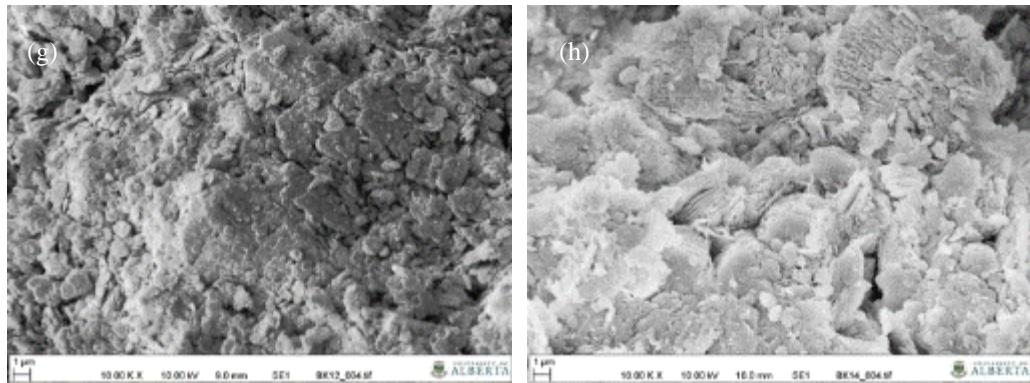
Figure G.7 Photomicrographs of BK20 in unconfined compression test at  $w=28\%$ ,  $T_c=7$  days,
