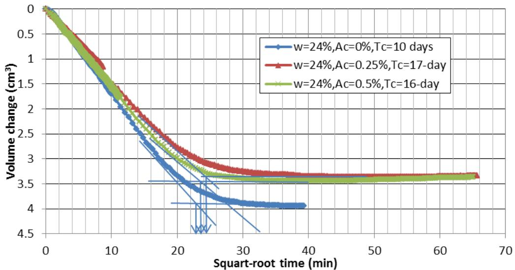
Figure 5.8 Volume change vs. time for  $w=24\%$  &  $p_0'=150\text{kPa}$
