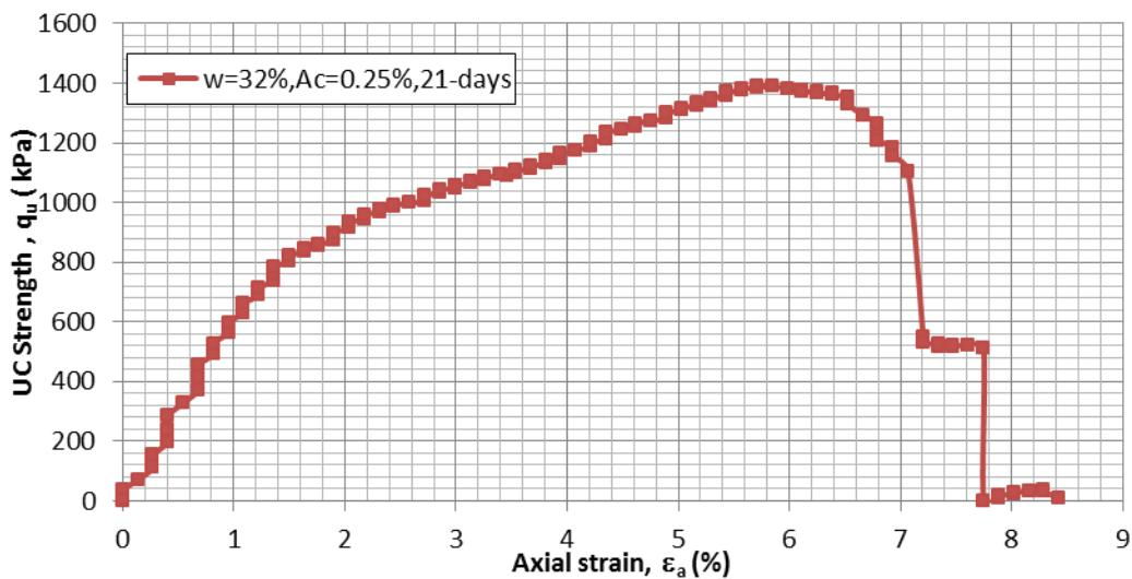
Figure C.9  $q$  vs.  $\epsilon_a$  for  $A_c=0.25\%$ ,  $w=32\%$ , 21-day moisture room dry, sample-1
