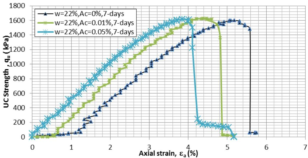
Figure 5.16 UC stress-strain curves for moisture room dry,  $T_c=7$  days
