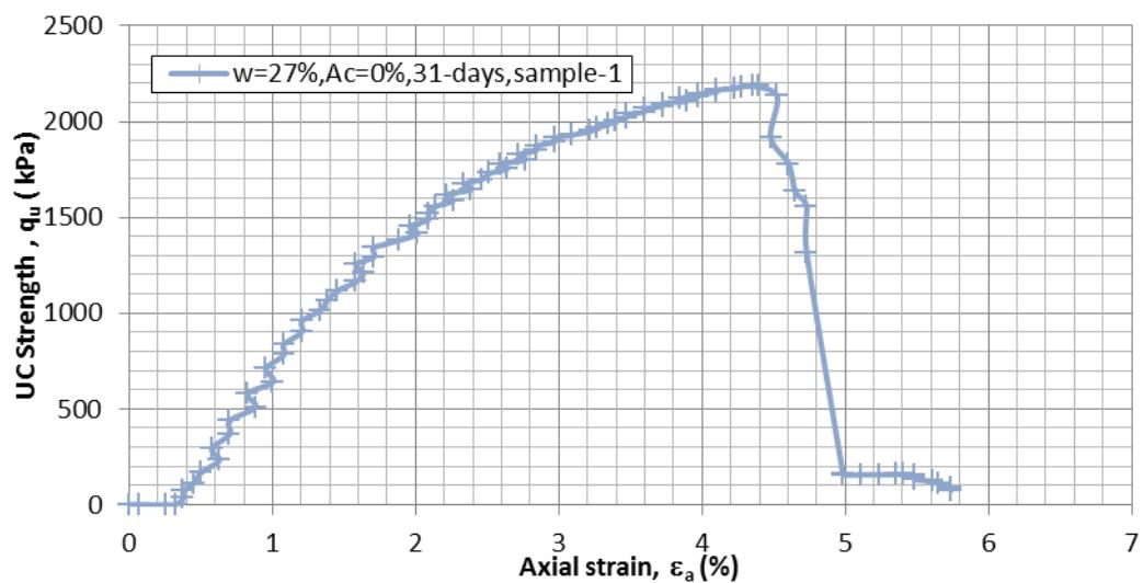
Figure C.17  $q$  vs.  $\epsilon_a$  for  $A_c=0\%$ ,  $w=27\%$ , 31-day moisture room dry, sample-1
