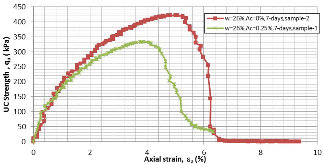
Figure 5.24 UC stress-strain curves for moisture room curing,  $T_c=7$  days
