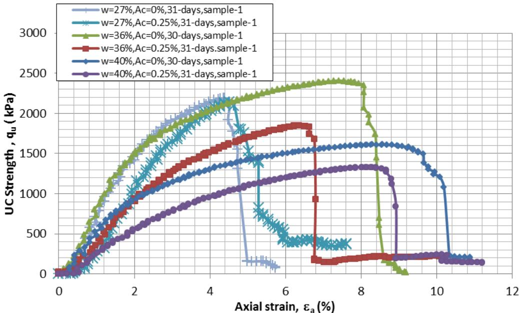
Figure 5.22 UC stress- strain curve for  $Ac=0$  &  $0.25\%$ ,  $T_c=31$  days
