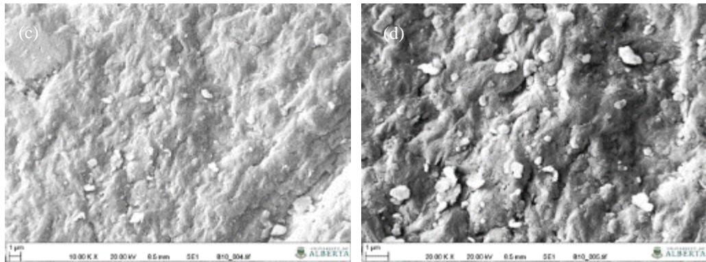
Figure G.6 Photomicrographs of bentonite in unconfined compression test at  $w=32\%$ ,  $T_c=21$  days, (a)  $A_c=0.025\%$ ,  $M\sim 500X$ ; (b)  $A_c=0.025\%$ ,  $M\sim 5,000X$ ; (c)  $A_c=0.025\%$ ,  $M\sim 10,000X$ ; (d)  $A_c=0.025\%$ ,  $M\sim 20,000X$ .
