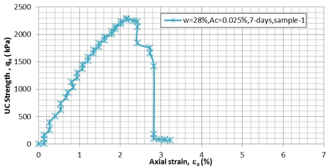
Figure D.13  $q$  vs.  $\varepsilon_a$  for  $A_c=0.025\%$ ,  $w=28\%$ , 7-day air dry, sample-1
