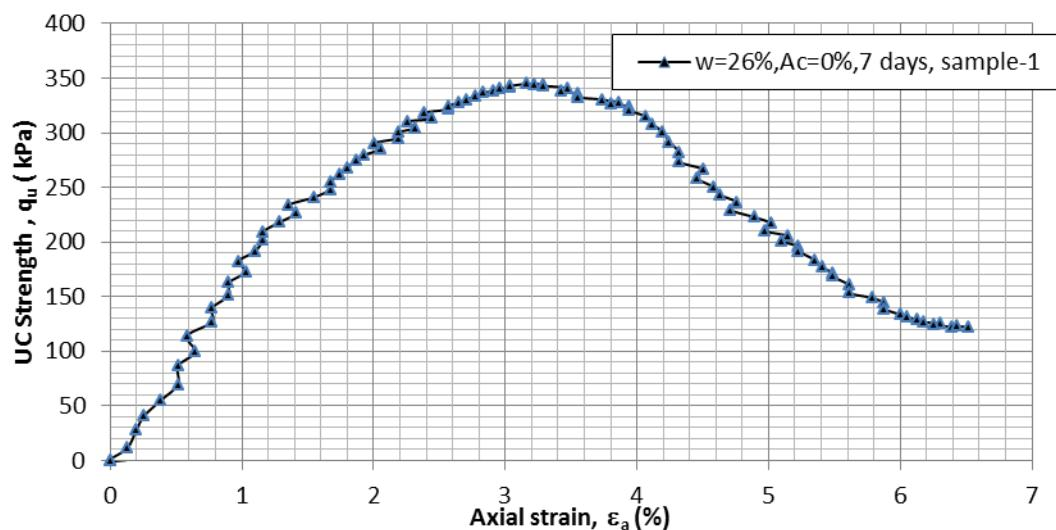
Figure D.5  $q$  vs.  $\epsilon_a$  for  $A_c=0\%$ ,  $w=26\%$ , 7-day moisture room dry, sample-1
