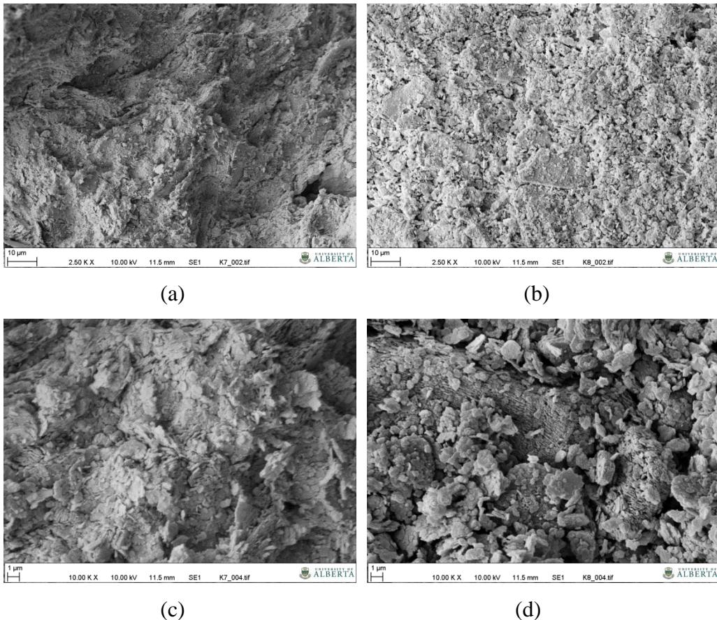
Figure 6.3 Photomicrographs of kaolinite at  $w=24\%$ ,  $T_c=7$  days (a)  $M\sim 2,500X$ ,  $A_c=0\%$ ; (b)  $M\sim 2,500X$ ,  $A_c=0.25\%$ ; (c)  $M\sim 10,000X$ ,  $A_c=0\%$ ; (d)  $M\sim 10,000X$ ,  $A_c=0.25\%$
