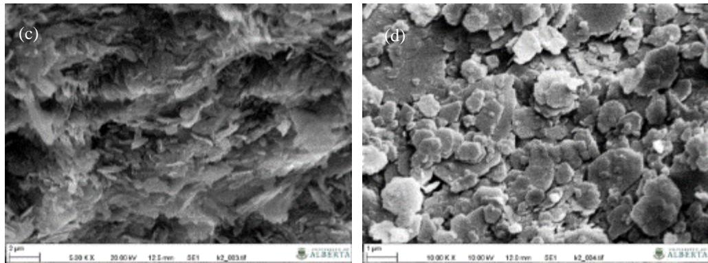
Figure G.2 Photomicrographs of kaolinite in drained triaxial test at  $w=24\%$ ,  $A_c=0.25\%$ ,  $T_c=16$  days, (a)  $M\sim 500X$ ; (b)  $M\sim 2,500X$ ; (c)  $M\sim 5,000X$ ; (d)  $M\sim 10,000X$ .
