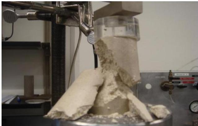
Figure D.8 Photo after UC test for sample-2:  $A_c=0\%$ ,  $w=26\%$ , 7-day moisture room dry
