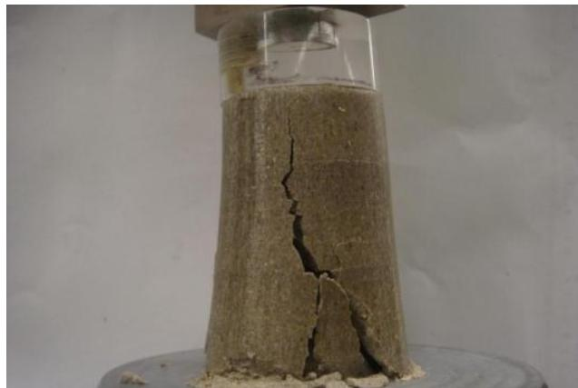
Figure C.16 Photo after UC test for sample-1:  $A_c=0.25\%$ ,  $w=27\%$ , 31-day moisture room dry
