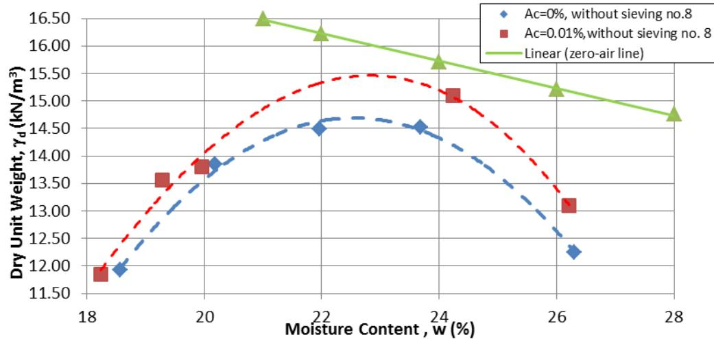
Figure 4.2 Compaction curve of kaolinite without passing No. 8 sieve
