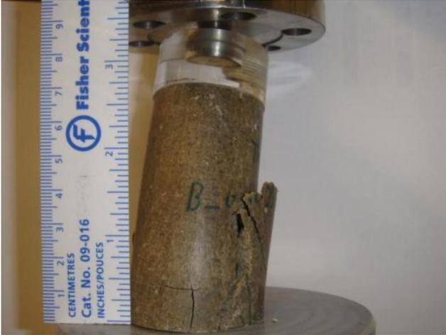
Figure C.8 Photo after UC test for sample-2:  $A_c=0.025\%$ ,  $w=32\%$ , 21-day moisture room dry
