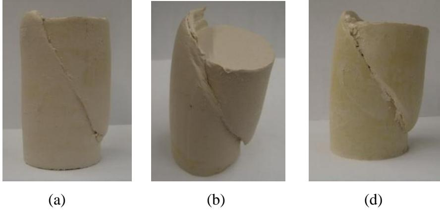
Figure 5.14: Photos of specimens after CD test: (a)  $A_c=0\%$ ,  $w=24\%$ ,  $p_0'=150\text{kPa}$ ; (b)  $A_c=0.25\%$ ,  $w=24\%$ ,  $p_0'=150\text{kPa}$ ; (c)  $A_c=0.5\%$ ,  $w=24\%$ ,  $p_0'=150\text{kPa}$ .
