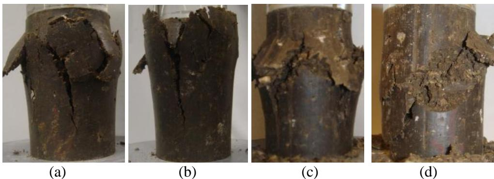
Figure 5.32: Photos of specimens after UC test: (a)  $A_c=0\%$ ,  $w=17\%$ , 0-day; (b)  $A_c=0.025\%$ ,  $w=17\%$ , 0-day; (c)  $A_c=0\%$ ,  $w=17\%$ , 5-day moisture room dry; (d)  $A_c=0.025\%$ ,  $w=17\%$ , 5-day
