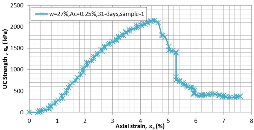
Figure C.15  $q$  vs.  $\epsilon_a$  for  $A_c=0.25\%$ ,  $w=27\%$ , 31-day moisture room dry, sample-1
