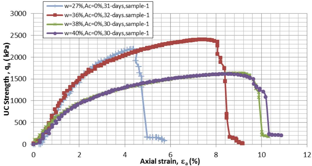
Figure 5.20 UC stress- strain curve for  $Ac=0\%$ ,  $T_c=30\text{--}32$  days
