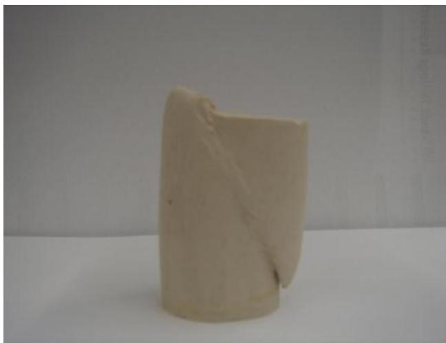
Figure A.15 Photo after CD test for Sample:  $A_c=0.5\%$ ,  $w=24\%$ , 16-day &  $p_0'=50$ kPa
