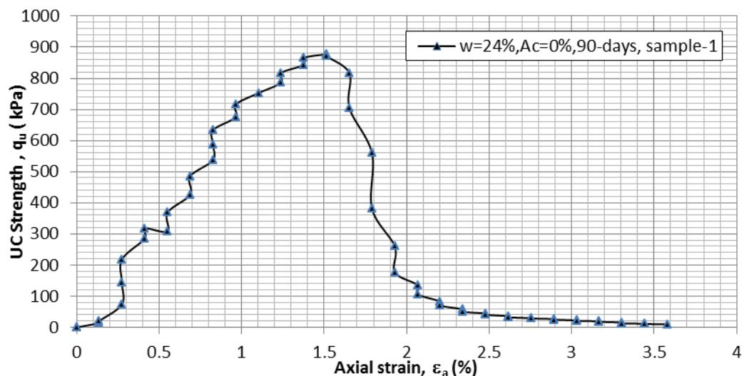
Figure D.21  $q$  vs.  $\varepsilon_a$  for  $A_c=0\%$ ,  $w=24\%$ , 90-day air dry, sample-1
