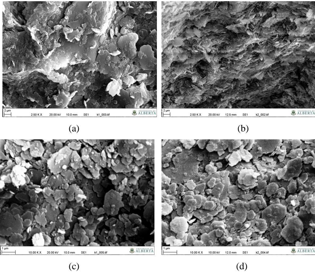
Figure 6.2 Photomicrographs of kaolinite at  $w=24\%$ , (a)  $M \sim 2,500X$ ,  $A_c=0\%$ ,  $T_c=10$  days; (b)  $M \sim 2,500X$ ,  $A_c=0.25\%$ ,  $T_c=17$  days; (c)  $M \sim 10, 000X$ ,  $A_c=0\%$ ,  $T_c=10$  days; (d)  $M \sim 10, 000X$ ,  $A_c=0.25\%$ ,  $T_c=17$  days.
