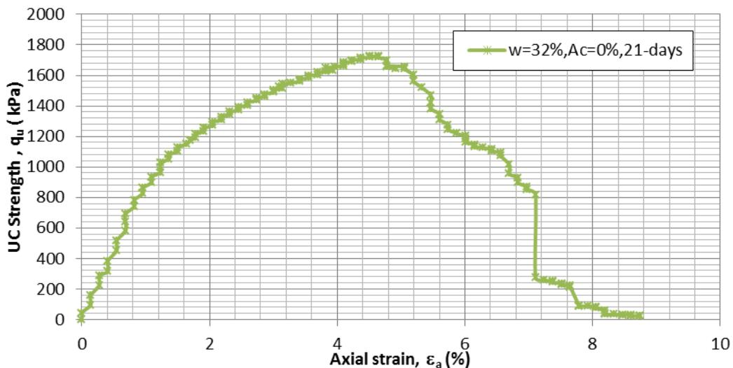
Figure C.1  $q$  vs.  $\epsilon_a$  for  $A_c=0\%$ ,  $w=32\%$ , 21-day moisture room dry, sample-1
