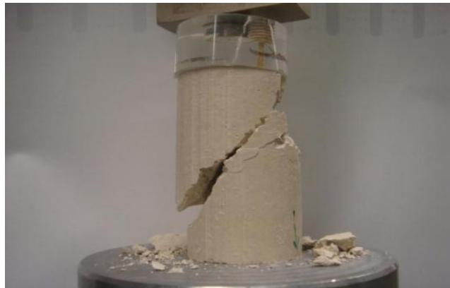
Figure B.14 Photo after UC test for sample-1:  $A_c=0.05\%$ ,  $w=22\%$ , 7-day moisture room dry
