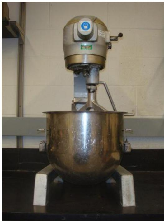
Figure 3.1 Electrical mixer used in soil mixing
