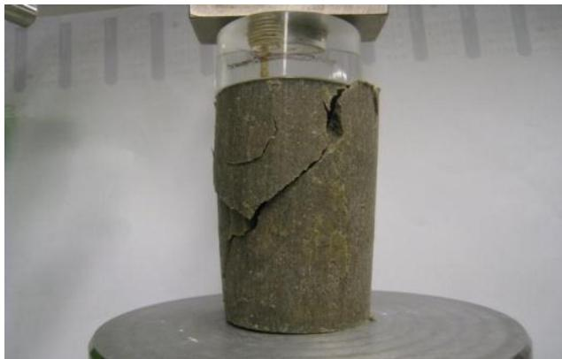
Figure C.20 Photo after UC test for sample-1:  $A_c=0\%$ ,  $w=36\%$ , 31-day moisture room dry
