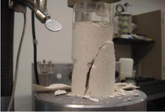
Figure D.20 Photo after UC test for sample-2:  $A_c=0.25\%$ ,  $w=28\%$ , 7-day air dry
