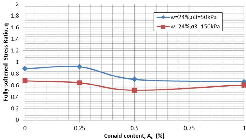
Figure 5.4 Fully-softened deviator stress ratio vs. Conaid content for CD tests at confining pressures of 50kPa and 150kPa
