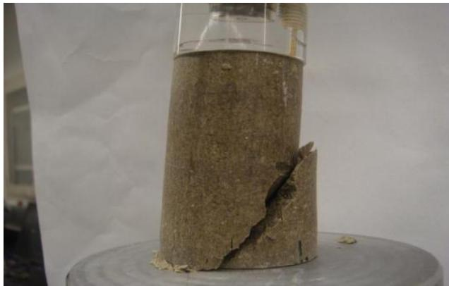
Figure C.14 Photo after UC test for Sample-1:  $A_c=0.25\%$ ,  $w=36\%$ , 31-day moisture room dry
