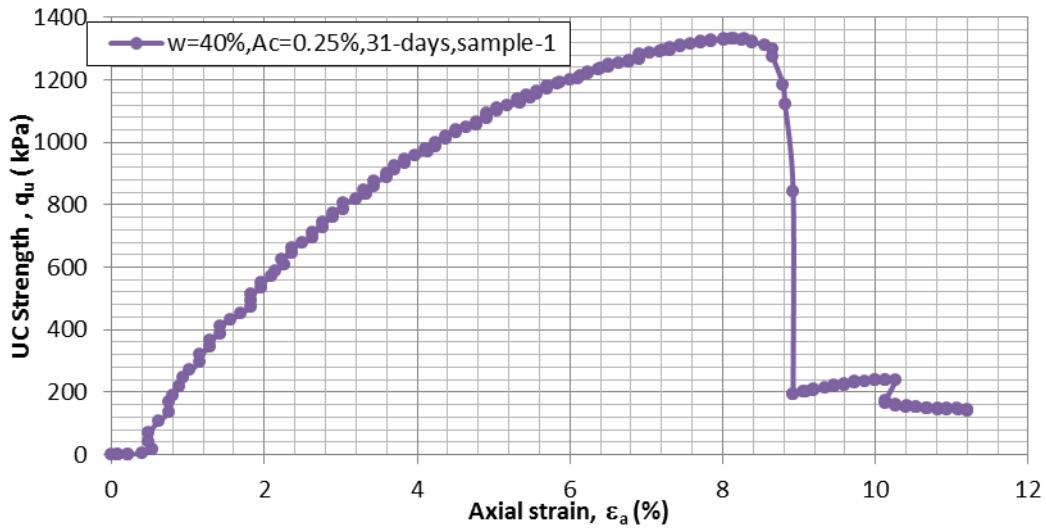
Figure C.11  $q$  vs.  $\epsilon_a$  for  $A_c=0.25\%$ ,  $w=40\%$ , 31-day moisture room dry, sample-1
