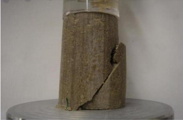
Figure C.12 Photo after UC test for sample-1:  $A_c=0.25\%$ ,  $w=40\%$ , 31-day moisture room dry
