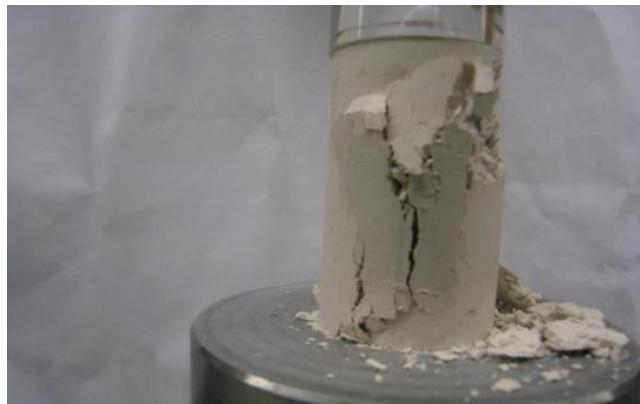
Figure B.4 Photo after UC test for Sample-2:  $A_c=0\%$ ,  $w=24\%$ , 7-day air dry
