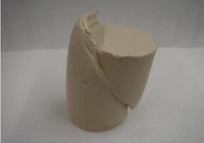
Figure A.8 Photo after CD test for Sample:  $A_c=0.25\%$ ,  $w=24\%$ , 17-day &  $p_0'=150\text{kPa}$
