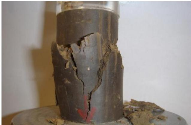
Figure E.2 Photo after UC test for sample-1:  $A_c=0\%$ ,  $w=16.5\%$ , 12-day moisture room dry
