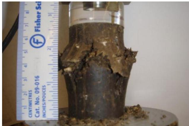
Figure F.2 Photo after UC test for sample-2:  $A_c=0\%$ ,  $w=17\%$ , 5-day moisture room dry
