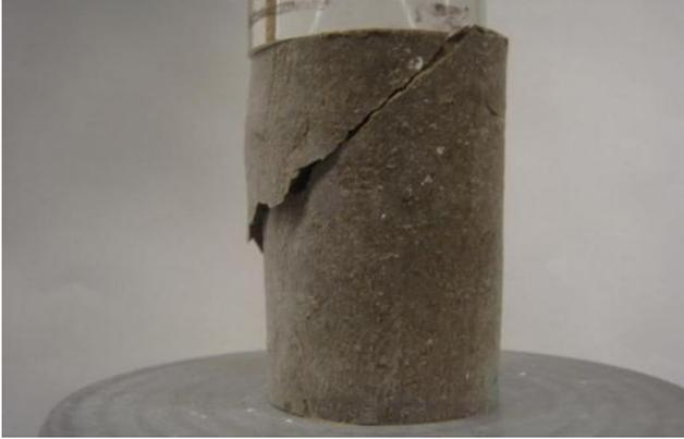
Figure C.22 Photo after UC test for sample-1:  $A_c=0\%$ ,  $w=40\%$ , 31-day moisture room dry
