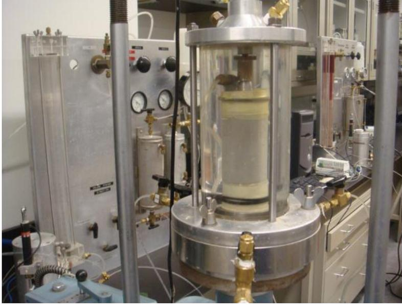
Figure 3.2 Photo of triaxial test apparatus
