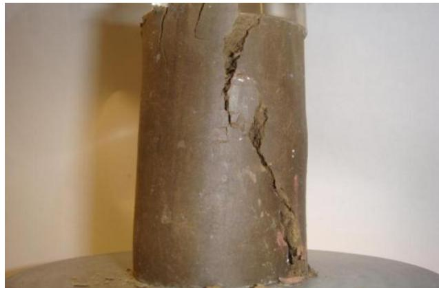
Figure E.10 Photo after UC test for sample-1:  $A_c=0\%$ ,  $w=19\%$ , 21-day moisture room dry
