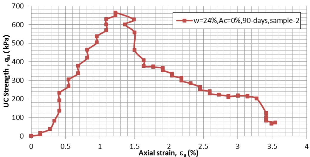
Figure D.23  $q$  vs.  $\varepsilon_a$  for  $A_c=0\%$ ,  $w=24\%$ , 90-day air dry, sample-2
