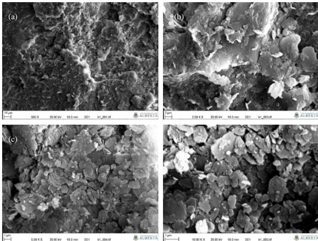
Figure G.1 Photomicrographs of kaolinite in drained triaxial test at  $w=24\%$ ,  $A_c=0\%$ ,  $T_c=10$  days, (a) M~500X; (b) M~2,500X; (c) M~5, 000X; (d) M~10, 000X.
