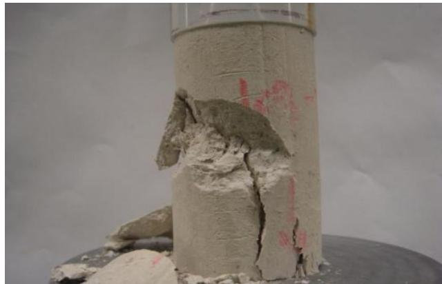
Figure D.16 Photo after UC test for sample-2:  $A_c=0.025\%$ ,  $w=28\%$ , 7-day air dry
