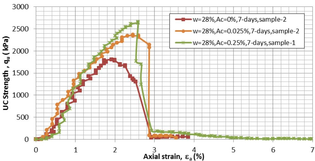
Figure 5.25 UC stress-strain curves for air-dried,  $T_c=7$  days
