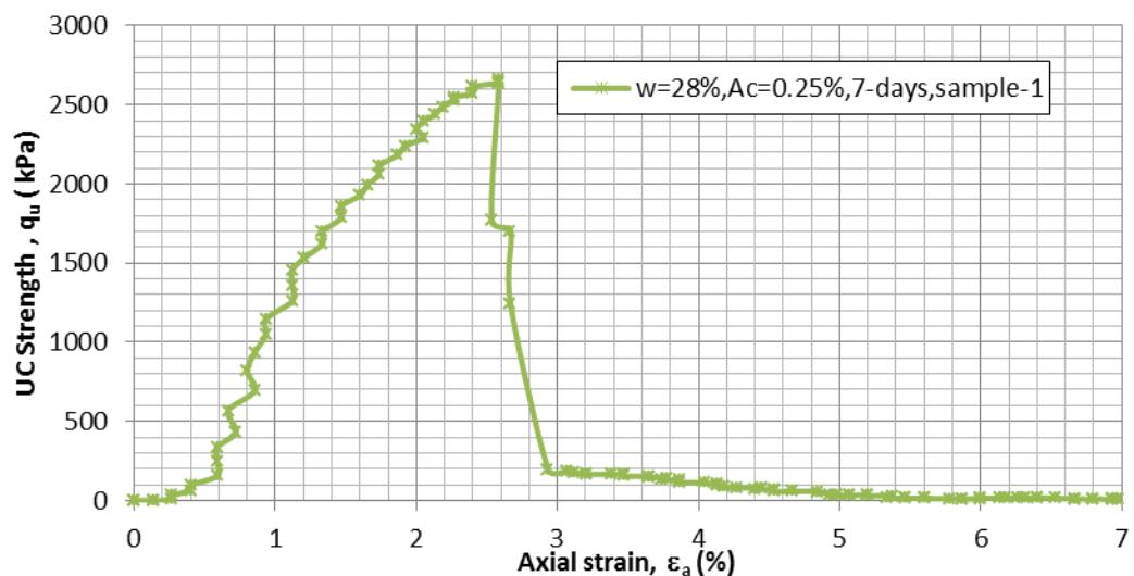
Figure D.17  $q$  vs.  $\varepsilon_a$  for  $A_c=0.25\%$ ,  $w=28\%$ , 7-day air dry, sample-1
