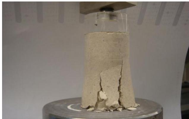
Figure D.2 Photo after UC test for sample-1:  $A_c=0.25\%$ ,  $w=26\%$ , 7-day moisture room dry
