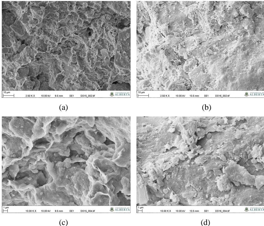
Figure 6.6 Photomicrographs of Devon silt at  $w=16.5\%$ ,  $T_c=12$  days, (a)  $M\sim 2,500X$ ,  $A_c=0\%$ ; (b)  $M\sim 2,500X$ ,  $A_c=0.05\%$ ; (c)  $M\sim 10,000X$ ,  $A_c=0\%$ ; (d)  $M\sim 10,000X$ ,  $A_c=0.05\%$ .
