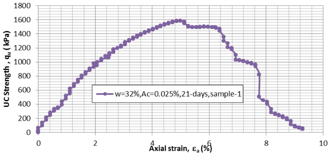
Figure C.5  $q$  vs.  $\epsilon_a$  for  $A_c=0.025\%$ ,  $w=32\%$ , 21-day moisture room dry, sample-1
