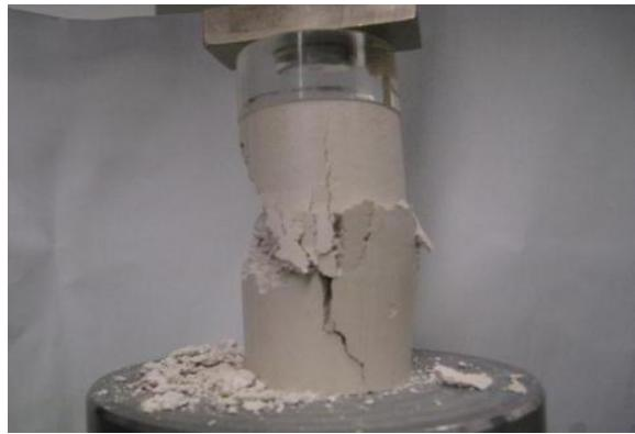
Figure B.2 Photo after UC test for Sample-1:  $A_c=0\%$ ,  $w=24\%$ , 7-day air dry
