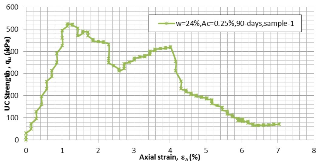
Figure D.25  $q$  vs.  $\varepsilon_a$  for  $A_c=0.25\%$ ,  $w=24\%$ , 90-day air dry, sample-1
