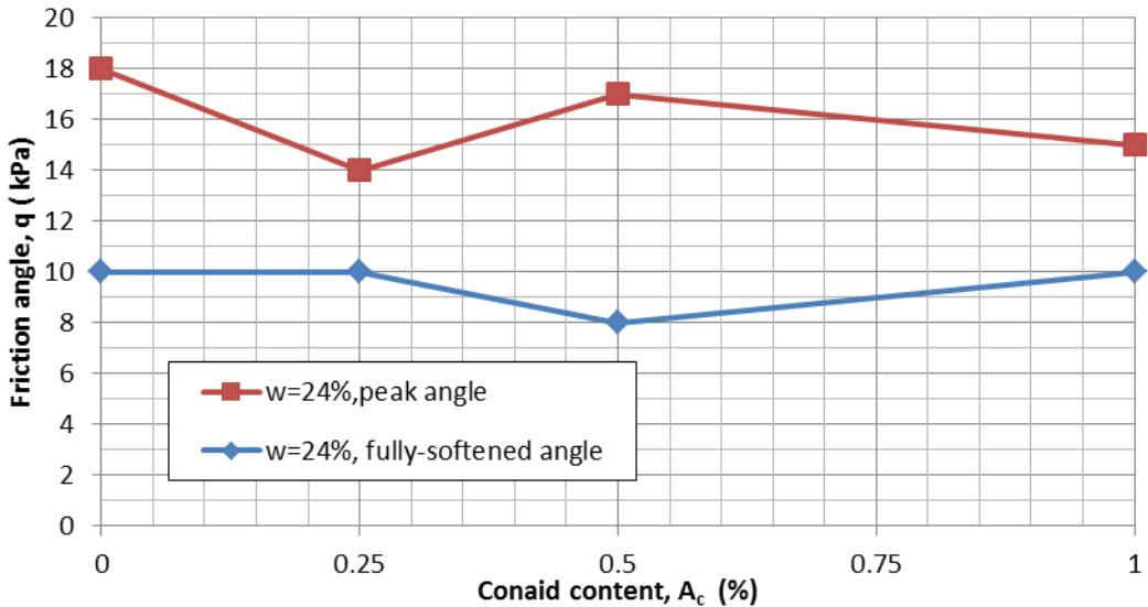
Figure 5.13 Effective friction angles vs. Conaid content
