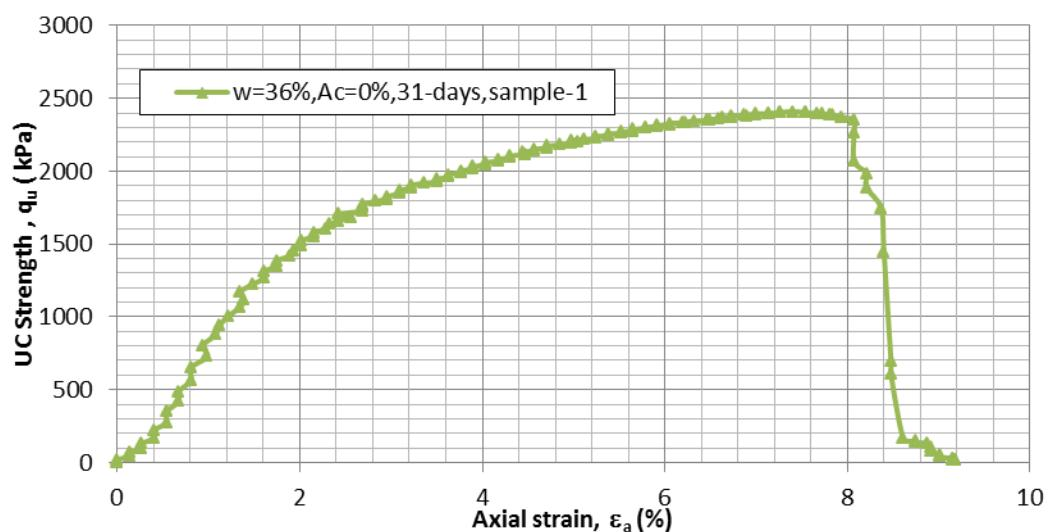
Figure C.19  $q$  vs.  $\epsilon_a$  for  $A_c=0\%$ ,  $w=36\%$ , 31-day moisture room dry, sample-1
