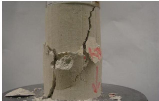
Figure D.14 Photo after UC test for sample-1:  $A_c=0.025\%$ ,  $w=28\%$ , 7-day air dry
