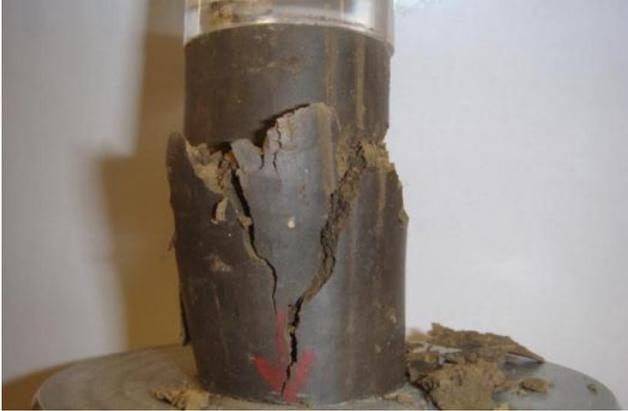
Figure E.2 Photo after UC test for sample-1:  $A_c=0\%$ ,  $w=16.5\%$ , 12-day moisture room dry
