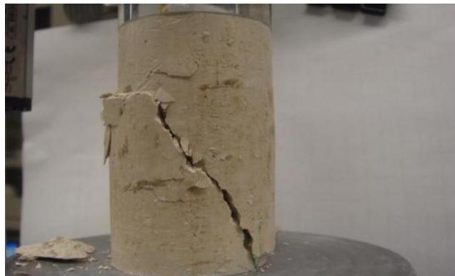
Figure B.10 Photo after UC test for sample-1:  $A_c=0\%$ ,  $w=22\%$ , 7-day moisture room dry
