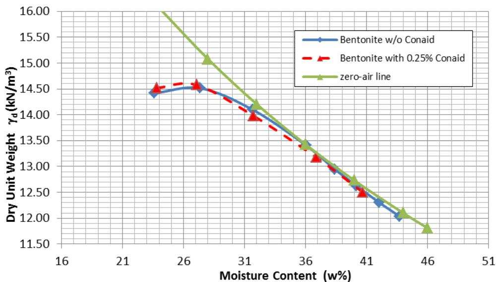
Figure 4.7 Modified Proctor compaction curves for bentonite
