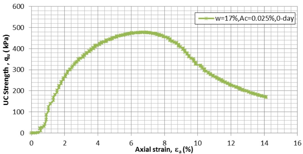
Figure F.7  $q$  vs.  $\epsilon_a$  for  $A_c=0.025\%$ ,  $w=17\%$ , 0-day (as-molded), sample-1
