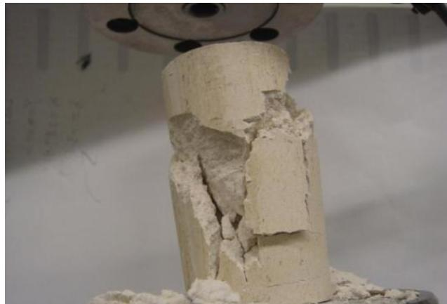
Figure D.22 Photo after UC test for sample-1:  $A_c=0\%$ ,  $w=28\%$ , 90-day air dry
