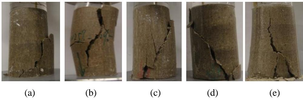
Figure 5.23: Photos of specimens after UC test: (a)  $A_c=0\%$ ,  $w=32\%$ , 21-day moisture room dry; (b)  $A_c=0.025\%$ ,  $w=32\%$ , 21-day moisture room dry; (c)  $A_c=0.25\%$ ,  $w=32\%$ , 21-day moisture room dry; (d)  $A_c=0\%$ ,  $w=27\%$ , 31-day moisture room dry; (e)  $A_c=0.25\%$ ,  $w=27\%$ , 31-day moisture room dry
