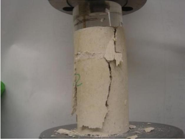
Figure D.28 Photo after UC test for sample-2:  $A_c=0.25\%$ ,  $w=24\%$ , 90-day air dry
