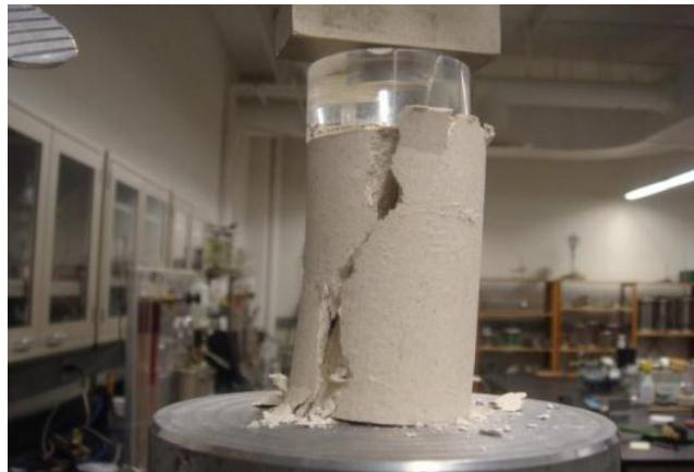
Figure D.18 Photo after UC test for sample-1:  $A_c=0.25\%$ ,  $w=28\%$ , 7-day air dry
