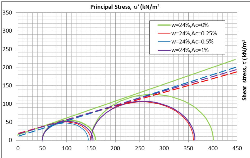
Figure 5.10 Peak envelope of Mohr circles for  $w=24\%$  &  $p_0'=50$  kPa, 150 kPa
