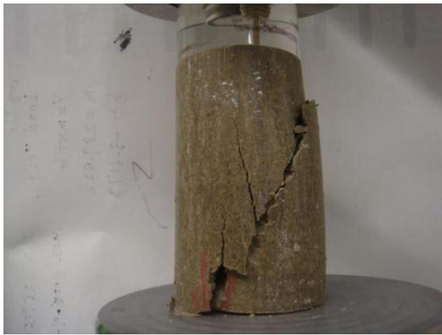
Figure C.10 Photo after UC test for sample-1:  $A_c=0.25\%$ ,  $w=32\%$ , 21-day moisture room dry
