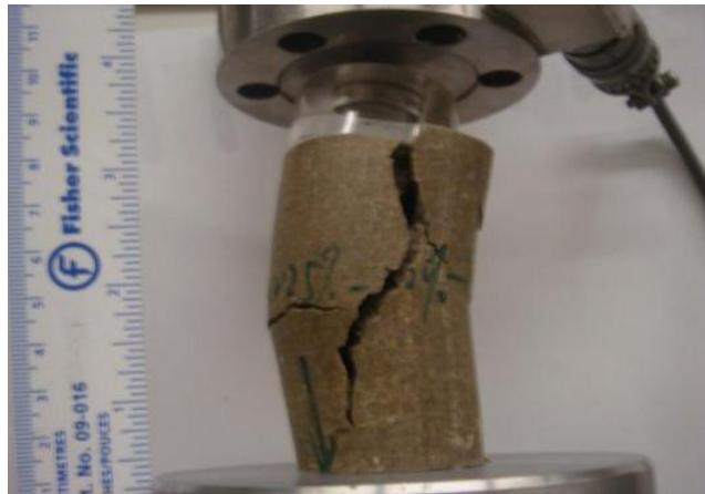
Figure C.6 Photo after UC test for Sample-1:  $A_c=0.025\%$ ,  $w=32\%$ , 21-day moisture room dry
