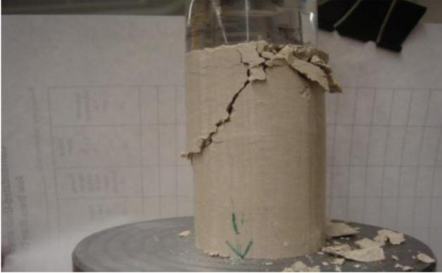
Figure B.12 Photo after UC test for sample-2:  $A_c=0\%$ ,  $w=22\%$ , 7-day moisture room dry
