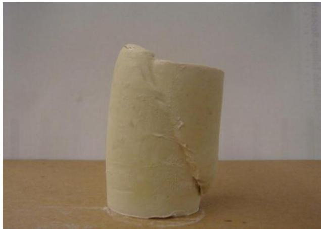
Figure A.19 Photo after CD test for Sample:  $A_c=1\%$ ,  $w=24\%$ , 14-day &  $p_0'=50$ kPa
