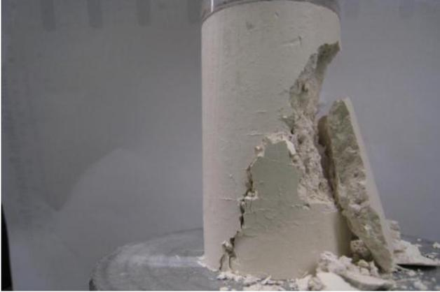
Figure B.6 Photo after UC test for Sample-1:  $A_c=0.25\%$ ,  $w=24\%$ , 7-day air dry
