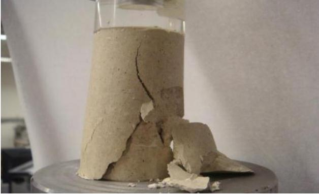
Figure D.6 Photo after UC test for sample-1:  $A_c=0\%$ ,  $w=26\%$ , 7-day moisture room dry
