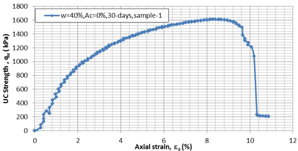
Figure C.21  $q$  vs.  $\epsilon_a$  for  $A_c=0\%$ ,  $w=40\%$ , 31-day moisture room dry, sample-1
