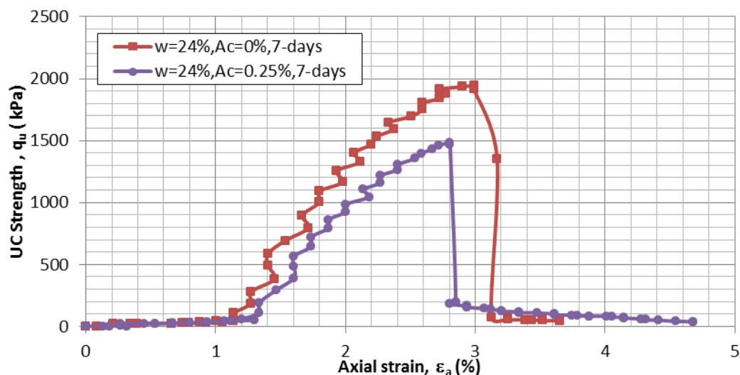
Figure 5.15 UC stress-strain curves for air-dried specimens,  $T_c=7$  days
