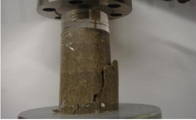
Figure C.2 Photo after UC test for sample-1:  $A_c=0\%$ ,  $w=32\%$ , 21-day moisture room dry
