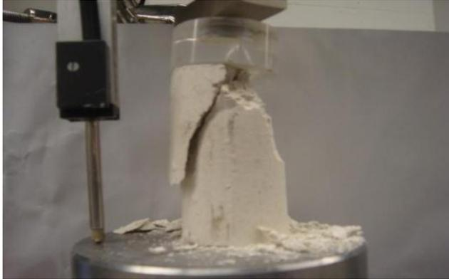
Figure D.10 Photo after UC test for sample-1:  $A_c=0\%$ ,  $w=28\%$ , 7-day air dry
