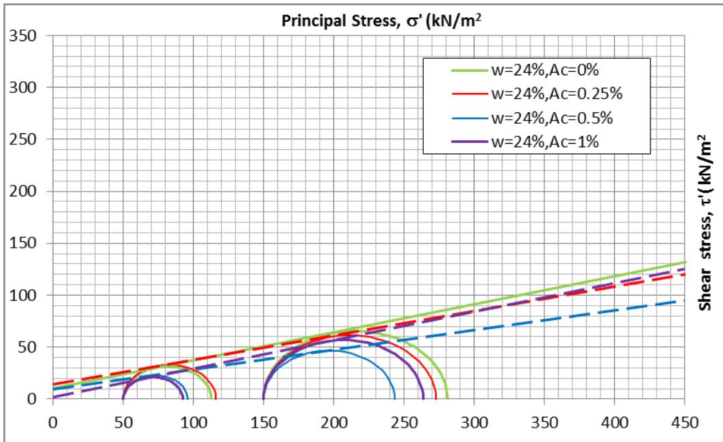
Figure 5.11 Fully-softened envelope of Mohr circles for  $w=24\%$  &  $p_0'=50$ kPa, 150kPa
