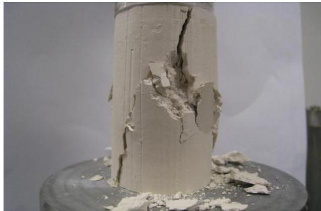
Figure B.8 Photo after UC test for sample-2:  $A_c=0.25\%$ ,  $w=24\%$ , 7-day air dry
