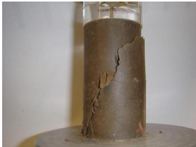
Figure E.14 Photo after UC test for sample-1:  $A_c=0.05\%$ ,  $w=19\%$ , 21-day moisture room dry
