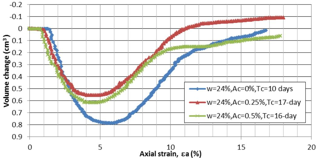
Figure 5.7 Volume change vs.  $\epsilon_a$  for  $w=24\%$  &  $p_0'=150\text{kPa}$
