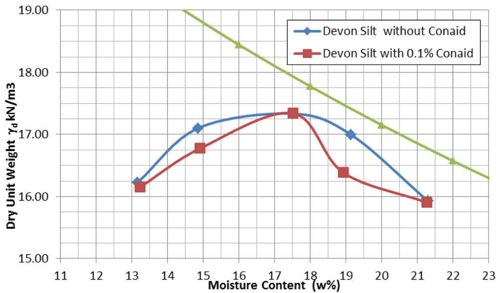
Figure 4.6 Standard Proctor compaction curves for Devon silt
