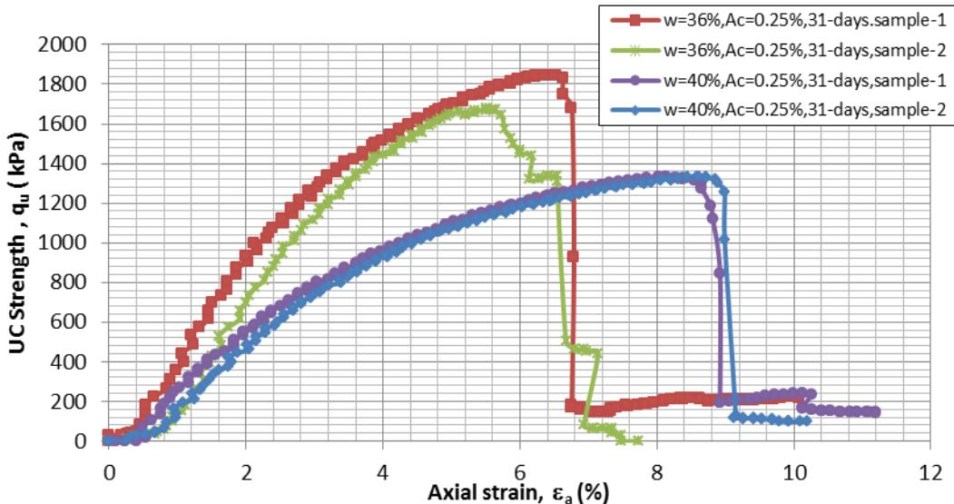
Figure 5.21 UC stress- strain curve for  $Ac=0.25\%$ ,  $T_c=31$  days
