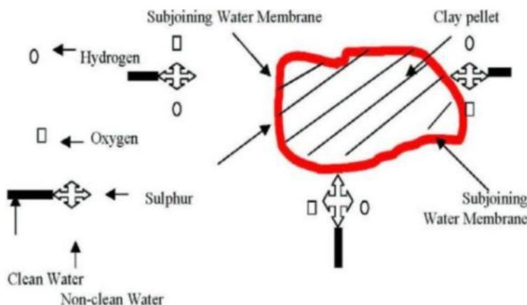
After the ion exchange, clay pellet is surrounded by the sulphonating oil
