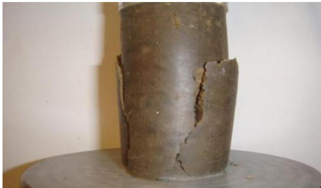
Figure E.6 Photo after UC test for sample-1:  $A_c=0.05\%$ ,  $w=16.5\%$ , 12-day moisture room dry
