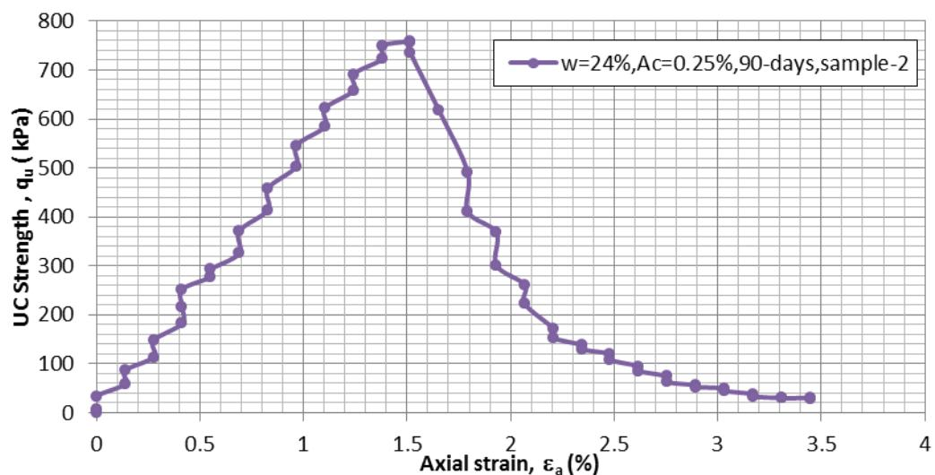
Figure D.27  $q$  vs.  $\epsilon_a$  for  $A_c=0.25\%$ ,  $w=24\%$ , 90-day air dry, sample-2
