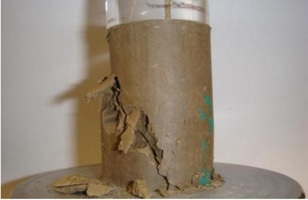
Figure E.12 Photo after UC test for sample-2:  $A_c=0\%$ ,  $w=19\%$ , 21-day moisture room dry
