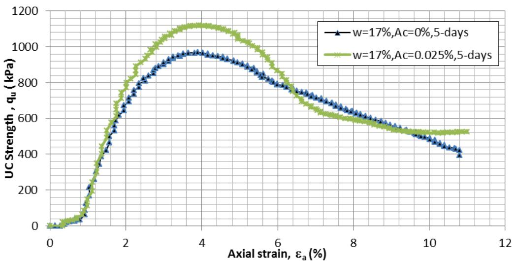
Figure 5.31 UC stress- strain curve for  $w=17\%$ ,  $T_c=5$  days
