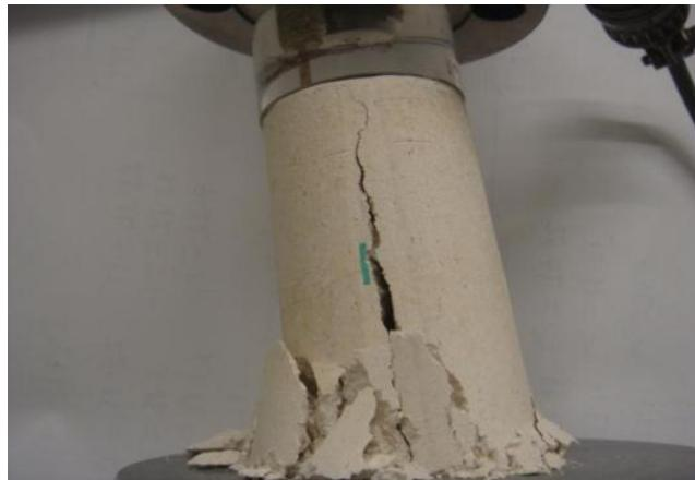
Figure D.26 Photo after UC test for sample-1:  $A_c=0.25\%$ ,  $w=24\%$ , 90-day air dry
