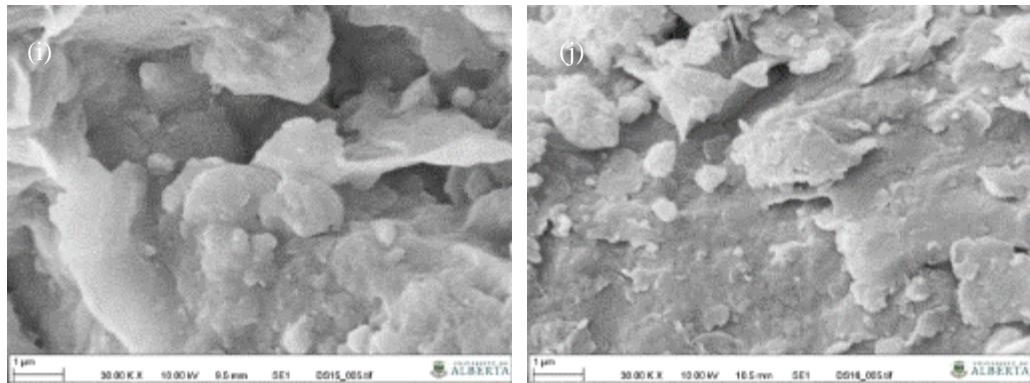
Figure G.9 Photomicrographs of Devon silt in unconfined compression test at  $w=16.5\%$ ,  $T_c=12$  days, (a)  $A_c=0\%$ ,  $M\sim 500X$ ; (b)  $A_c=0.05\%$ ,  $M\sim 500X$ ; (c)  $A_c=0\%$ ,  $M\sim 2,500X$ ; (d)  $A_c=0.05\%$ ,  $M\sim 2,500X$ ; (e)  $A_c=0\%$ ,  $M\sim 5,000X$ ; (f)  $A_c=0.05\%$ ,  $M\sim 5,000X$ ; (g)  $A_c=0\%$ ,  $M\sim 10,000X$ ; (h)  $A_c=0.05\%$ ,  $M\sim 10,000X$ ; (i)  $A_c=0\%$ ,  $M\sim 310,000X$ ; (j)  $A_c=0.05\%$ ,  $M\sim 30,000X$ .
