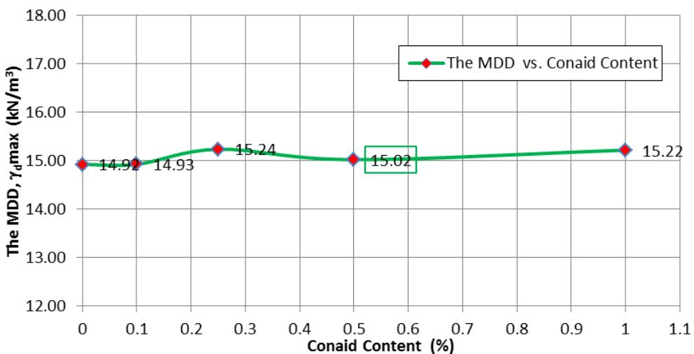
Figure 4.4 Maximum dry unit weight vs. Conaid content
