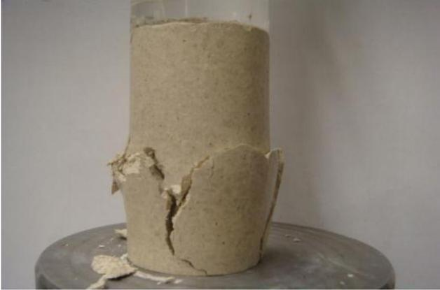
Figure D.4 Photo after UC test for Sample-2:  $A_c=0.25\%$ ,  $w=26\%$ , 7-day moisture room dry
