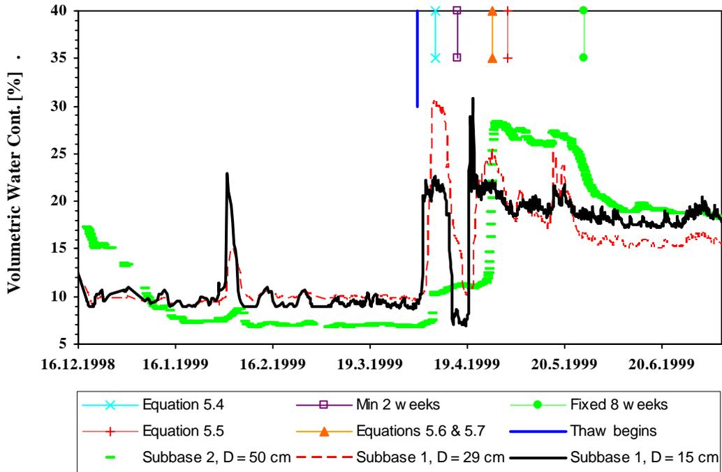
Figure 5- 5: Evaluation of various methods determining onset and removal of axle load limitations, Thingvellir spring 1999.
