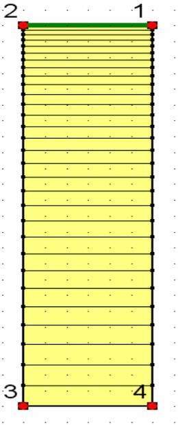
Figure 6- 13: The mesh used in the analysis, the section is 1.5m wide and the height is 6m.
