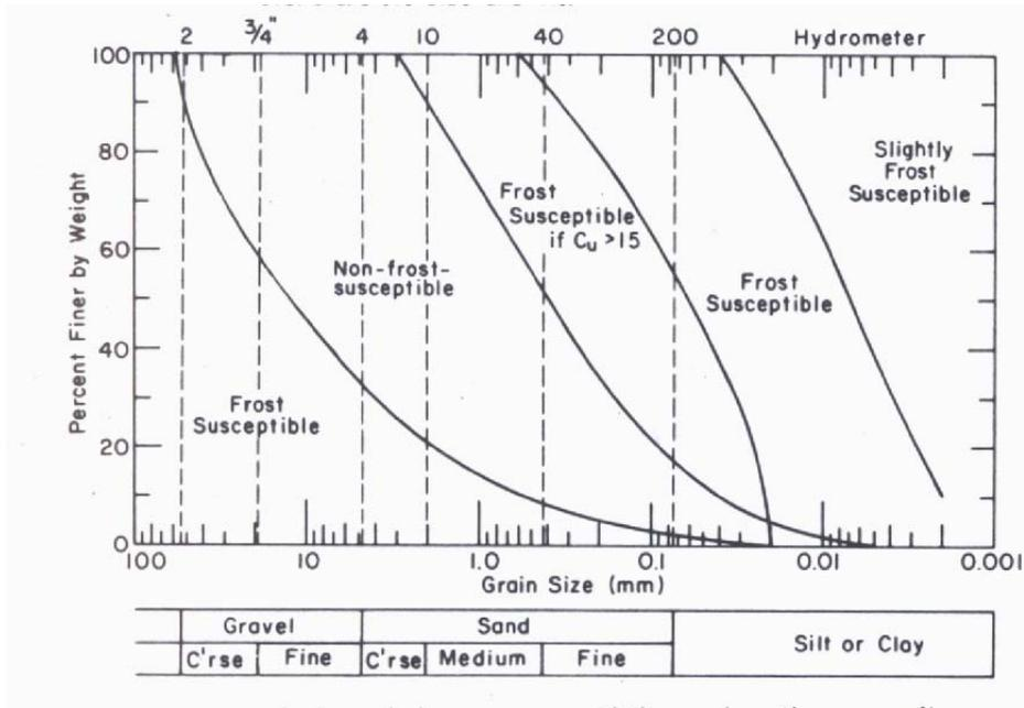
Figure 3-3: Limits of frost susceptibility of soils according to Chamberlain (1981)
