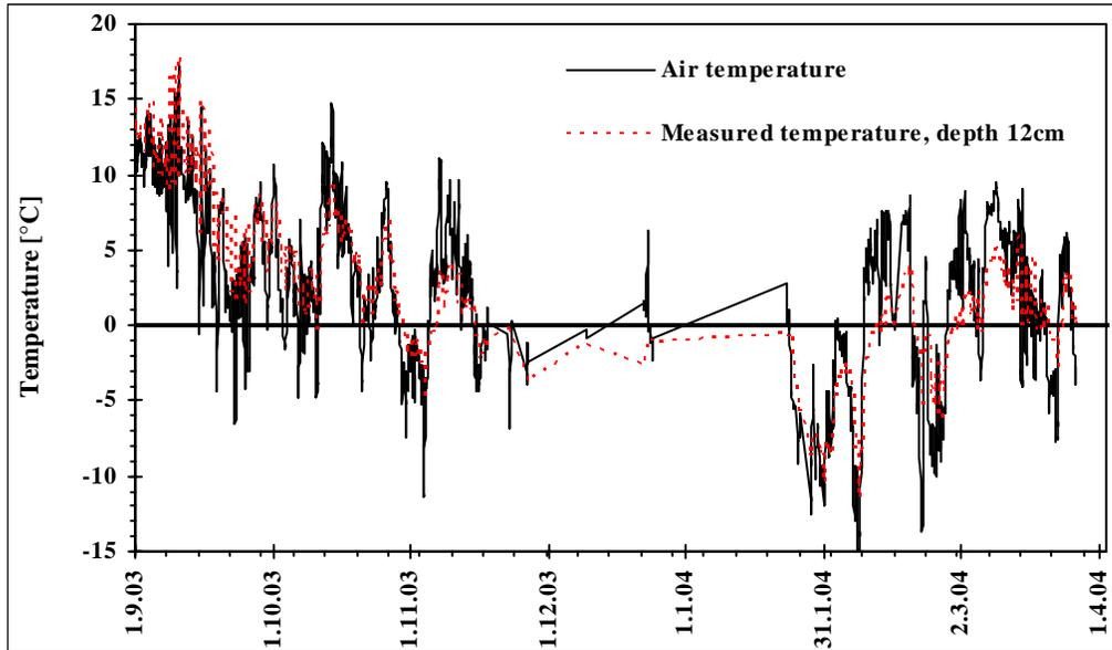
Figure 5- 6: Comparison between air temperature and temperature at 7cm depth in the road section at Vatnskaard 2003-2004.
