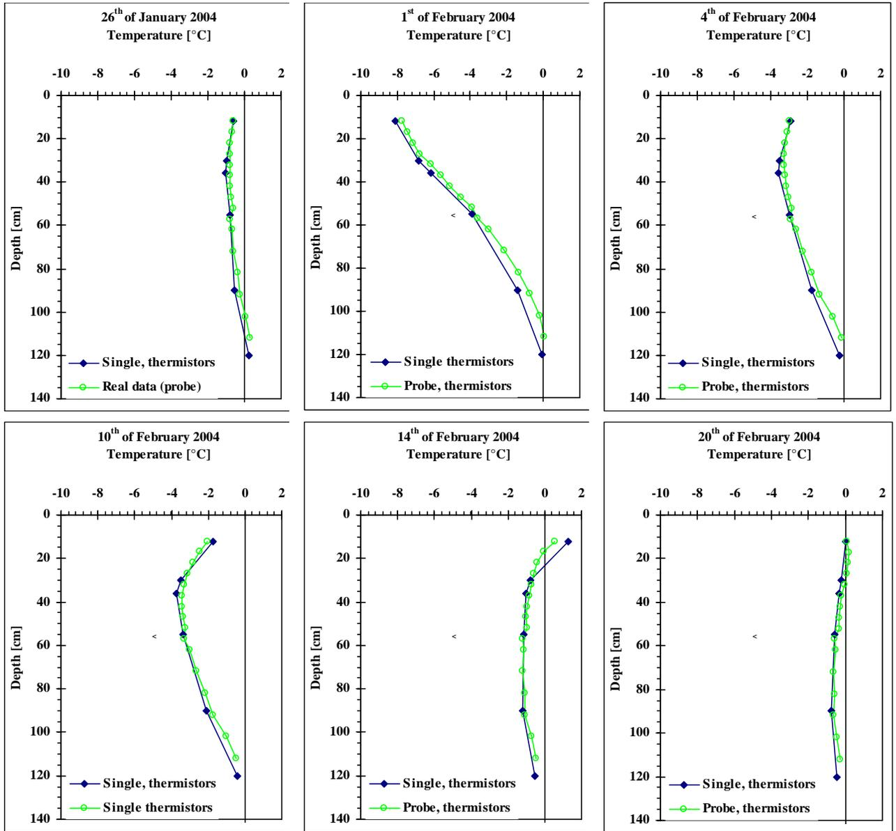
Figure 5- 7: Heat distribution in the road during spring thaw at Dyrastadir January and February 2004
