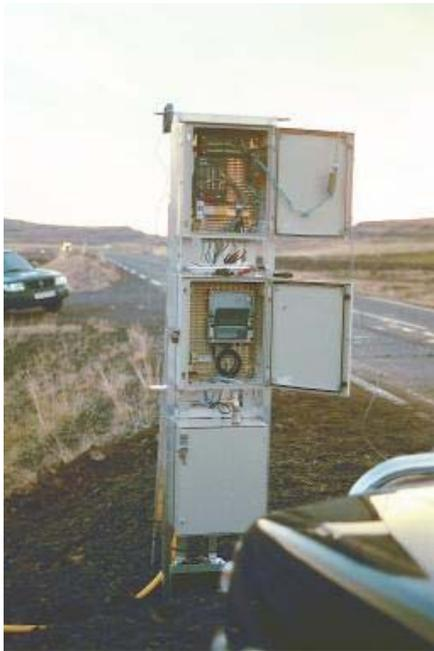
Figure 4- 4: Data logger and transmitting device [Erlingsson 2002a].
