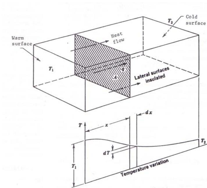
Figure 3-4: Schematic drawing of heat flow after Andersland and Ladanyi (2004).
