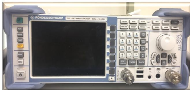
**Figure 4.5: Vector Network analyzer**
