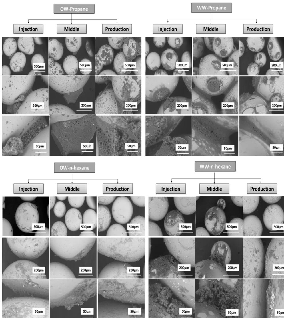
**Figure 5-6: Effect of the glass bead surface on the injection, middle, and production points after the injection of solvents (propane and n-hexane) into two different wet glass surfaces (WW and OW) at 50 °C and 2068 kPa.**
