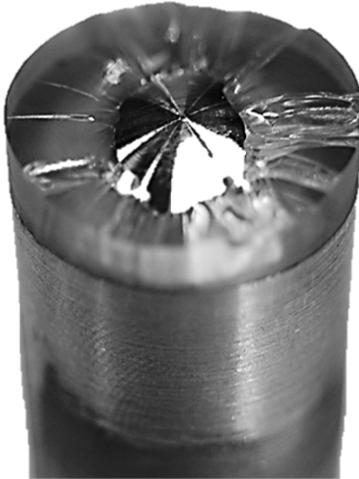
Figure 4.10: Interface of the failed specimen under pure tensile load
