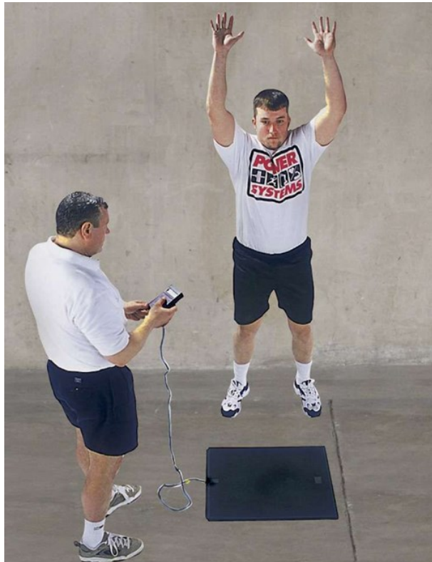
Figure 5 Jump mat (Power Systems, USA) used for vertical jump height estimation (adapted from: https://www.power-systems.com/shop/product/just-jump )
