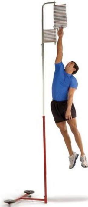
Figure 4 Commercial Vertec (ROGUE Fitness, USA) used for estimation of vertical jump height based on the highest displaced vane (adapted from: https://www.elitefts.com/powermax-vertec-jump-measuring-device.html )
