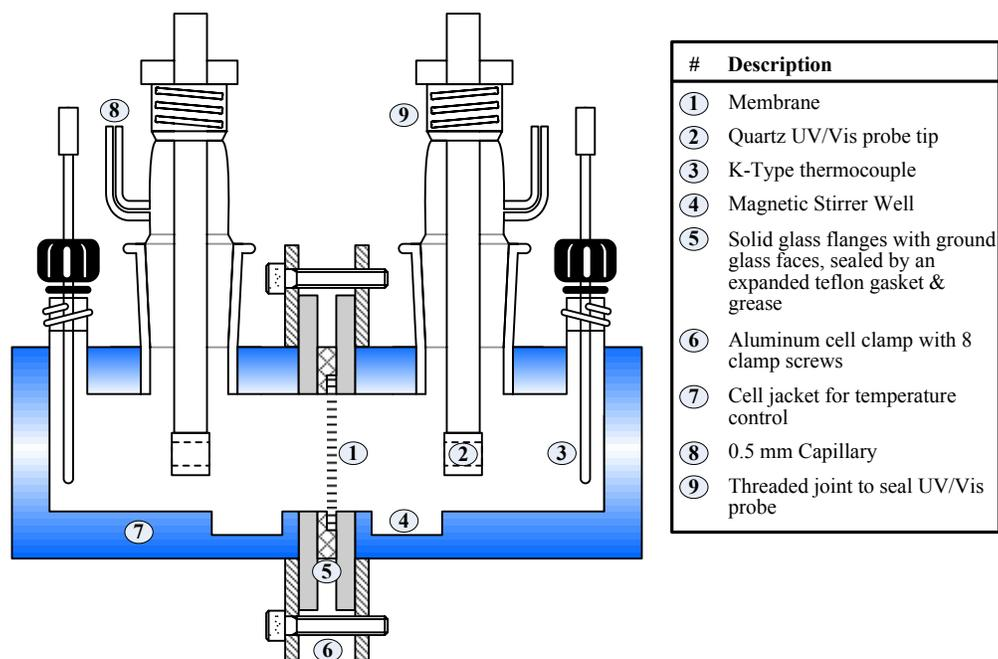
**Figure 4-4:** Schematic diagram of stirred diaphragm diffusion cell
