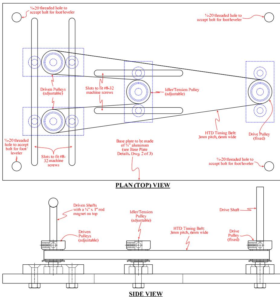
**Figure 4-5:** Detailed drawing of the magnetic stirrer assembly
