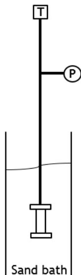
**Figure 3.1.** Batch reactor system used for visbreaking reactions.
