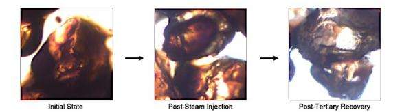
Figure 44—Wettability alteration mechanism presented by switchable solvent on sand grain surface poststeam-chemical-based recovery.
