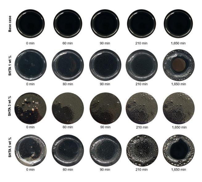
Figure 65—Potential foamy oil recovery mechanisms presented by SHTA at different concentrations collected after core flooding: (a) heavy-oil A and (b) heavy-oil B.
