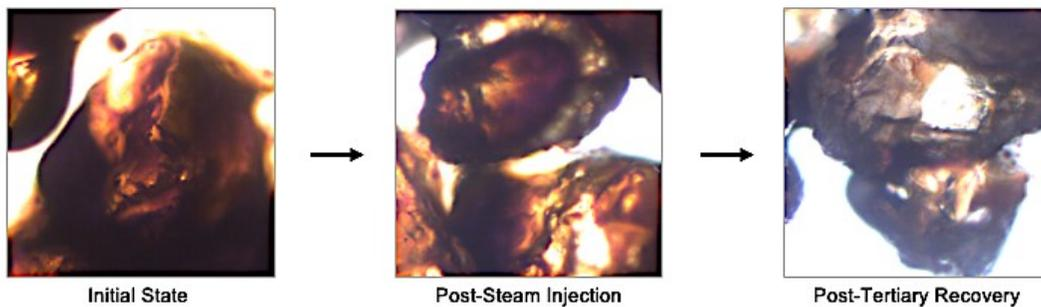
**Figure 44—Wettability alteration mechanism presented by switchable solvent on sand grain surface post-steam-chemical-based recovery.**
