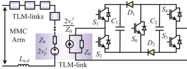
Fig. 7. MMC SM partitioned by TLM-link.
