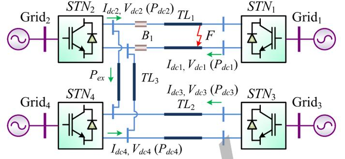
Fig. 8. Four-terminal HVdc grid based on mixed MMC topologies and the UFMCB.
