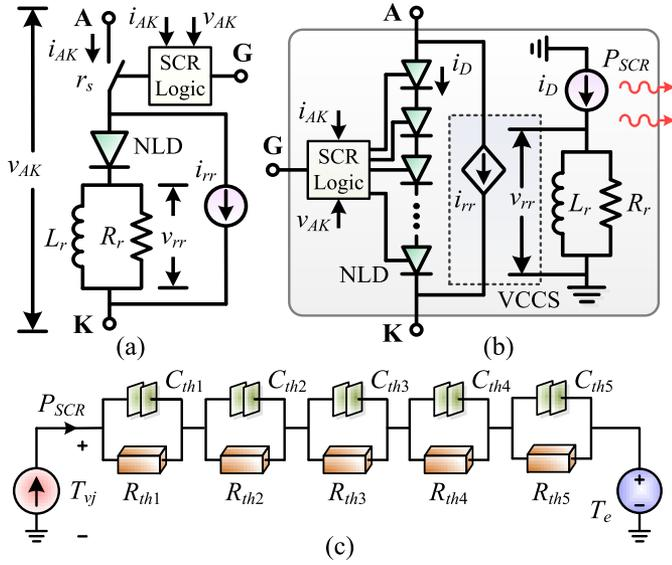
Fig. 1. Nonlinear behavioral thyristor model. (a) Single device. (b) Scalable thyristor model with (c) cascaded  $R$ - $C$  network for thermal impedance.
