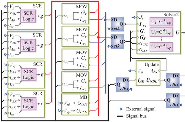
Fig. 9. Synthesized hardware architecture of the UFMCB on the FPGA.
