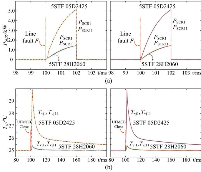
Fig. 13. UFMCB thyristor device-level results during closing from real-time HIL emulation (left) and ANSYS/Simplorer (right). (a) Power loss. (b) Junction temperature.
