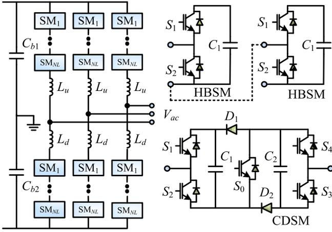
Fig. 6. Three-phase MMC topology and its SM configurations.
