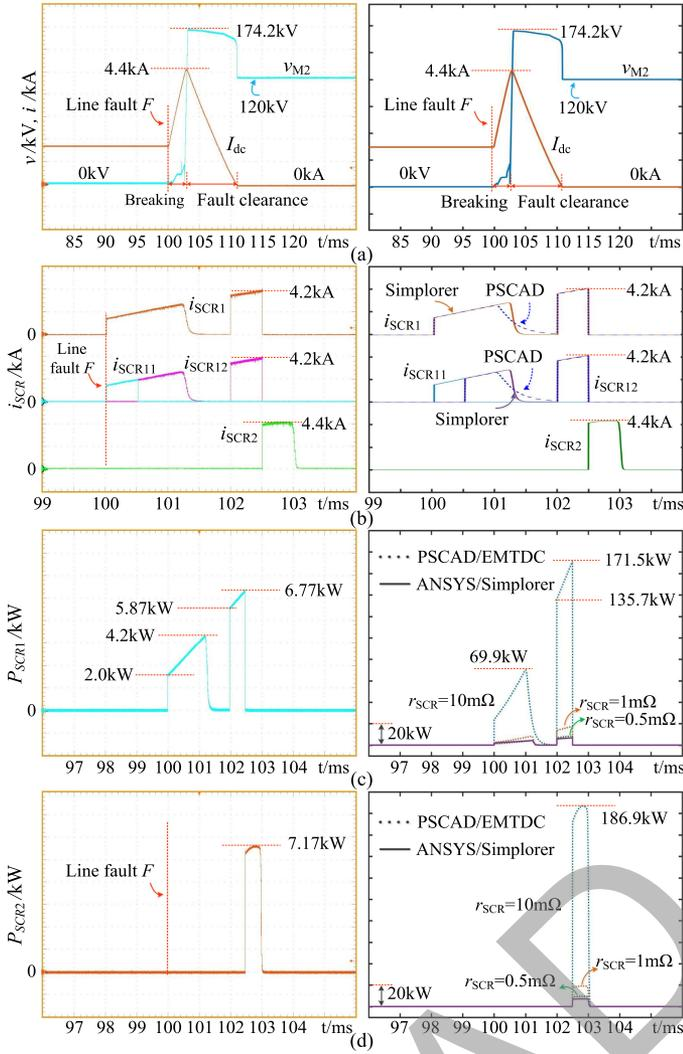
**Fig. 11.** UFMCB real-time emulation oscilloscope results (left) validated by ANSYS/Simplorer and PSCAD/EMTDC (right). (a) Protection waveforms. (b) SCR currents. (c) SCR<sub>1</sub> power consumption. (d) SCR<sub>2</sub> power consumption.
