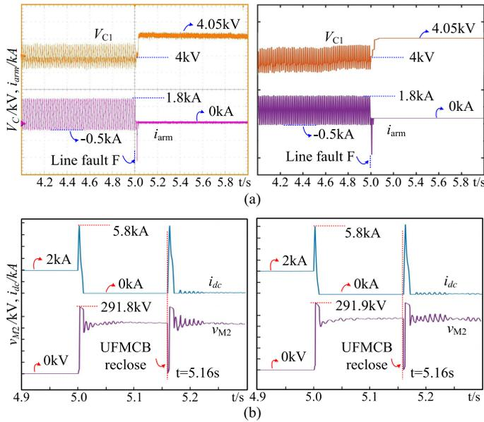
Fig. 16. Real-time HIL emulation results (left) and PSCAD/EMTDC validation (right) of protections initiated by (a) CDSM-MMC and (b) UFMCB with reclosure.
