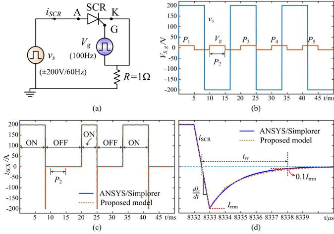
Fig. 2. Thyristor model validation. (a) Test circuit. (b) Source and gate voltages. (c) and (d) Thyristor current.
