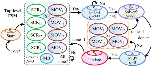
Fig. 10. UFMCB top-level FSM.
