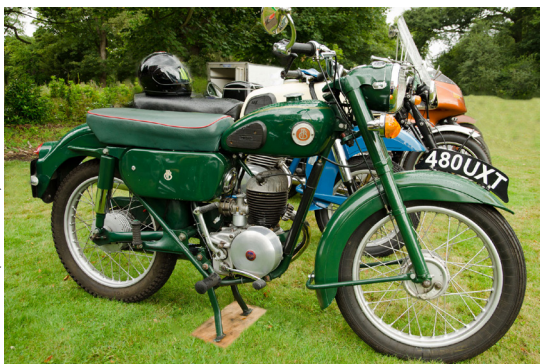
Figure 9. Motorcycle of the type ridden by the author during the 1960s (Francis Barnett Falcon 200 cc 2-stroke).
