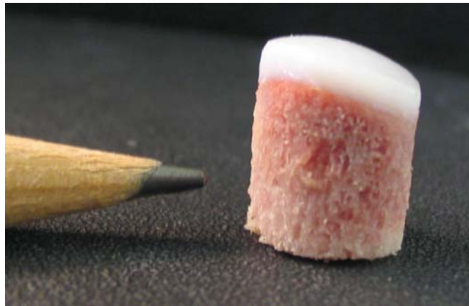
Figure 2-2: A cartilage-bearing bone graft (dowel) sample, excised from the femoral head of the knee joint of a sexually mature pig, Killed for food purposes. The diameter of the dowel is 10 mm and the thickness of cartilage is 2 mm on average.
