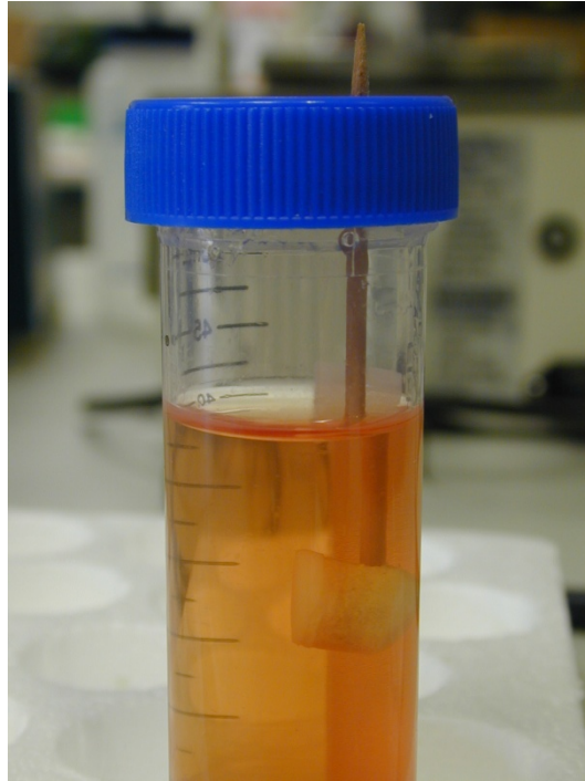
Figure 3-3: A cartilage dowel prepared for the MRI experiment in PBS/media solution. A wooden stick is used to keep the cartilage in place with the face of the cartilage (top surface) perpendicular to the magnetic field B_0 .
