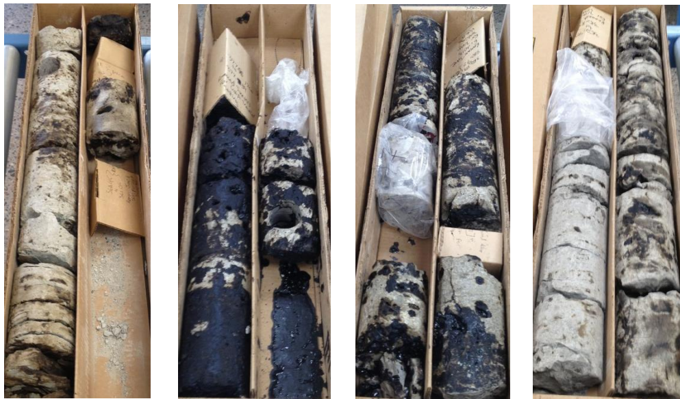
Figure 1.2: Vuggy dolomite core from Grosmont UG2 layer with varying presence of bitumen (photos of Laricina core)
