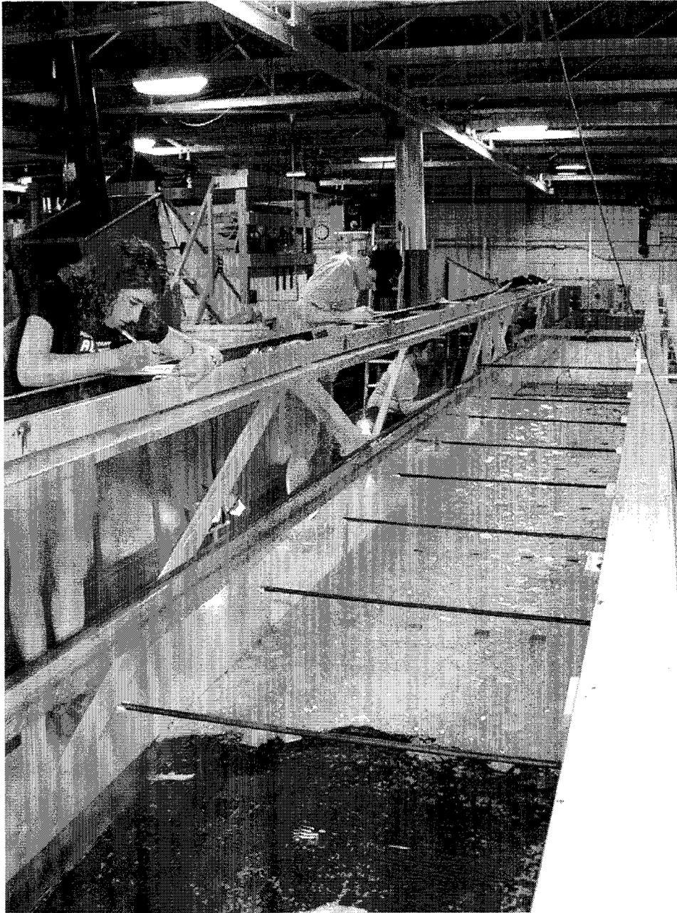
Figure D.1 Manual particle tracking – note transverse markers and tracking particles.
