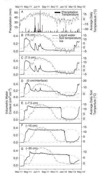
Fig. 4. Water and heat dynamics of 30 cm topsoil treatment during March 2011 to April 2012.
