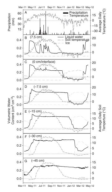
Fig. 3. Water and heat dynamics of 15 cm topsoil treatment during March 2011 to April 2012.
