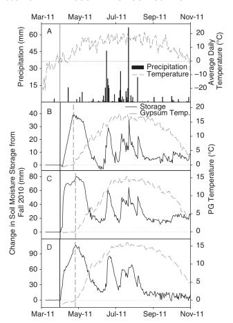
**Fig. 6.** Changes in storage within topsoil cap for the 15- (B), 30- (C) and 46-cm (D) capping soil treatments.
