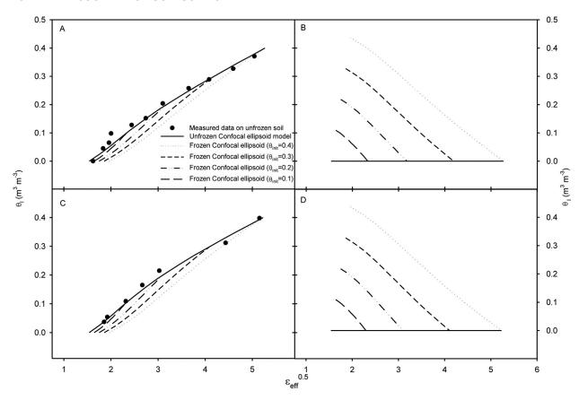
Fig. 2. TDR calibration curves for the estimation of liquid unfrozen water content  $(\theta_i)$  and ice content  $(\theta_i)$  for the topsoil cap (A & B) and the phosphogypsum (C & D).
