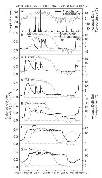
Fig. 5. Water and heat dynamics of 46 cm topsoil treatment during March 2011 to April 2012.
