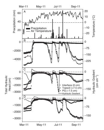
Fig. 7. Total hydraulic head and hydraulic gradient across soil PG interface for the 15- (B), 30- (C) and 46-cm (D) capping soil treatments during March 2011 to November 2011.
