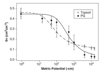
Fig. 1. van Genuchten (1980) model fitted to the moisture retention curves for the topsoil and PG material. van Genuchten parameters are  $\alpha = 0.036 \text{ cm}^{-1}$ , n = 1.57,  $\theta r = 0.11 \text{ cm}^3 \text{ cm}^{-3}$ ,  $\theta s = 0.46 \text{ cm}^3 \text{ cm}^{-3}$  for topsoil, and  $\alpha = 0.0054 \text{ cm}^{-1}$ , n = 1.67,  $\theta r = 0.027 \text{ cm}^3 \text{ cm}^{-3}$ ,  $\theta s = 0.44 \text{ cm}^3$  $cm^{-3}$  for PG.
