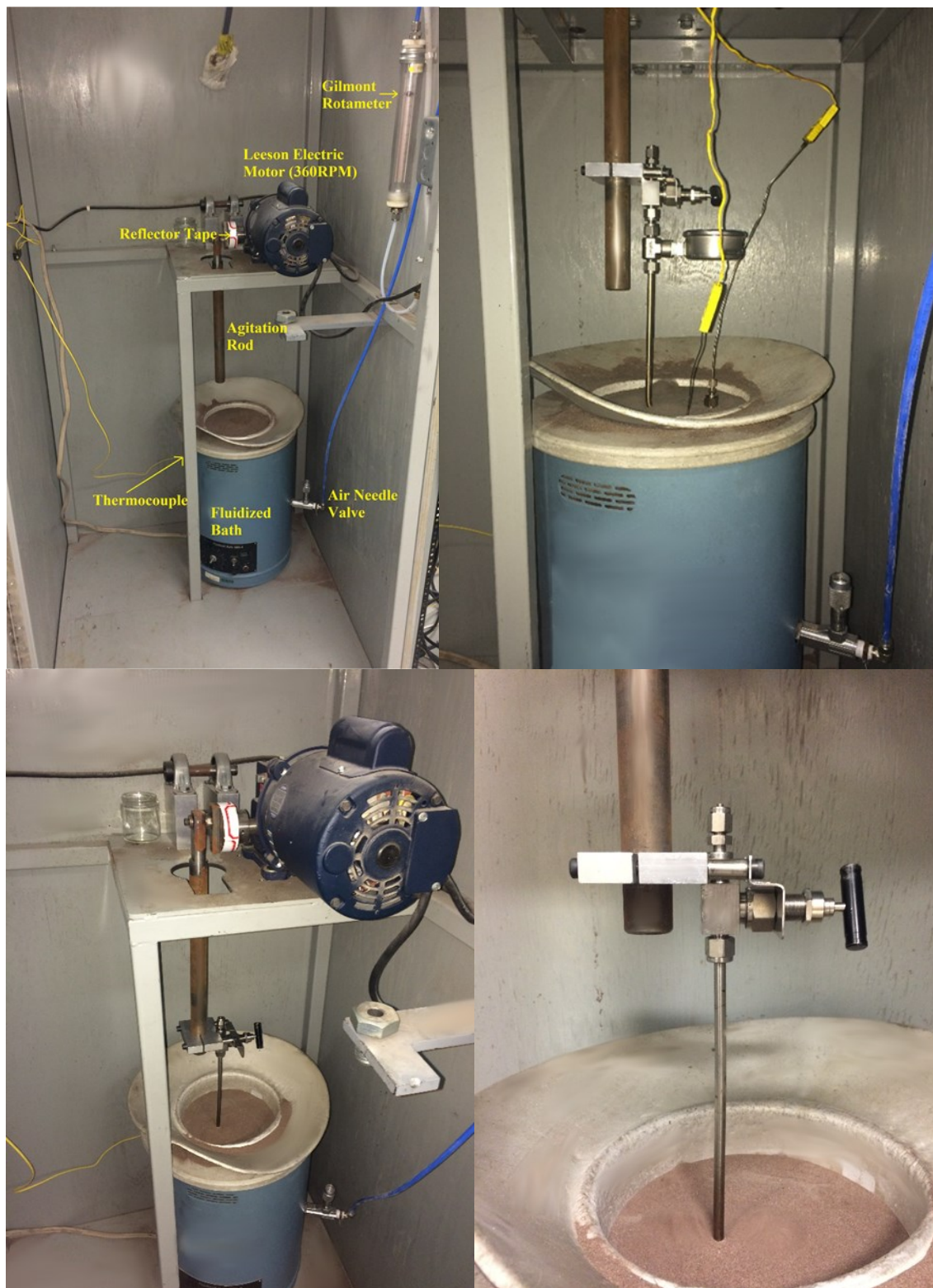
Figure 3.7. Images of the second fluidized bath setup and attached modified batch microreactor designs.
