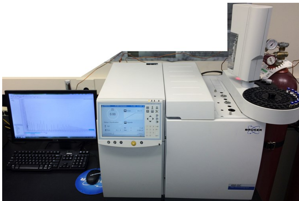
Figure 3.21. Bruker 450-GC used for boiling point distribution measurement.
