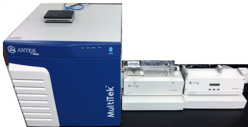
Figure 3.17. MultiTek™ analyzer used for sulfur and nitrogen analysis.
