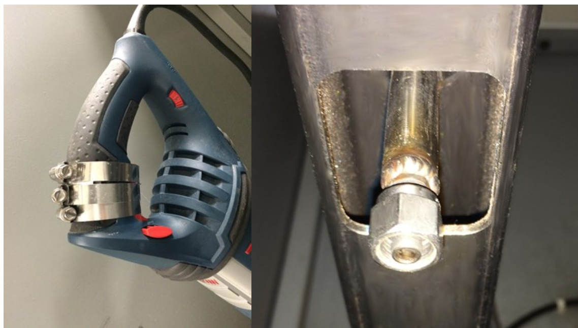
Figure 3.6. BOSCH agitator RPM controller and custom Swagelok® attachment fitting.
