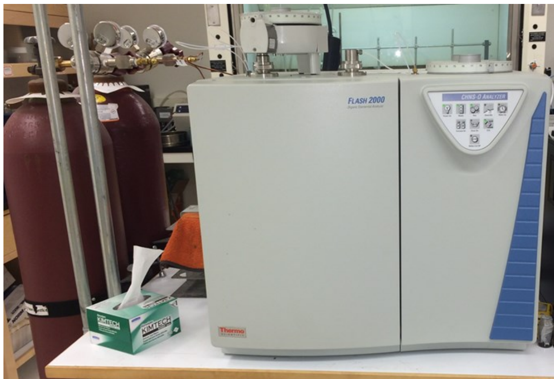
Figure 3.16. Flash 2000 organic elemental analyzer used for carbon and hydrogen analysis.
