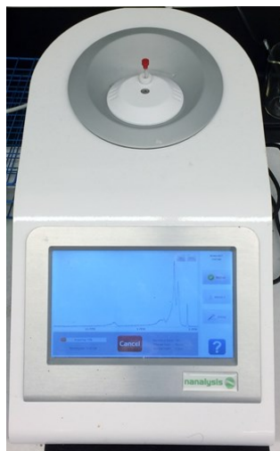
Figure 3.23. Nanalysis 60MHz benchtop nuclear magnetic spectrometer.
