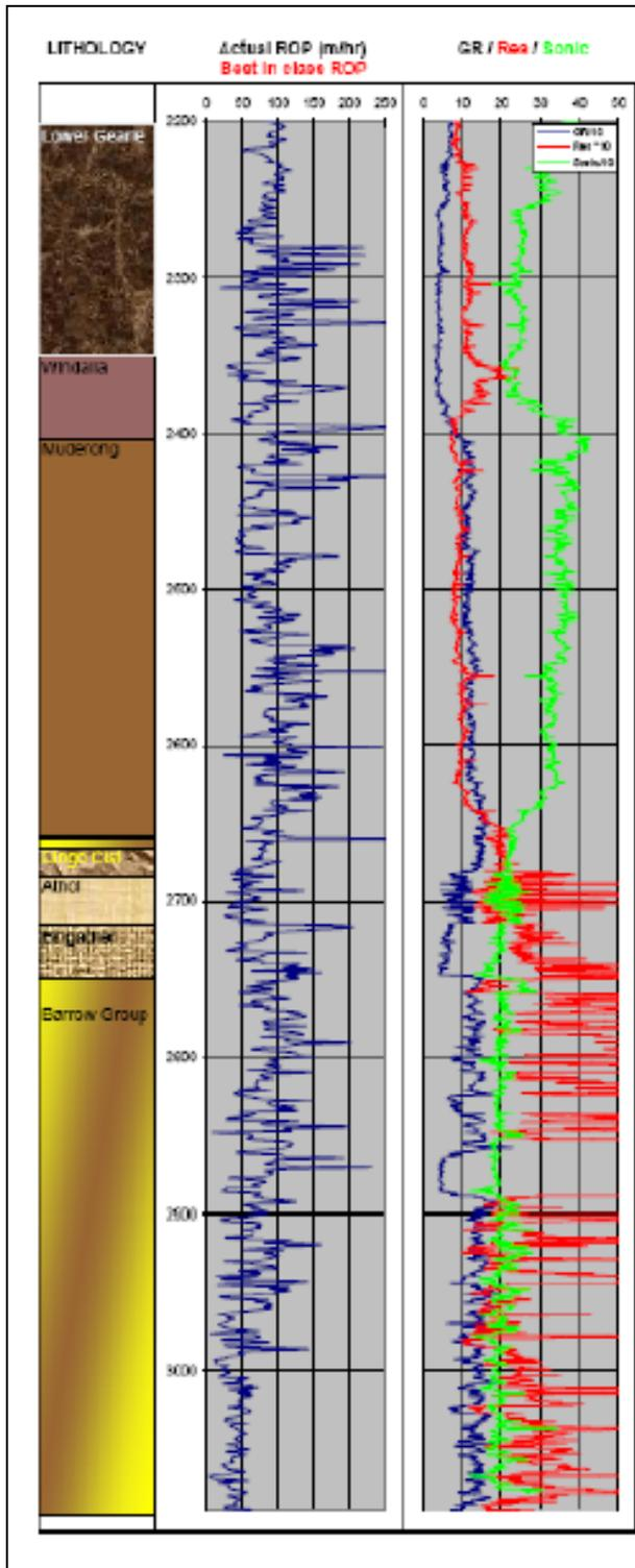
Figure 4-71: Lithology, Rate of penetration (ROP) and Gamma Ray log from left to right (part 2, modified from End of Well Report of Chandon-1).
