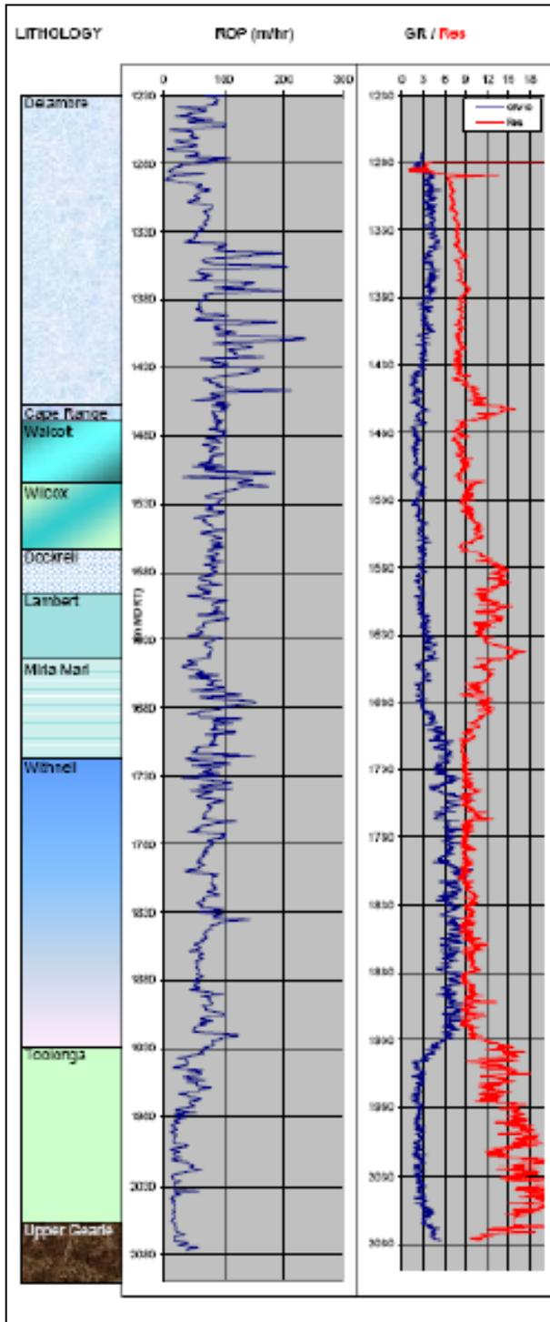
Figure 4-70: Geological sequence, Rate of penetration (ROP) and Gamma Ray log from left to right (modified from End of Well Report of Chandon-1).
