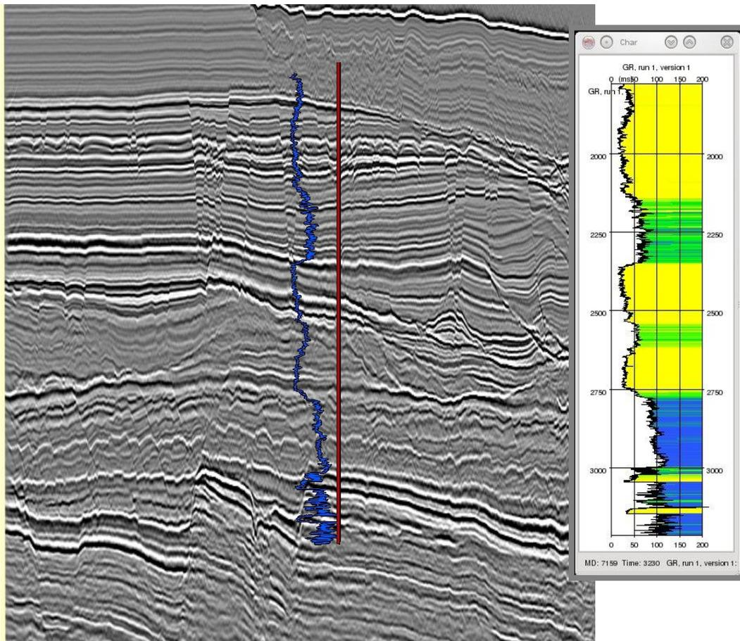
Figure 4-72: Wire-line well log of Chandon-1 in time domain: superimpose on cross-line 3930 (left) and show total depth of 3230 TWT (right). In the right picture, response from gamma ray log shows low radioactive rocks in yellow and high radioactive rocks in blue. The low radioactive rocks are potentially reservoirs such as sandstone and limestone. The high radioactive rocks are larger in clay content.
