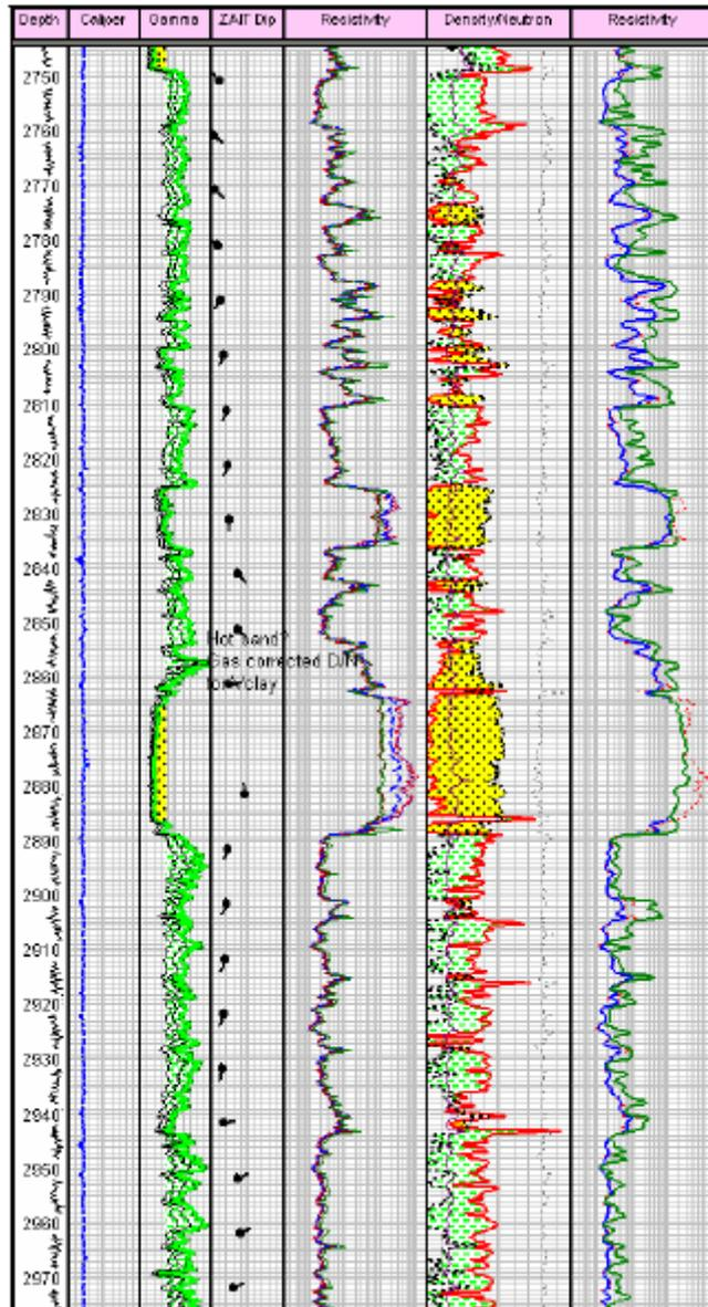
Figure 3-7: Wireline log of Chandon-1 and its different property measurement
