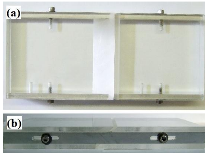
Figure 4.2: The rectangular phantom with a 45-degree dip fracture in the middle: (a) top view and (b) side view.
