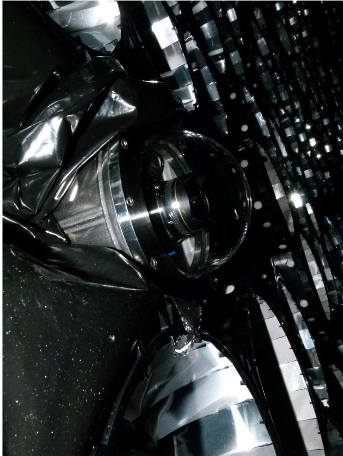
(a) Camera 1 installed amongst the SNO+ PMTs. The black plastic visible creates a boundary between the water within the PSUP, and the water without.
