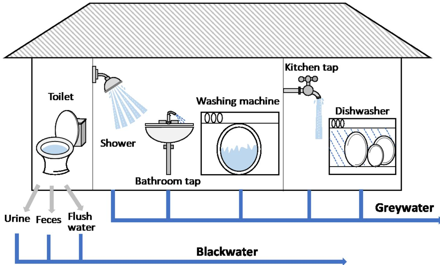
Fig. 1. Source separation of blackwater from domestic wastewater.
