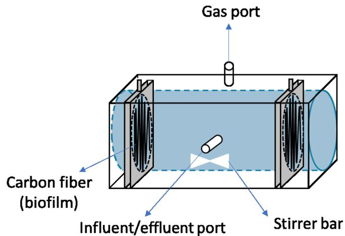
**Fig. 3.** Configuration of carbon fiber amended anaerobic biofilm reactor.
