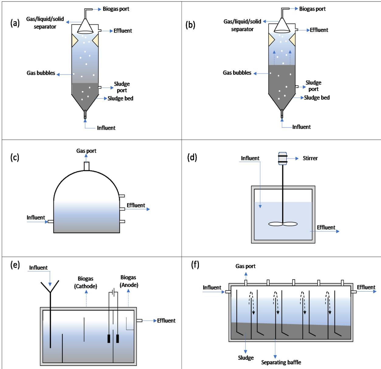
**Fig. 2.** Schematic diagrams of different anaerobic bioreactor systems studied for anaerobic blackwater treatment: (a) UASB; (b) UASB-ST; (c) AC; (d) CSTR; (e) MEC-ST; (f) ABR.
