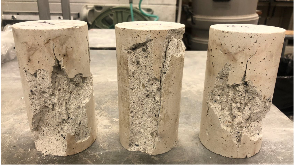
Figure A.1 Fracture types of some representative N-A-S-H geopolymer mortars collected from compression test in Chapter 3.
