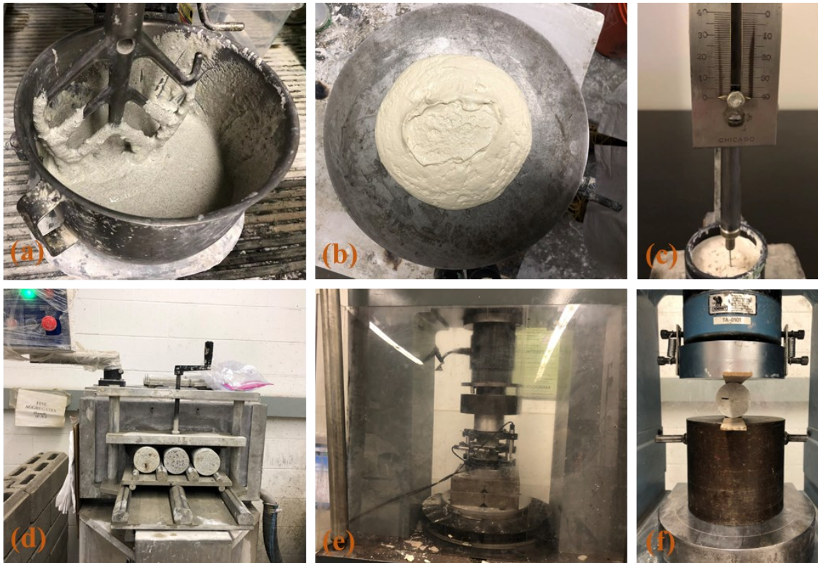
Figure 3.2 View of employed machines and apparatus for measuring fresh and hardened properties of N-A-S-H geopolymers: (a) mixer, (b) flow table, (c) Vicat needle apparatus, (d) grinder, compression machine for (e) modulus and (f) compressive alongside splitting tensile strength.
