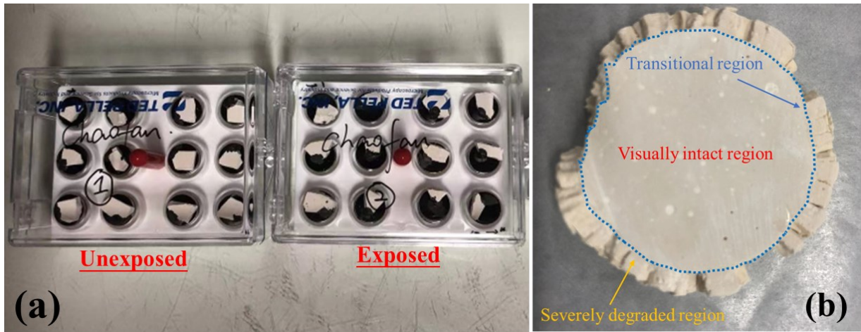
Figure 5.24 (a) Paste species for SEM test and (b) the scanned area for exposed specimens.
