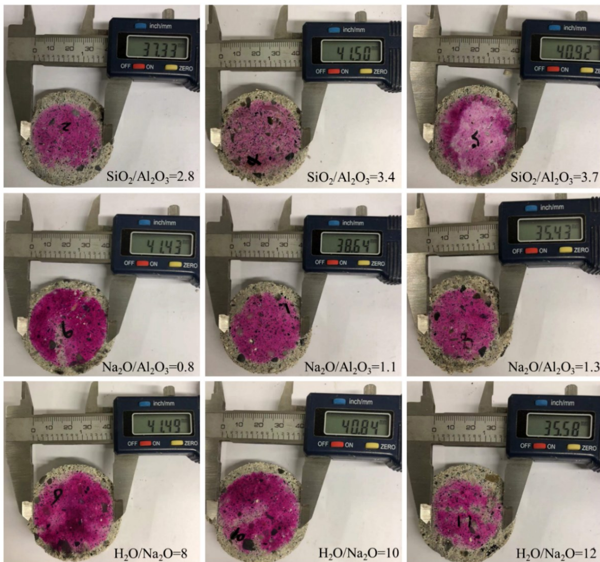
Figure 5.5 Representative images of visual inspection upon geopolymer mortars after 12 weeks of sulphuric acid attack.
