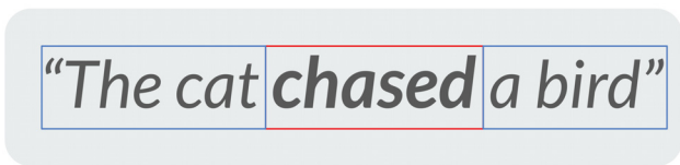
Figure 2.1: A word (red) and its context (blue) with a window size of 2
