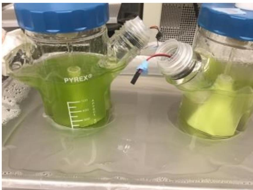
Figure 3.1. Experimental set-up for the scale-up study of LIPUS effect on *Chlorella*'s biomass accumulation during mixotrophic growth in spinner-flask bioreactors, where left is LIPUS stimulated sample, and right is control.
