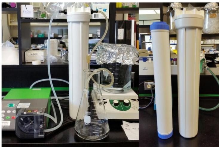
Figure 5.10. A large scale-up filtration set up, using a commercial filtration cartridge, but filled with AgNPs-coated AC and then put into a housing unit.
