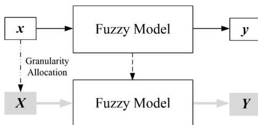
Figure 5.1. The concept of granular input space in fuzzy model systems
