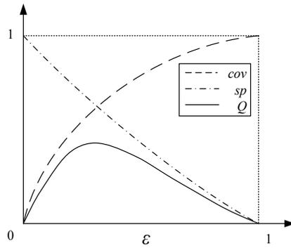
Figure 2.2. Example relationship between coverage, specificity,  $V$  and the allocation of information granularity  $\varepsilon$ .
